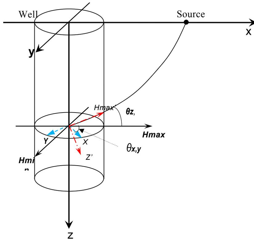
FIG A. 2 The coordinate system of x, y, and z components at the local receiver depth along with the coordinate axis that will be used after rotation (after Hinds et al., 1996).
