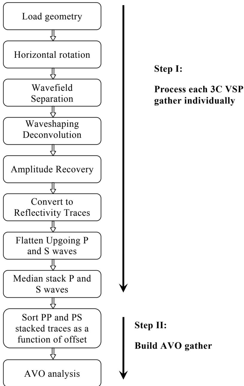
FIG 4. The walkaway VSP processing workflow for AVO analysis (modified after Coulombe et al., 1996). Each offset was processed individually to get a reflectivity trace from each shot, and then all shots were combined to form an offset-dependent gather for AVO analysis.
