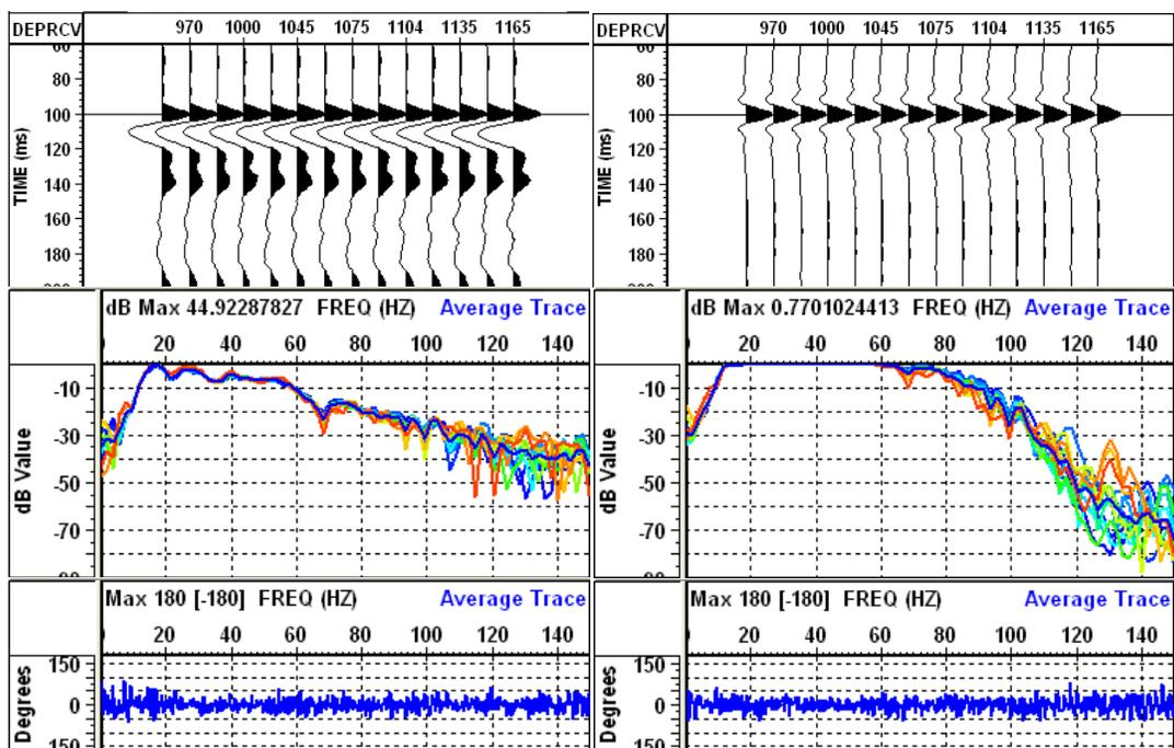
FIG 7. Downgoing P waves before (top left) and after (top right) deterministic deconvolution, as well as the corresponding amplitude spectra (the average spectrum is in blue) and average phase spectra (shot offset 558 m).
