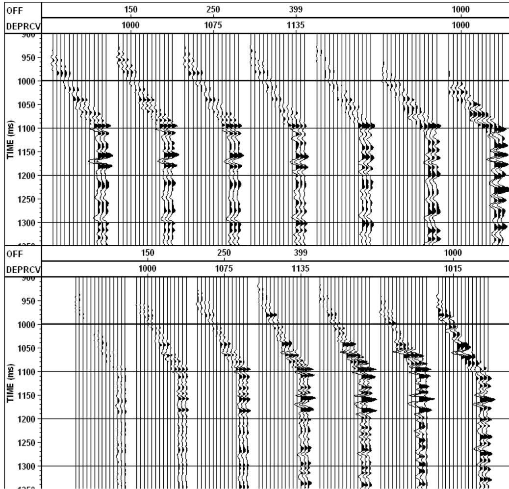
FIG 14. A 50 ms corridor mute to depth 1115m of upgoing P and upgoing SV waves.
