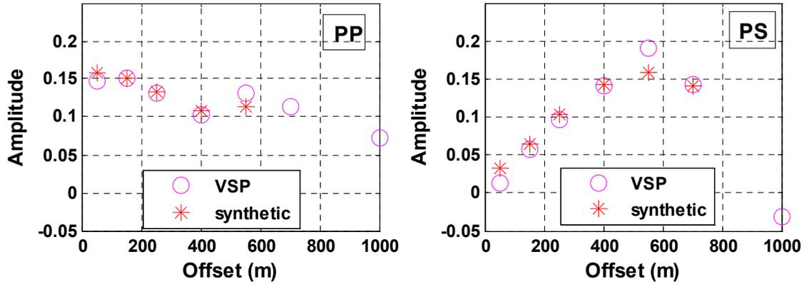
FIG 20. Comparison between the amplitude at the base of the channel sand from walkaway VSP and synthetic seismograms (generated by Syngam) for PP and PS data. The amplitude of synthetic data were scaled to the average amplitude level of VSP data.
