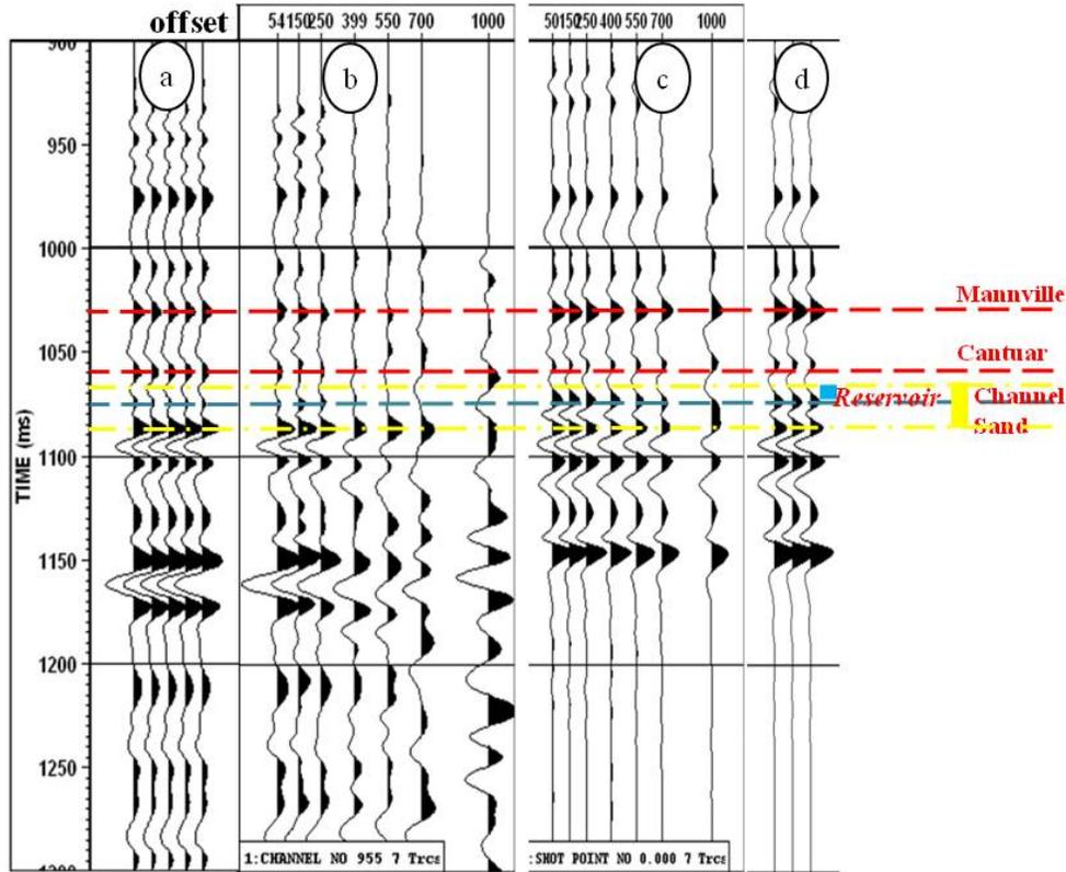
FIG 18. Comparison of PP offset gathers from walkaway VSP processing and PP synthetic seismogram from sonic and density logs. a: upgoing P wave corridor stack of the zero-offset (54 m) VSP (repeated five times); b: PP offset gather from walkaway VSP; c: PP synthetic offset gather; d: stacked traces of the PP synthetic seismogram (repeated three times).
