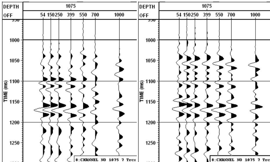
FIG 11. NMO and static correction (by flattening the 1096 ms event) applied to an upgoing P and SV offset-dependent reflectivity gather at a receiver depth of 1075 m.
