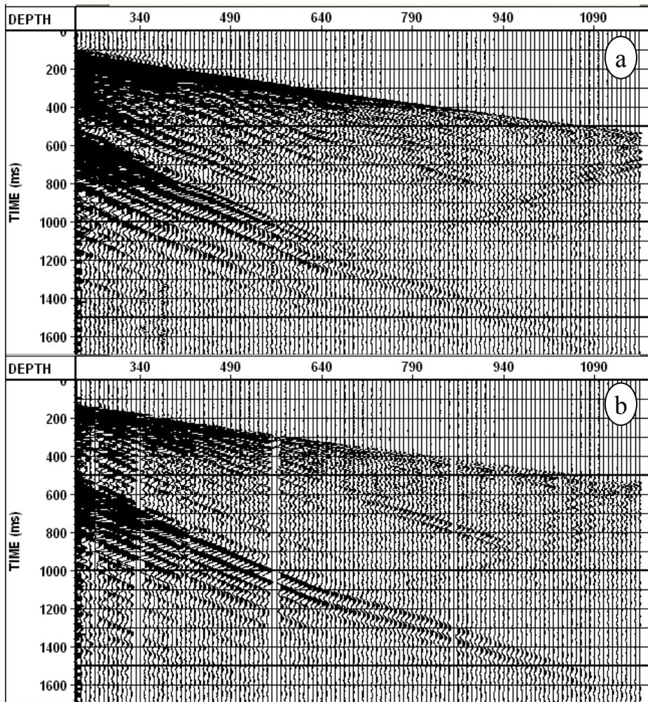
FIG A. 3 Hmax (horizontal radial, a) and Hmin (horizontal transverse, b) of zero-offset VSP (offset 54m, vertical vibrator). Hmax and Hmin are from horizontal rotation of X and Y components.
