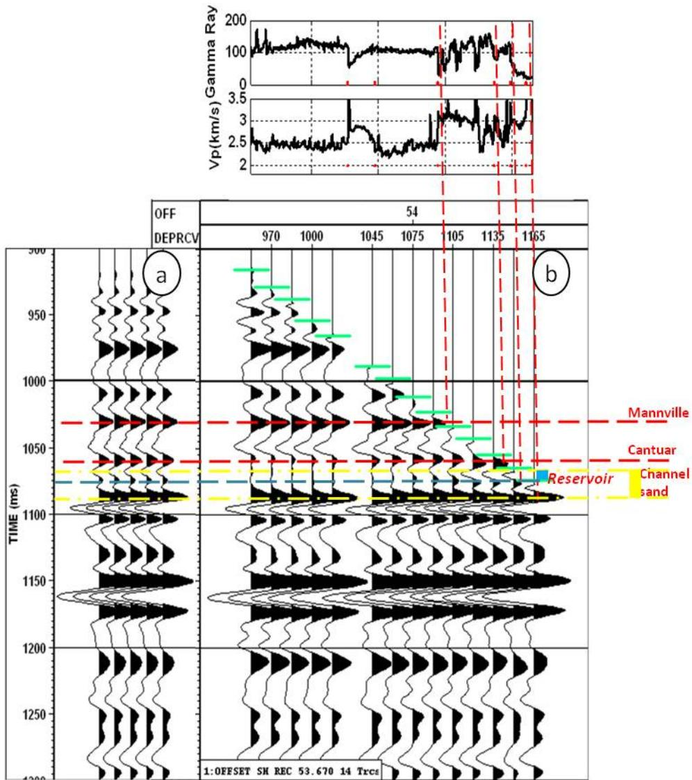
FIG 16. Correlation between well logs and zero-offset VSP within walkaway VSP receiver depth range. a: upgoing P wave corridor stack; b: upgoing P wave in two-way P travelttime (applied NMO and first-arrival time flattening).
