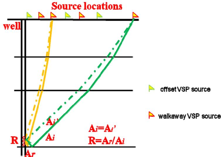
FIG 1. Schematic diagram of the advantage of walkaway VSP geometry for AVO processing. Since the receivers are located very close to the reflectors, the incidence wave amplitude  $A_i$  approximately equal to the downgoing wave amplitude  $A_i'$ . Thus the reflectivity  $R$  can be calculated by dividing the upgoing wave amplitude  $A_r$  by downgoing wave amplitude  $A_i$ . Shots at varied locations give different incidence angles, therefore AVO gather can be built.
