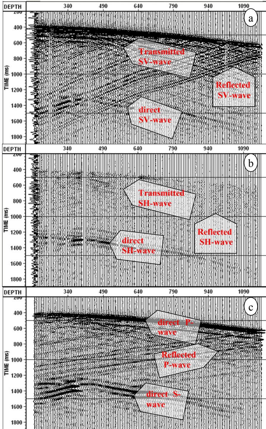
FIG A. 4 Hmax (horizontal radial, a), Hmin (horizontal transverse, b), and Z (c) components of far-offset VSP (offset 699 m). Hmax and Hmin are from horizontal rotation of X and Y components.
