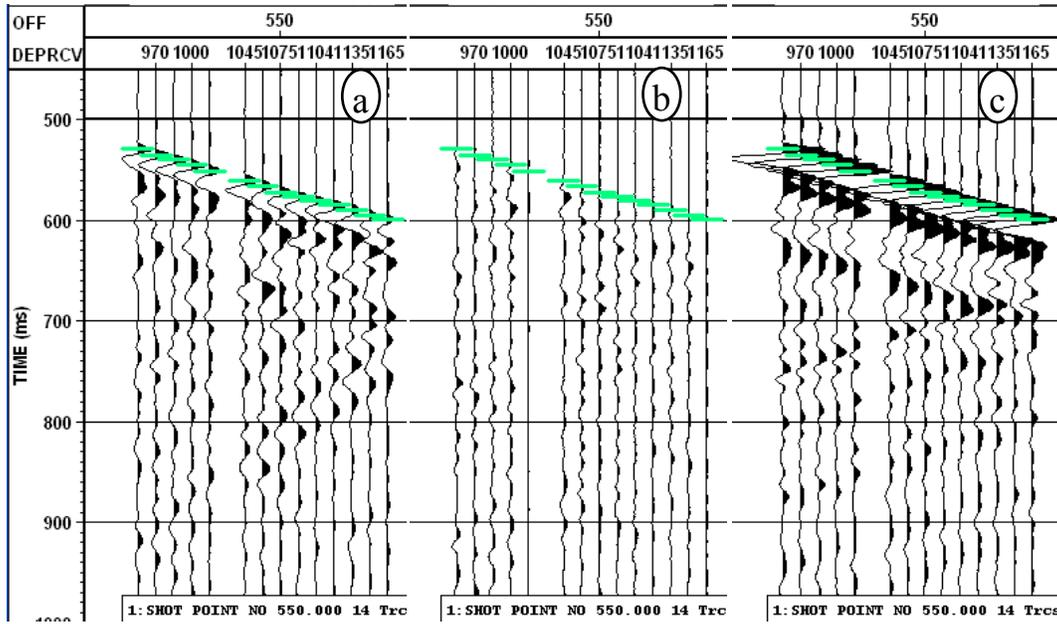
FIG 5. Hmax (a, horizontal radial), Hmin (b, horizontal transverse) after a horizontal rotation of X and Y components, and Z component data (c) of the offset 558 m shot (AGC applied, the green line is the first break picks). The waves received in transverse direction (Hmin) are much weaker than those in the radial direction (Hmax).
