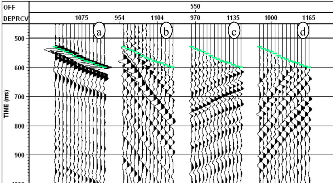
FIG 6. Downgoing P waves (a), downgoing SV waves (b), upgoing P waves (c), and upgoing SV waves (d) separated from Hmax and Z data of the offset 558 m shot (AGC applied, the green line indicates the first arrival picks).
