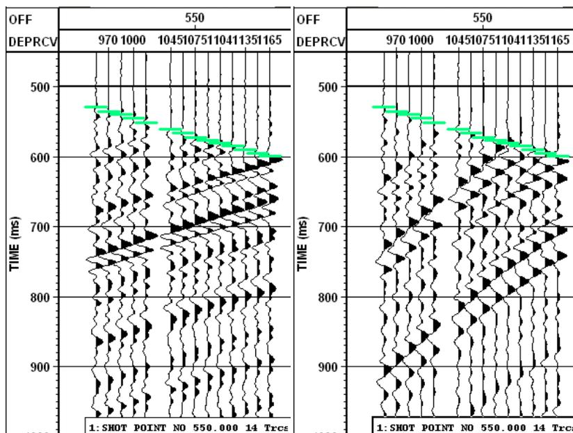
FIG 8. Upgoing P and SV waves after a deterministic deconvolution with operator derived from downgoing P waves (shot offset 558 m, the green line indicates first arrival picks).
