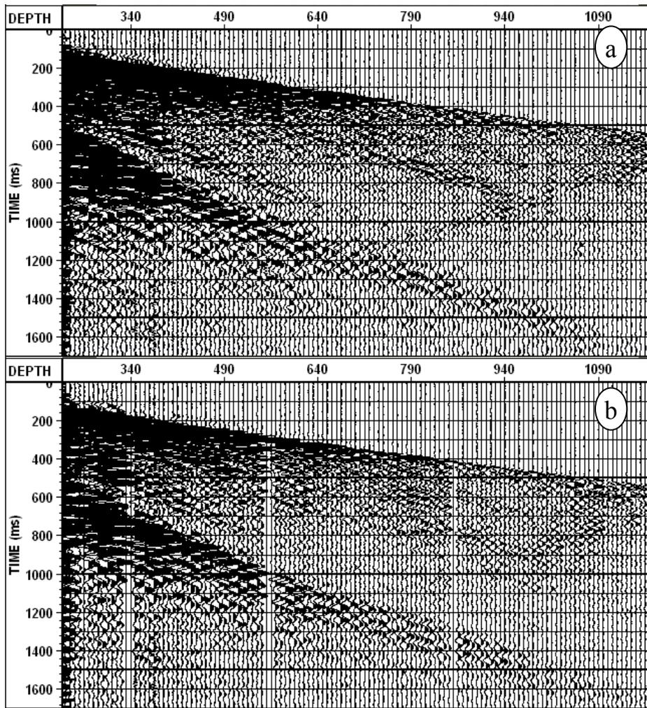
FIG A.1 (a) and Y components (b) of vertical vibrator zero-offset VSP data (source offset 54 m). It shows that the horizontal sensors are oriented in randomly azimuth. Very little coherent signal can be seen on the raw x and y data.
