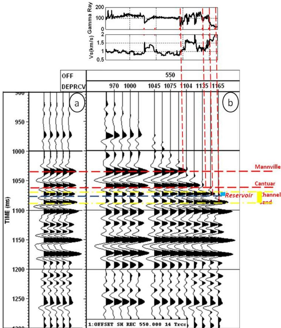
FIG 17. Correlation between well logs and source offset 558 m VSP within walkaway VSP receiver depth range. a: upgoing PS wave corridor stack; b: upgoing PS wave in two-way P travelttime (applied NMO and first-arrival time flattening).
