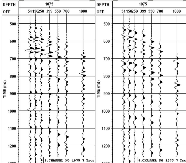
FIG 10. Upgoing P and SV offset-dependent reflectivity gather at a receiver depth of 1075 m.
