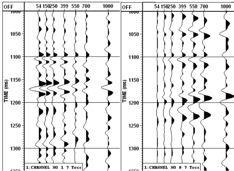
FIG 12. Offset gathers of upgoing P and upgoing SV waves from the common shot stack of 1096 ms event flattened gathers (no NMO correction). Note that only the 1096 ms reflection was exactly flattened, the other reflections were all dipping toward 1096 ms event.
