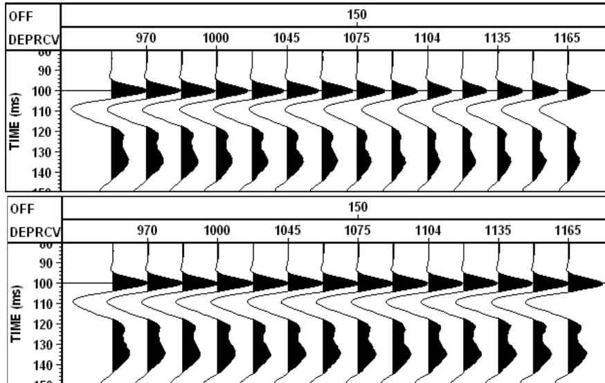
FIG 9. Downgoing P waves before and after mean scaling (flattened to 100 ms, shot offset 558 m). Note amplitude decay of direct P waves with increasing receiver depth before scaling.
