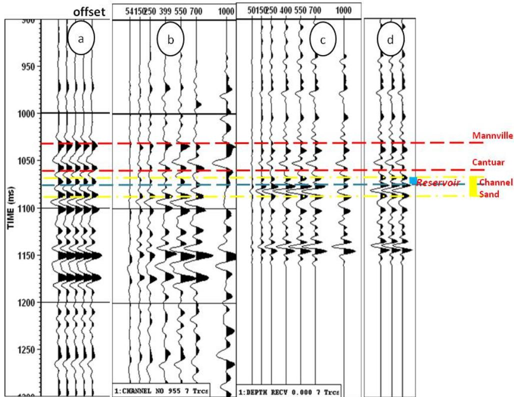
FIG 19. Comparison of the PS offset gather from walkaway VSP processing and PS synthetic seismograms from sonic and density logs. a: upgoing PS wave corridor stack of offset (558 m) VSP (repeated five times); b: PS offset gather from walkaway VSP; c: synthetic PS offset gather; d: stacked traces of the synthetic seismogram (repeated three times). All PS data are plotted in two-way P wave travelttime.
