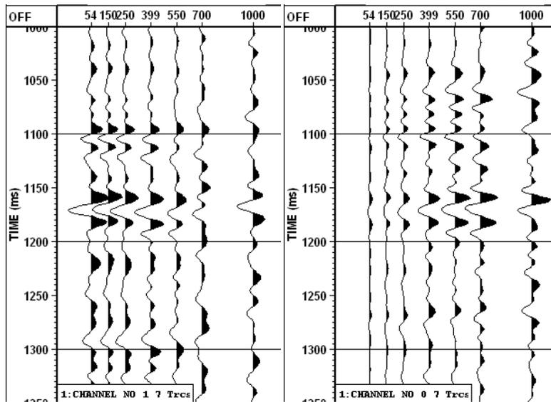
FIG 13. Offset gathers of upgoing P and upgoing SV waves from the common shot stack after NMO and static correction (by flattening the 1096 ms event). SV wavefield (P-SV) was also converted to PP reflection time.
