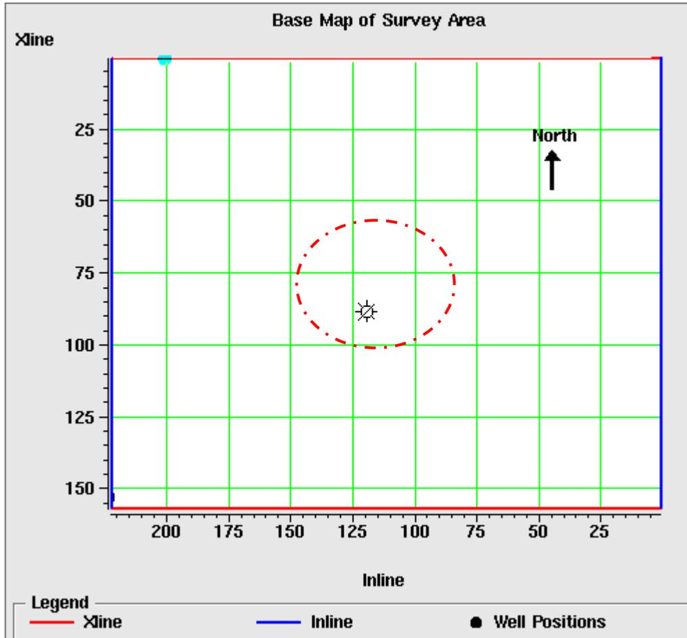
FIG 2. The time-lapse 3C-3D survey map. The red circle outlines the “trap door” area (where time delays of interpreted from seismic reflections around the mining level were caused possibly by brine inflow) interpreted from previous work (from John Boyd, personal communication, 2010).
