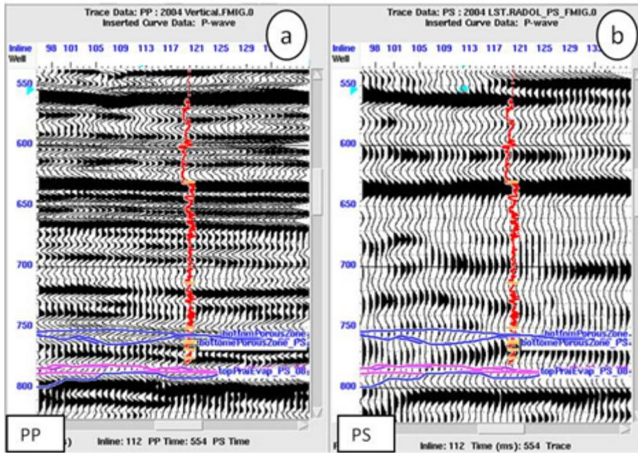
FIG 6. Registration of the PP data and PS data of the 2004 survey, both data are in PP time. The picked horizon at about 750ms is the base of the porous zone, and the horizon at about 800ms is approximated the top of Prairie Evaporite Formation. The horizontal bars on the well log curve are the geological markers.
