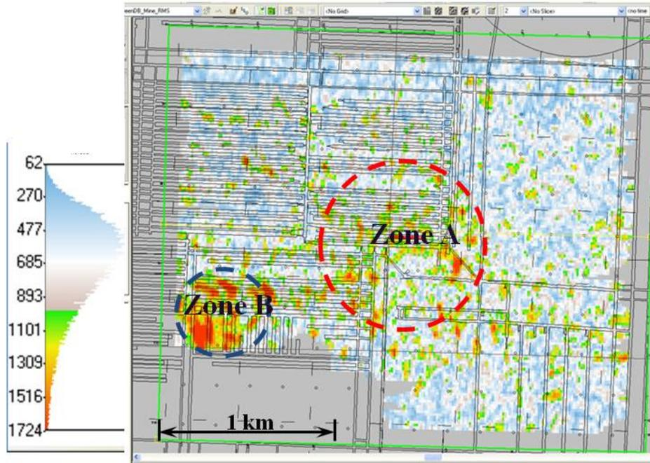
FIG 11. RMS amplitude difference of PS data from the Dawson Bay Formation to mine level between 2004 and 2008 survey.
