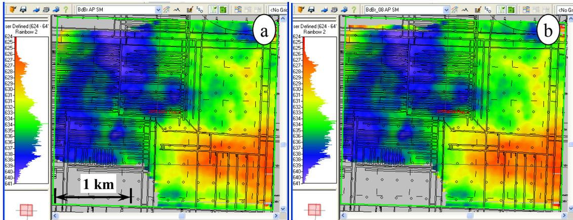
FIG 14. Time structure of the top of the Birdbear Formation on the PP data, a: 2004 survey; b: 2008 survey. There is almost no time shift between the two surveys.
