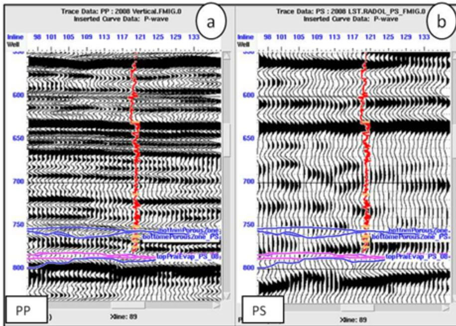
FIG 7. Registration of PP data (a) and PS data (b) of the 2008 survey, both data are in PP time. The picked horizon at about 750ms is the base of the porous zone, and the horizon at about 800ms is approximately the top of Prairie Evaporite Formation. The horizontal bars on the well log curve are the geological markers.
