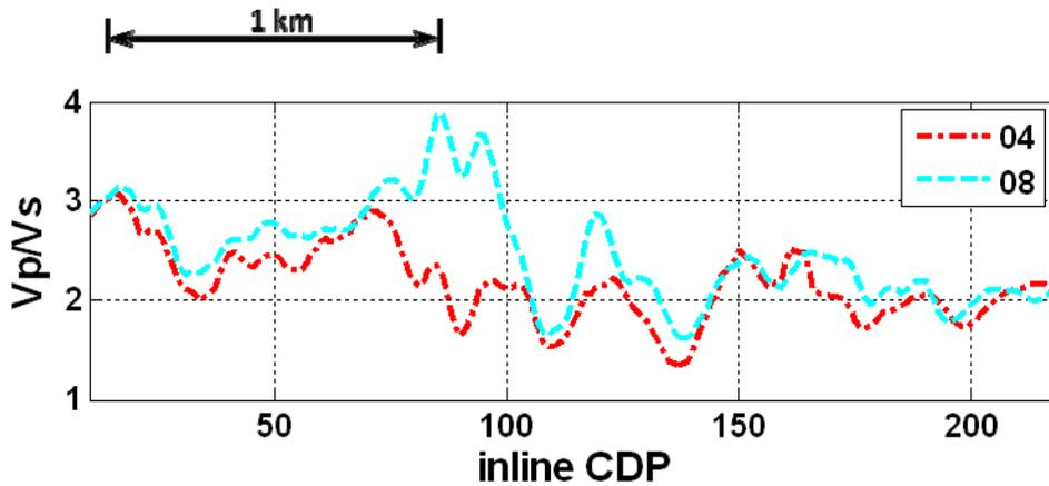
FIG 21. Average Vp/Vs values of west-east line 89 between the bottom of the Porous zone and the top of Prairie Evaporite Formation. The red line denotes the values from the 2004 survey, the blue line shows the values of the 2008 survey.
