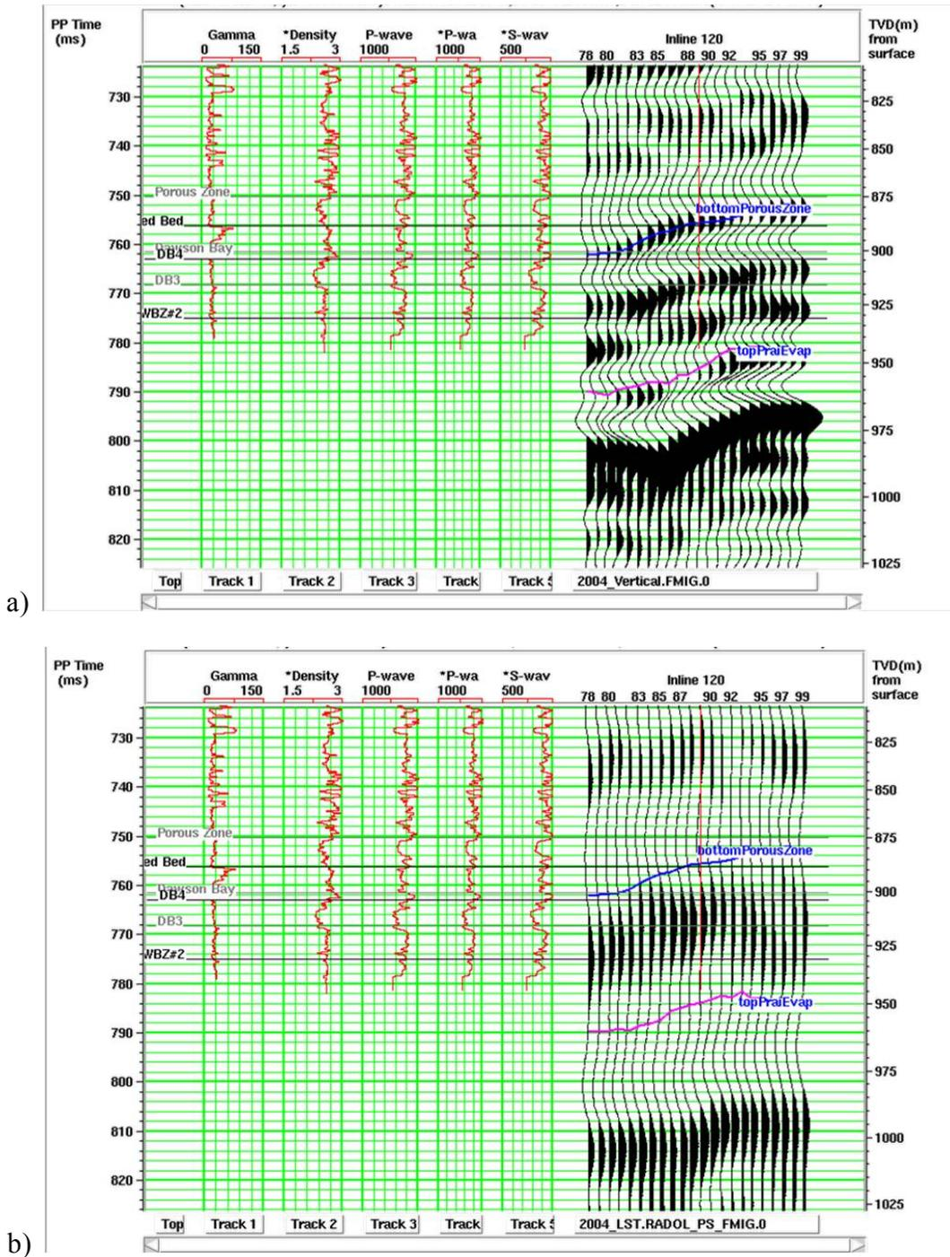
FIG 8. The base of the Porous Zone and the base of the Dawson Bay Formation picks and the correlation with well logs. On the vertical component, the base of the Porous Zone is a peak, the base of the Dawson Bay Formation corresponds to a zero-crossing point on seismic traces. On the radial component, there are no accurate picks for the two geological markers due to low resolution. Approximately they correspond to two zero-crossing points.
