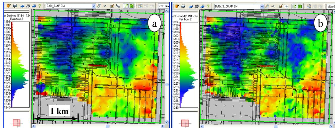
FIG 15. Time structure of the top of the Birdbear Formation on the PS data, a: 2004 survey; b: 2008 survey. The time shift between the two surveys is fairly small. A little delay was found on 2008 survey.
