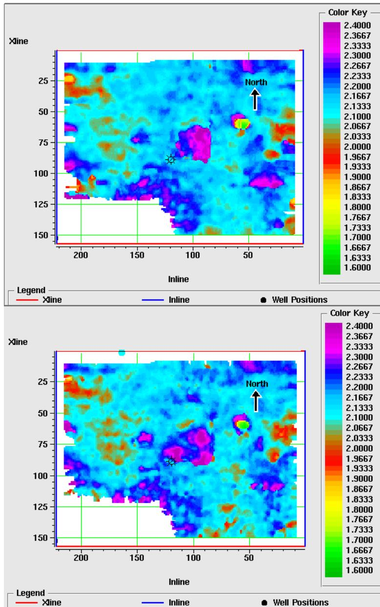
FIG 20. Interval Vp/Vs map from the Birdbear Formation to the Shell Lake anhydrite. a: 2004 survey; b: 2008 survey.
