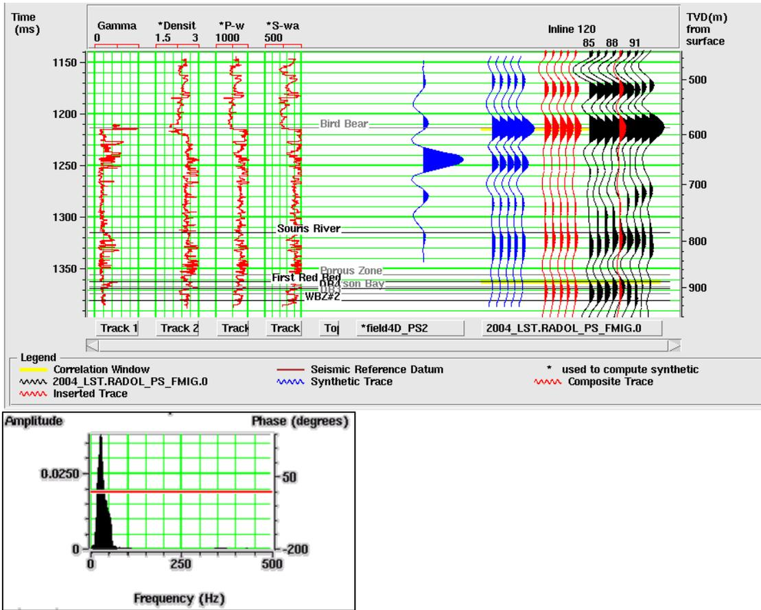
FIG 5. Correlation between the synthetic PS seismogram of well GROUT 59-1 and migrated PS data of 2004 survey. The synthetic seismogram is displayed in blue and repeated for 5 times, the seismic traces adjacent to the well are displayed in black. The corresponding frequency spectrum is shown at the bottom.
