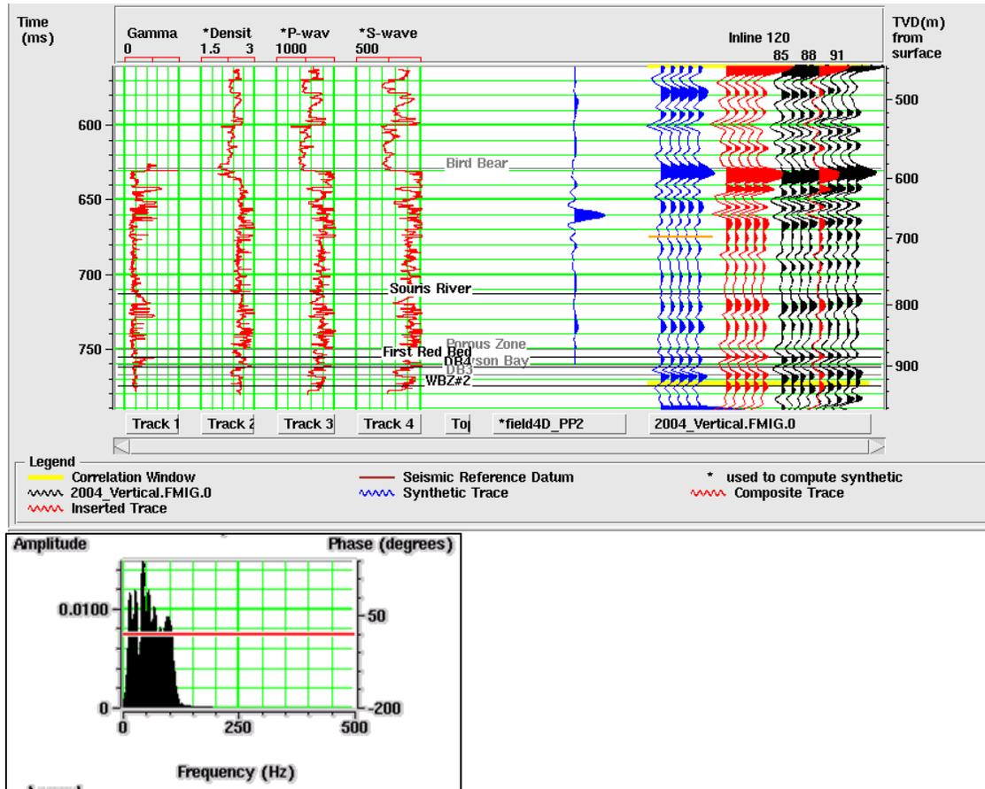
FIG 4. Correlation between the synthetic PP seismogram of well GROUT 59-1 and migrated PP data of 2004 survey. The synthetic seismogram is displayed in blue and repeated for 5 times, the seismic traces adjacent to the well are displayed in black. The corresponding frequency spectrum is shown at the bottom.
