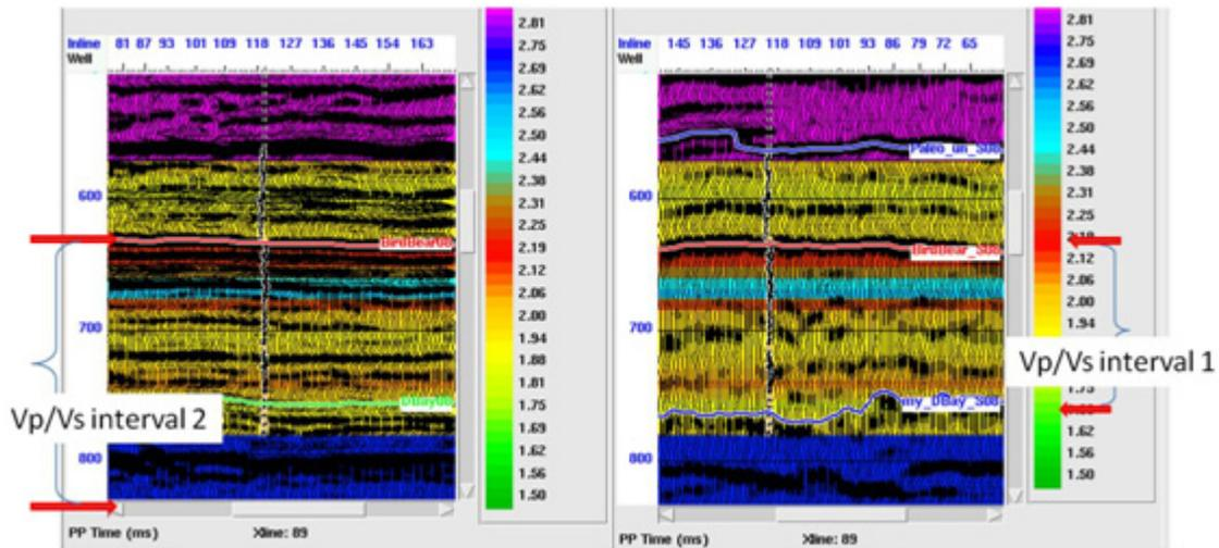
FIG 18. The arrow marks the intervals used for interval Vp/Vs calculation. Interval 1 is from the Birdbear Formation to the Dawson Bay Formation; interval 2 is from the Birdbear Formation to (approximately) the Shell Lake anhydrite below the Dawson Bay Formation (Vp/Vs extrapolated from well values superimposed on the seismic sections).
