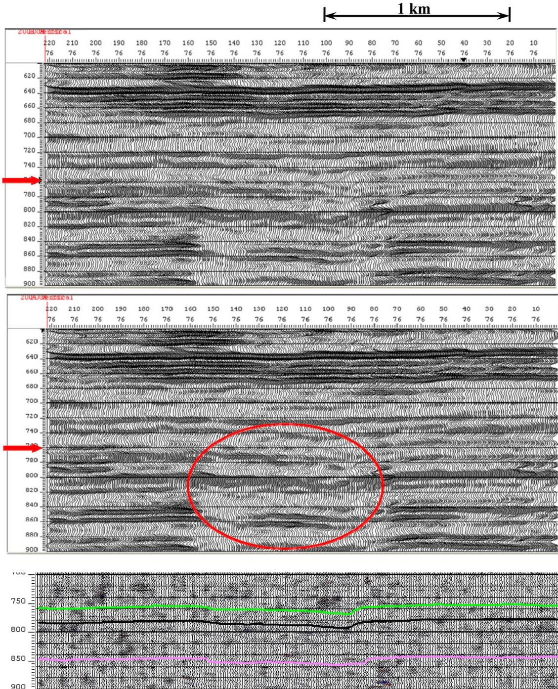
FIG 9. PP data of a west-east line. Top: 2004 survey; middle: 2008 survey; bottom: difference between the two data sets. The red arrows mark the location of the top of the Dawson Bay Formation. The red ellipse denotes the trap door area.
