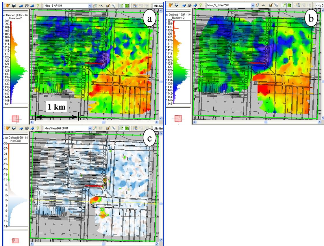
FIG 17. Time structure of the mine level on the PS data, a: 2004 survey; b: 2008 survey; c: PS travel time difference at the mine level between 2008 and 2004 survey.
