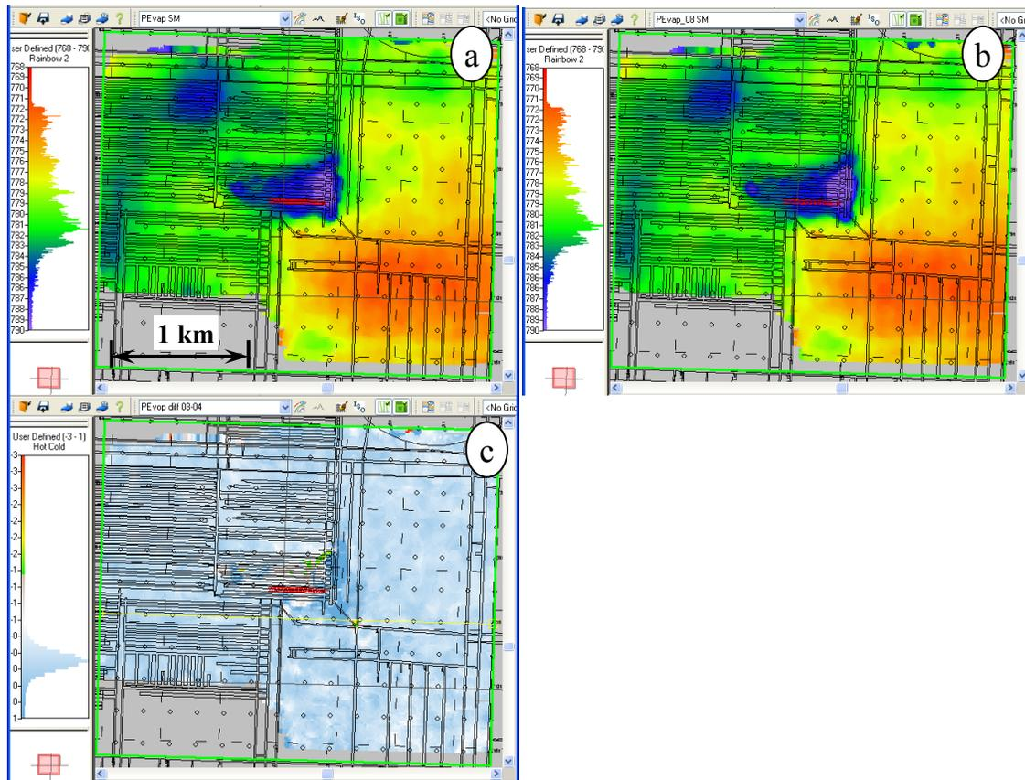
FIG 16. Time structure of the top of the Prairie Evaporite Formation on the PP data, a: 2004 survey; b: 2008 survey; c: PP travel time difference at the top of the Prairie Evaporite Formation between 2008 and 2004 survey.
