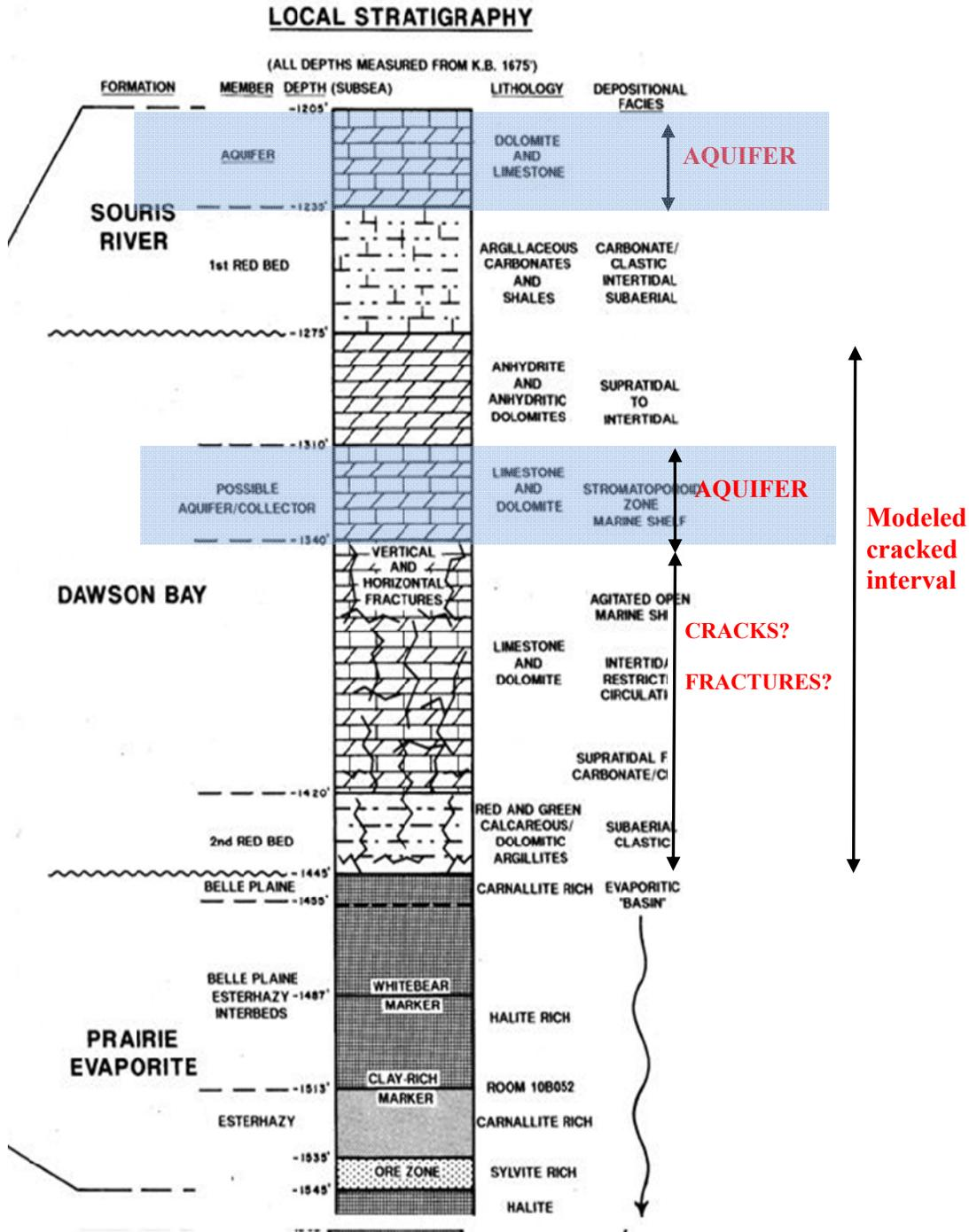
FIG 1. Local stratigraphy of Prairie Evaporite and overlying formations in the mining area. The Dawson Bay carbonates, dolomites, and shales can host fractures (from R. Edgcombe, personal communication, 2008).
