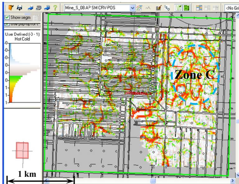
FIG 23 Positive curvature of the mine level on PS data of the 2008 survey.
