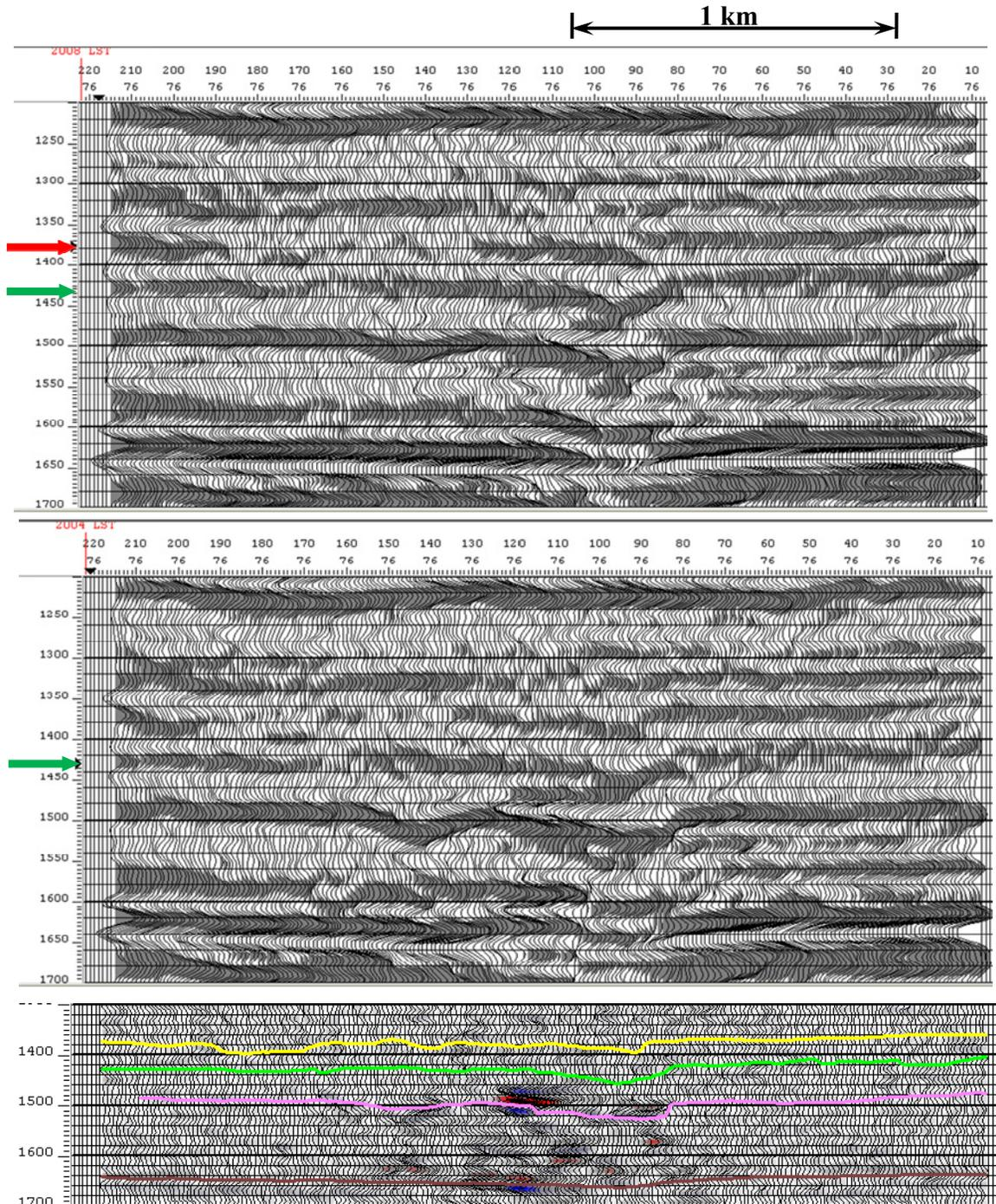
FIG 10. PS data of a west-east line. Top: 2004 survey; middle: 2008 survey; bottom: difference between the two data sets. The red arrows mark the location of the top of the Dawson Bay Formation. The green arrows are the mining zone. The trap door area is outlined by red ellipse.
