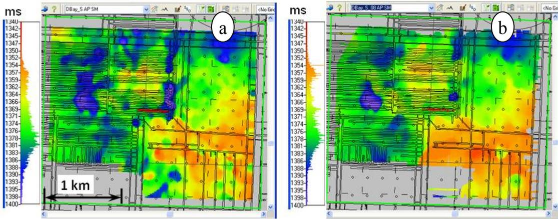
FIG 13. Time structure of the top of the Dawson Bay Formation on the PS data, a: 2004 survey; b: 2008 survey.
