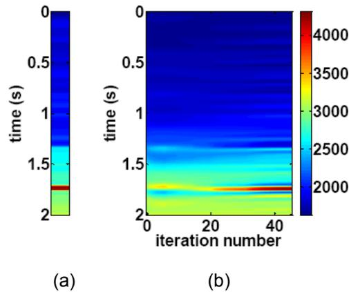
FIG. 8: FWI inversion updates at 1800m lateral position. a) The true velocity b) Velocity profiles updates vs. Iteration numbers.
