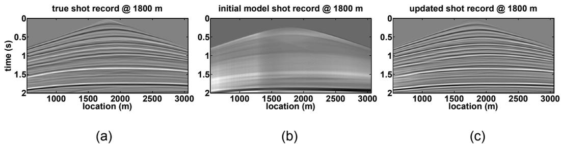
FIG. 9: FWI inversion shot prediction at 1800m lateral position (with 0.2s AGC window and minimum phase wavelet with 12 Hz dominant frequency). a) The true shot record b) the initial shot record c) the updated shot record after 45 iterations.
