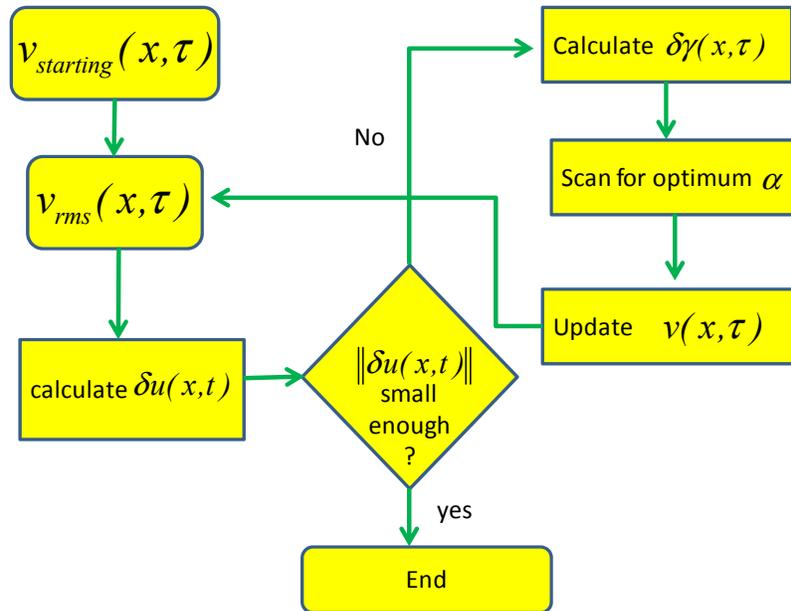
FIG. 5: Simplified algorithm for updating velocity using time migration FWI algorithm.
