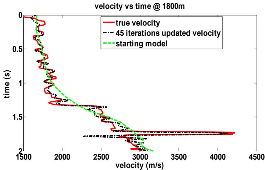
FIG. 7: Comparison between the true velocity model (solid red) the starting model (green dashed) and the FWI model (dashed dot black) using the PSTM strategy at 1800m lateral position.
