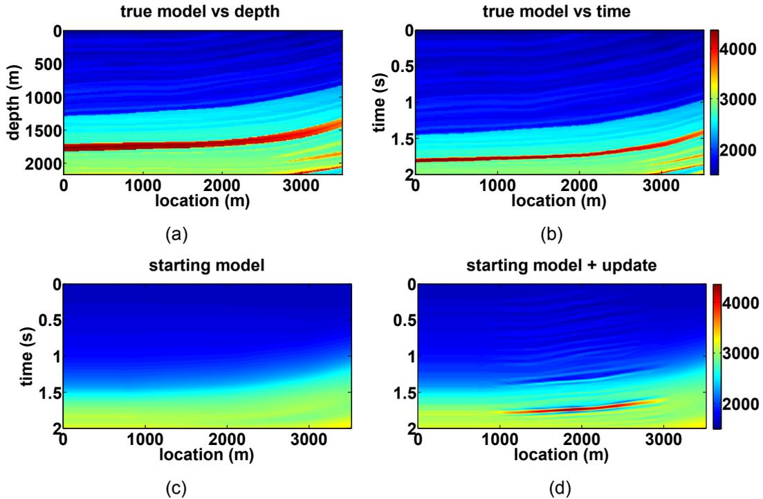
FIG. 6: FWI using PSTM for Marmousi model using 21 shots from 1250m to 2250m. a) True velocity vs depth b) True velocity vs time c) starting velocity d) The inverted velocity after 45 iterations.
