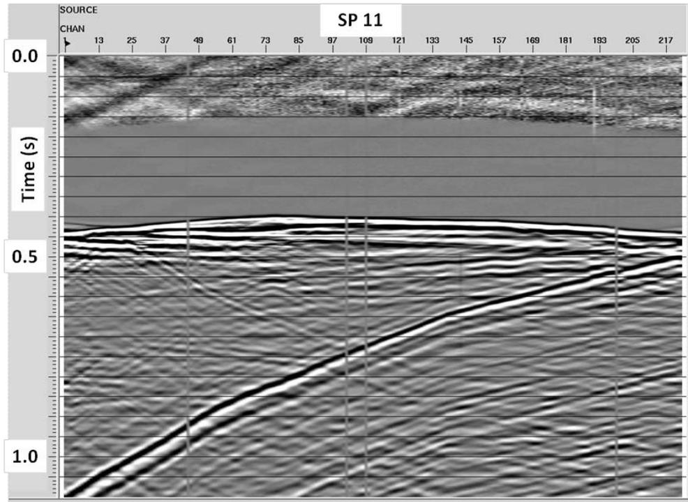
FIG. 12. Radial component of an offset VSP survey showing a high amplitude up-going PS-wave. Dynamite source.
