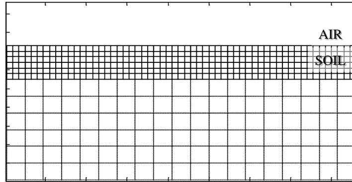
FIG 2. Spatial grid for velocity coefficient problem defined in soil layer.
