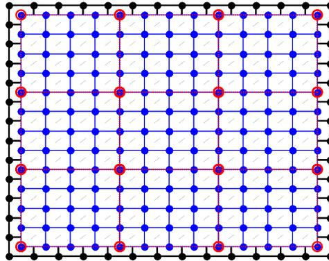
FIG 1. Regular grids used in grid scaling: Black –grid for wave propagation ( $u$  and  $\varphi$ ); Blue – fine grid for velocity field used  $c^2$  in finite-difference approximation of (1); Red – coarse grid for  $c^2$  used in gradient minimization (12)
