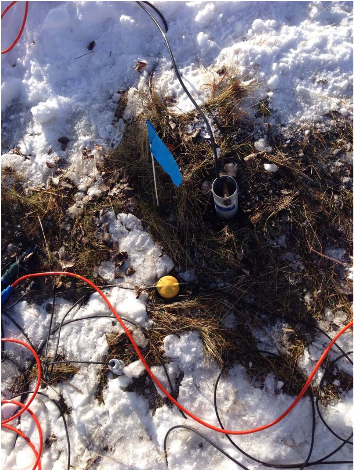
FIG. 22. The high sensitivity geophone (silver), the new Inova receiver (yellow) and a ground screw installed 3C geophone.
