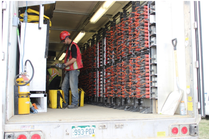
FIG. 14. The Hawk nodal system in the data harvesting/charging trailer.
