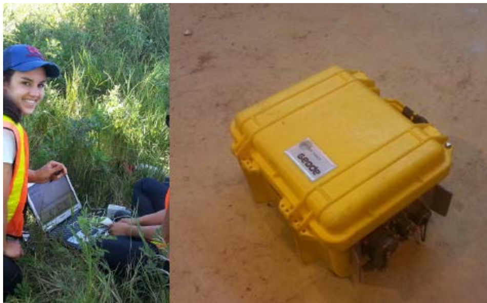
FIG. 3. The laptop recording Geode data and a sing Geode box.
