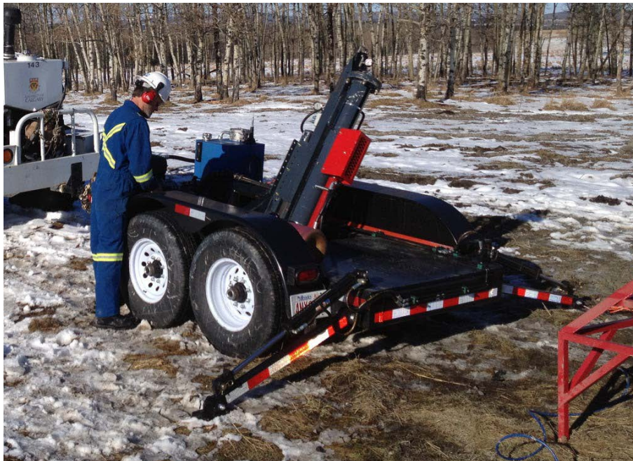
FIG. 7. The new nitrogen spring s-wave source.
