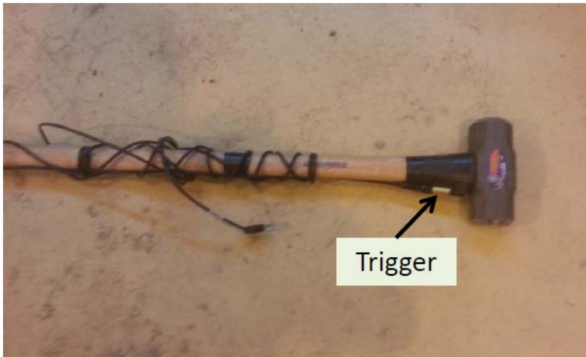
FIG. 8. The Geometrics trigger attached to a hammer source.
