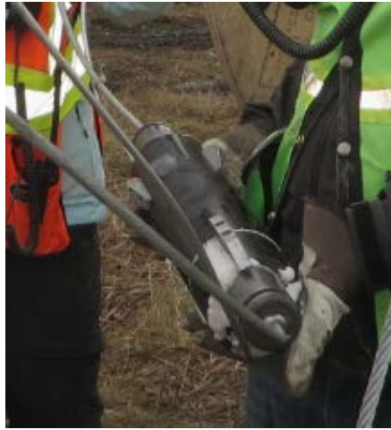
FIG. 4. The USSI fibre optic geophone inside it's clamping housing.
