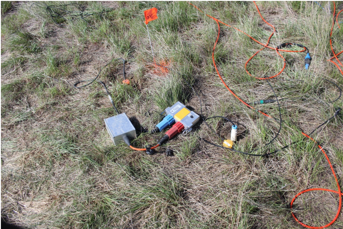
FIG. 13. The comparison of receivers, 3C analogue geophone connected to the nodal system, and an analogue geophone connected to the Aries, and a new digital sensor.
