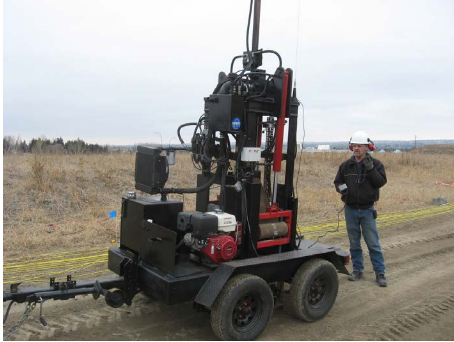
FIG. 6. The older elastic weight drop p-wave source.
