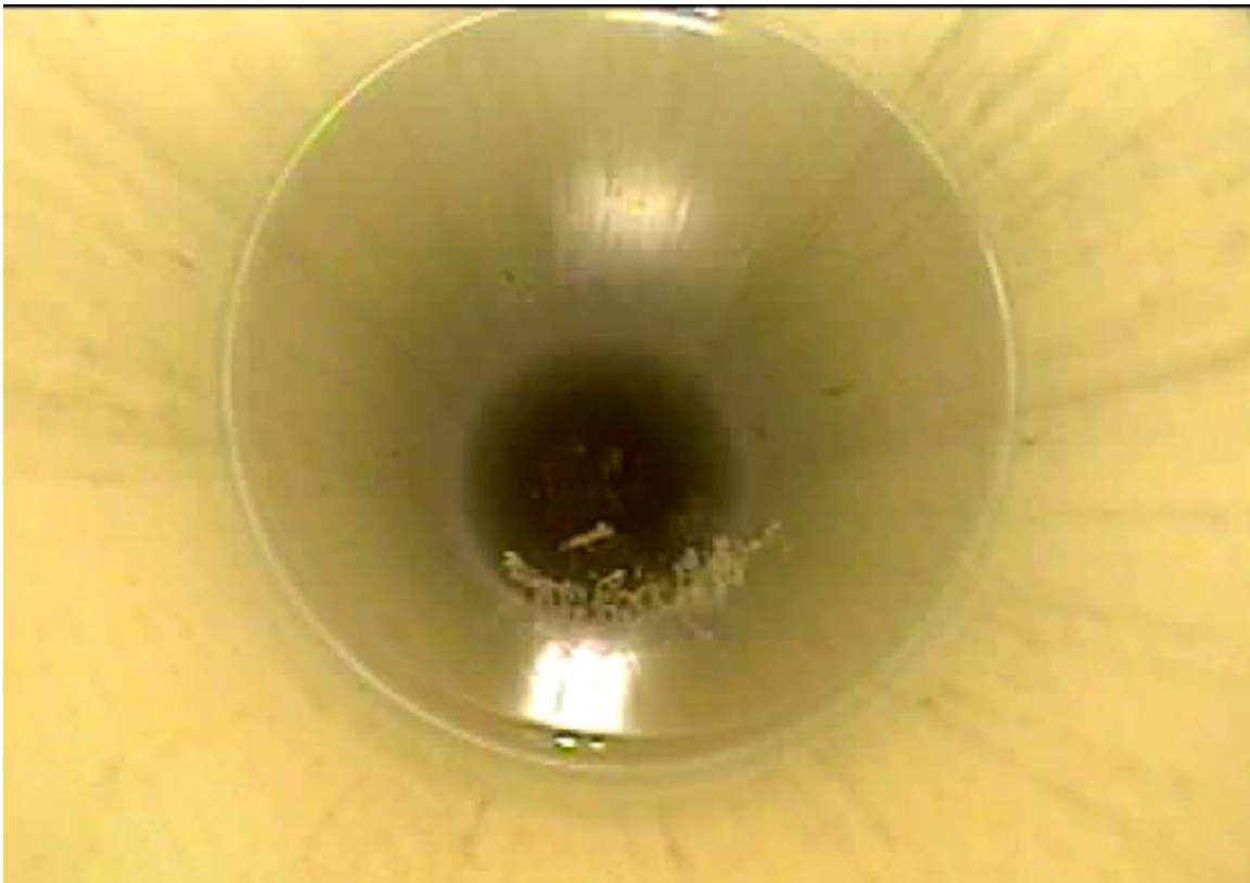
FIG. 11. The light from the down hole camera system being reflected off the water.
