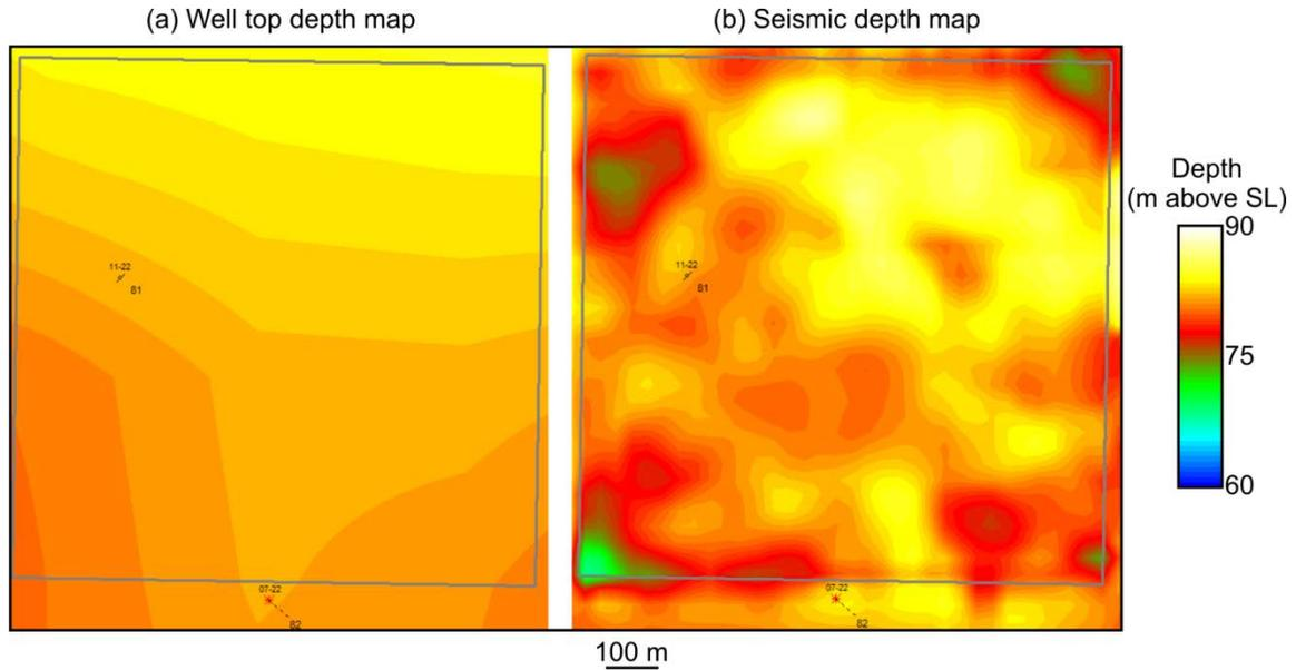
FIG. 10: Depth maps of the (a) gridded well top and (b) gridded seismic horizon from the 2014 3D seismic survey for the top second white Speckled Shale Formation over Section 22.
