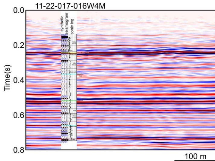
FIG. 4: Tie between synthetic seismogram for well 11-22-017-16W4M and a crossline from the 3D survey.
