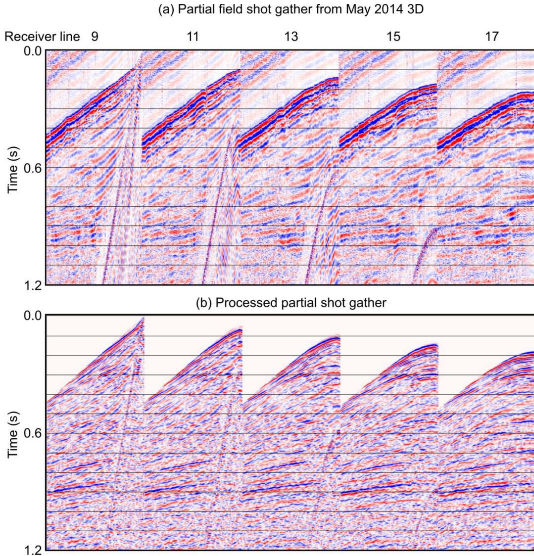
FIG 3: Field and processed partial shot gathers from the new 3D survey.
