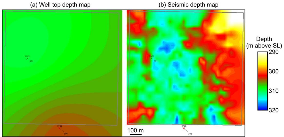
FIG. 9: Depth maps of the (a) gridded well top and (b) gridded seismic horizon from the 3D seismic survey for the top Medicine Hat Formation over Section 22.
