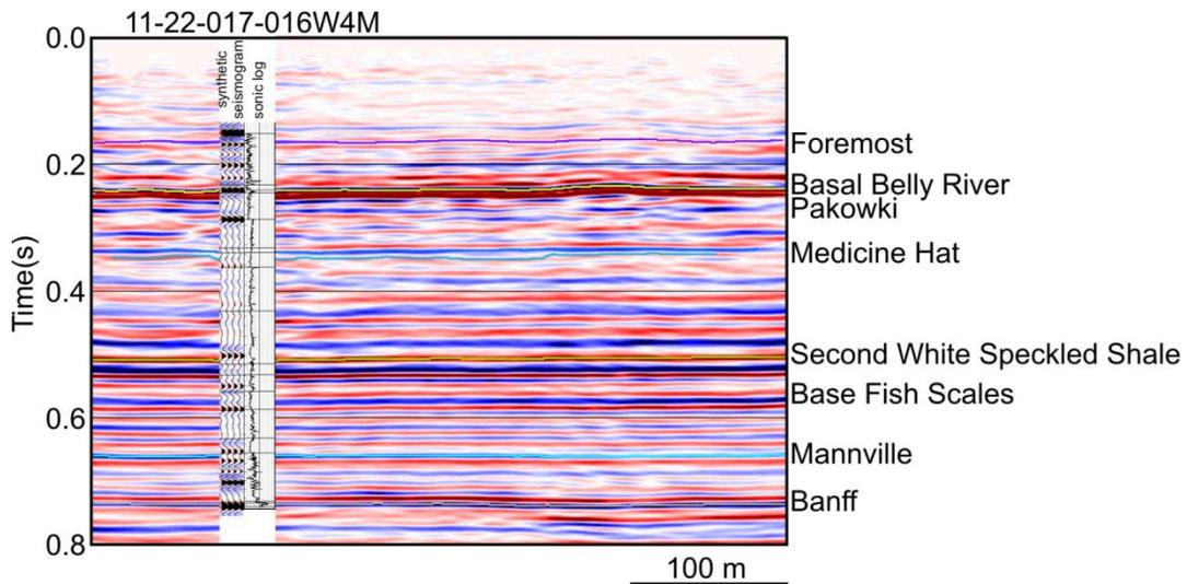
FIG 5: Synthetic seismogram for well 11-22-017-16W4M and the crossline with interpreted horizons.
