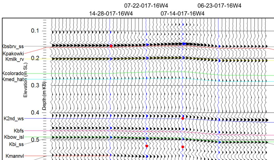
FIG. 6: Synthetic seismogram cross-section using local wells. The reservoir sands are usually too thin to be identified by seismic signature but there are subtle changes in the character of events when gas is present (red dots).
