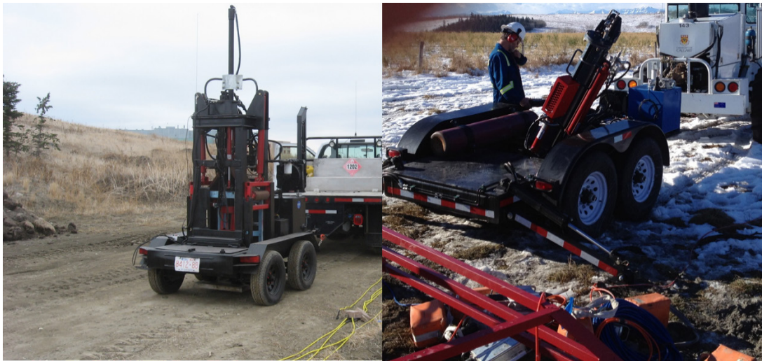
FIG. 7. The recently retired P-wave thumper on the left and the replacement P/S-wave thumper on the right.
