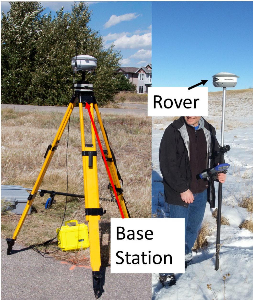
FIG. 8. The two main parts of the differential GPS system, the base station and the rover.
