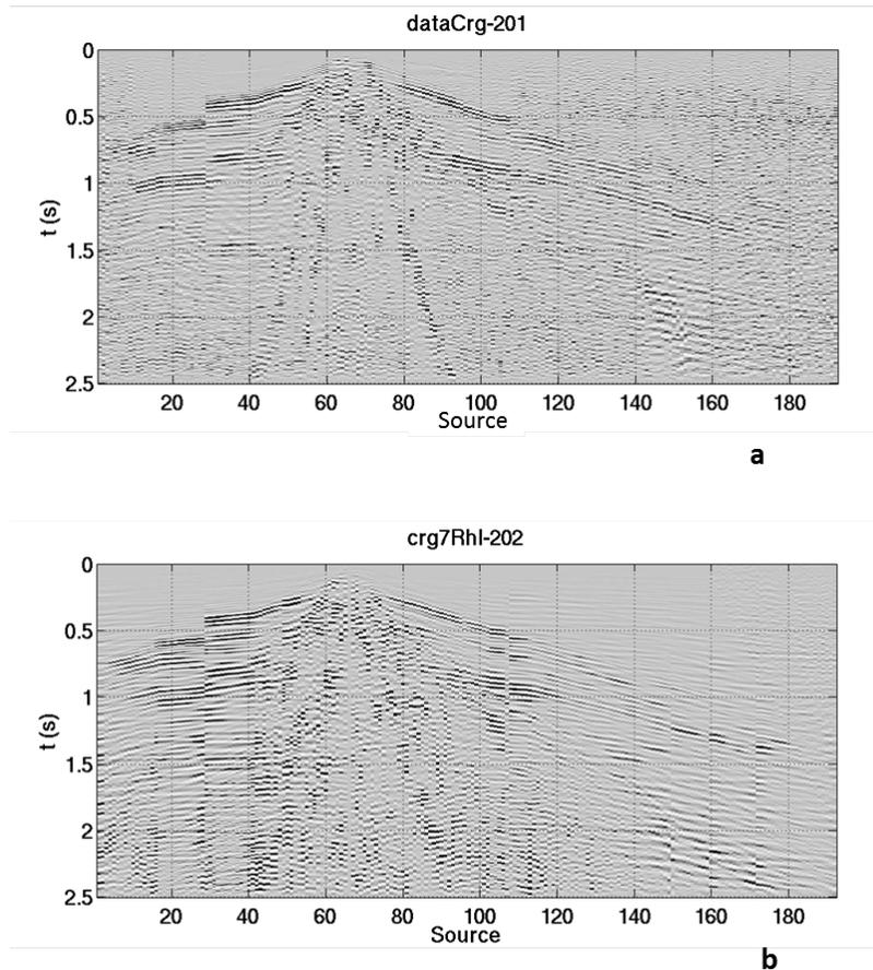
FIG. 3. Data corresponding to the crosscorrelation of CRG 201 from left to right hand side. (a) CRG 201 (b) CRG 202 interpolated, such that the offsets are the same that in the case of CRG 201.
