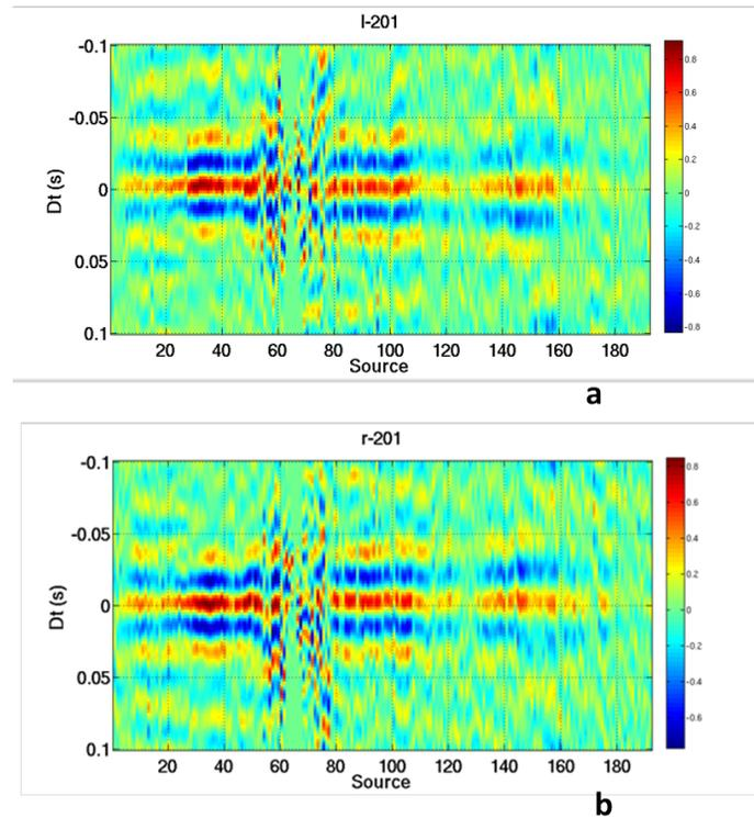
FIG. 4. Crosscorrelation of the traces in CRG 201 (a) Left to right direction. (b) Right to left direction. Notice the opposite polarity between these two directions.
