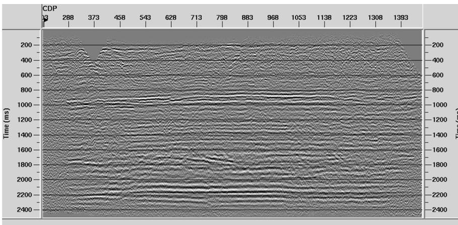
FIG. 12. Stack section using the receiver statics obtained with the CRS method.
