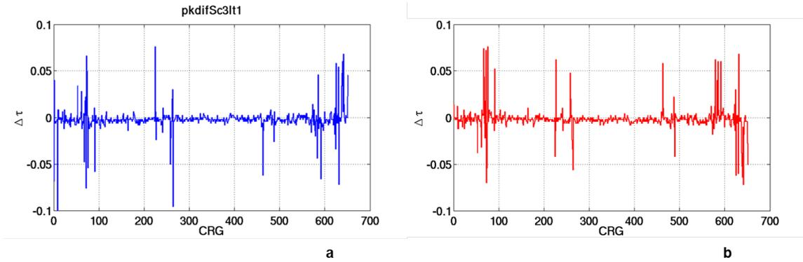
FIG. 8. Time delay for maximum picks on the crosscorrelations for both directions, obtained from the crosscorrelation stacks. (a) Left to right. (b) Right to left. Notice that Figure 8(a) is close to the inverse in  $\Delta\tau$  of Figure 8(b) however with a bias of about -2 ms, and that there are a number of outliers, (values higher than 0.02 s).
