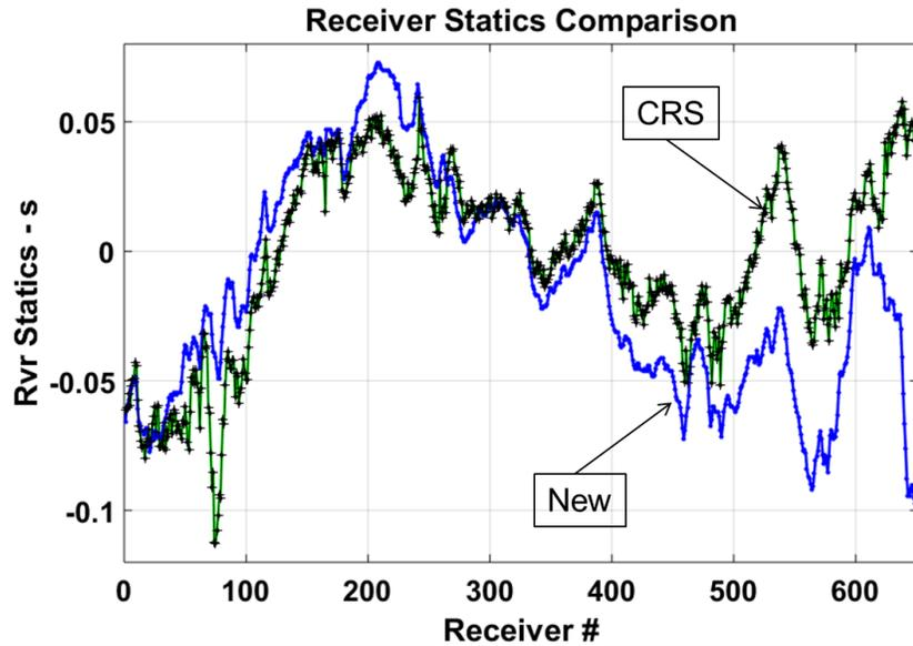
FIG. 10. Comparison of receiver statics delays using the CRS method and the new method.
