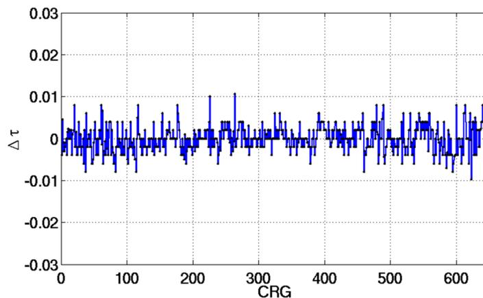
FIG. 9. Differential receiver statics after bias correction and edition of outliers. For the bias correction the results of Figure 8 are subtracted and divided by two.
