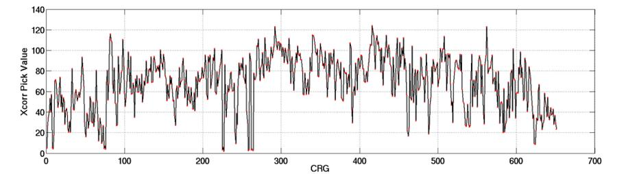
FIG. 7. Maximum picks on the crosscorrelations, obtained from the crosscorrelation stacks (Figure 6). The maximum possible value is 192, and low values correspond to lack of reliable data.
