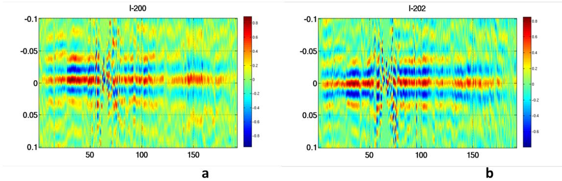
FIG. 5. Crosscorrelations results of the traces in CRG adjacents to CRG 201, in the direction left to right. (a) CRG 200, (b) CRG 202. Comparing with Figure 4(a) and ??(a) notice a subtle delay.
