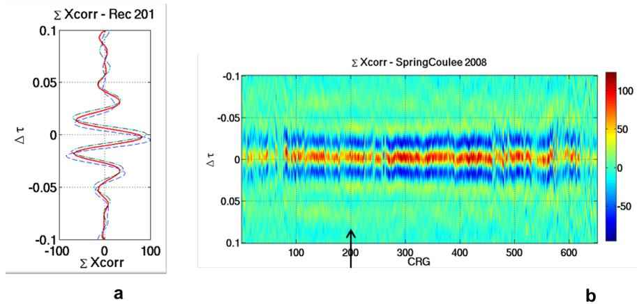
FIG. 6. Crosscorrelation stacks in the direction left to right for all receivers. (a) Individual stacks for CRGs 200 (blue dashed line), 201 (solid red) and 202 (black dash dotted). (b) Stacks for each one of the CRGs; the location of the selected in Figure (a) is shown by an arrow.
