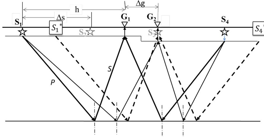
FIG. 1. Ray sketch of traces affected by receiver statics, that shows the  $PS$  events used for cross-correlation in the receiver statics algorithm. The traces of a CRG have the same  $R_i$  delay. The time delay between traces corresponds to the differential source and receiver time delays in the NS-LVL, plus the offset and geological time delays. Each trace of a CRG is crosscorrelated with the trace of the adjacent CRG corresponding to the same offset to obtain  $R_i$ .
