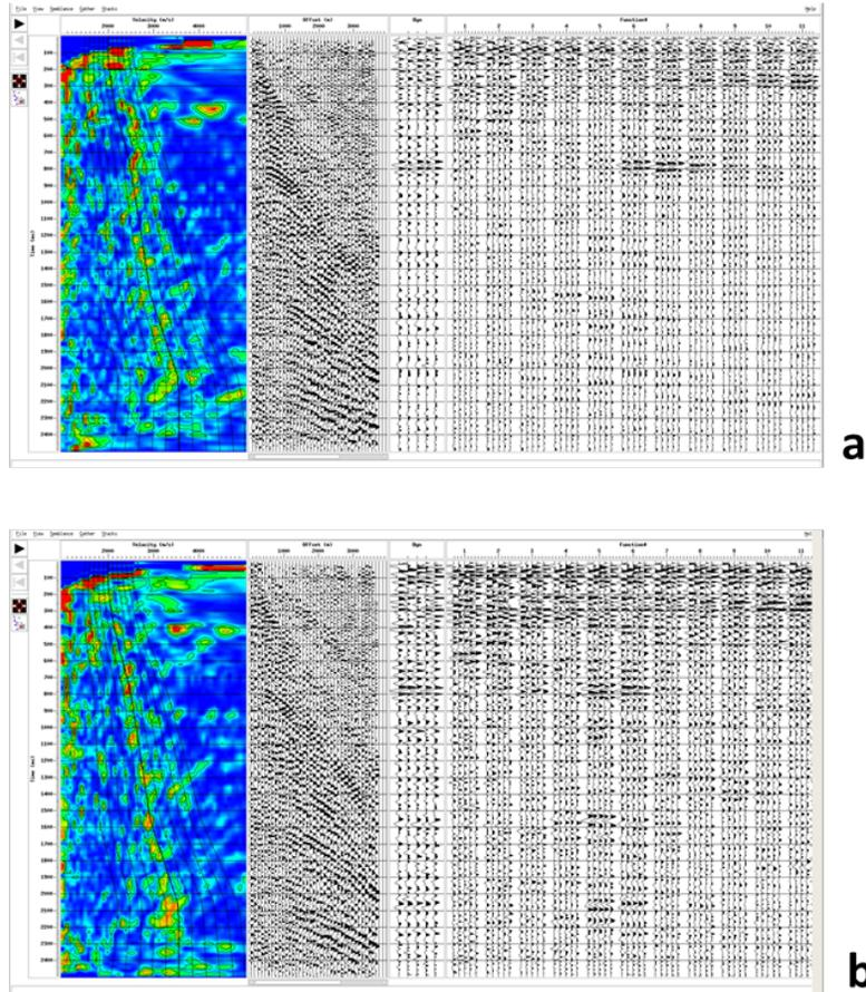
FIG. 13. Comparison of the receiver statics effect on Velocity analysis of a CDP. (a) Without the receiver statics correction. (b) With the receiver statics correction: the events are easier to follow.
