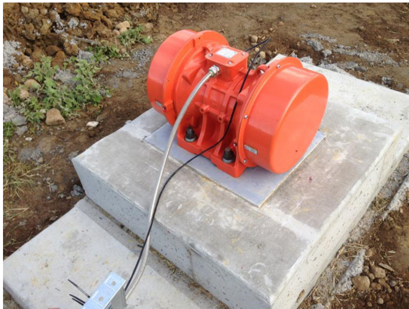
FIG. 5. LBNL permanent seismic source. Image courtesy of Barry Freifeld (LBNL), Curtin University and the Australian CO 2 CRC.
