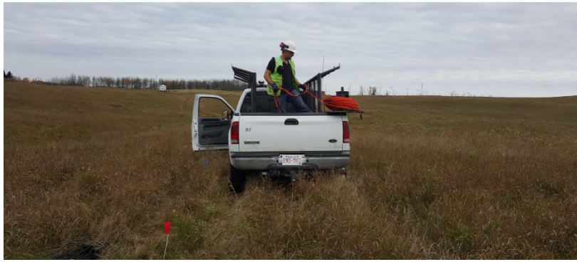
FIG. 14. Laying out the cable with the recorder in the distance.
