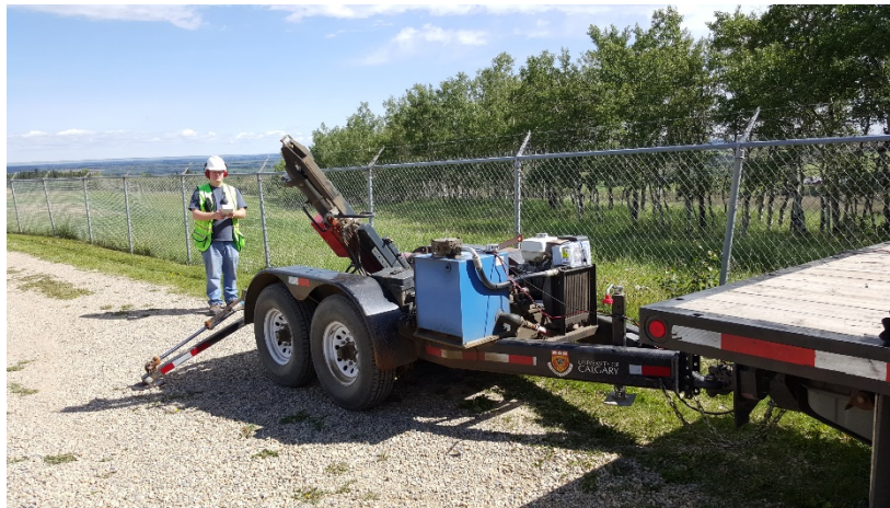
FIG. 6. The accelerated weight drop trailer tilted for an s-wave shot.
