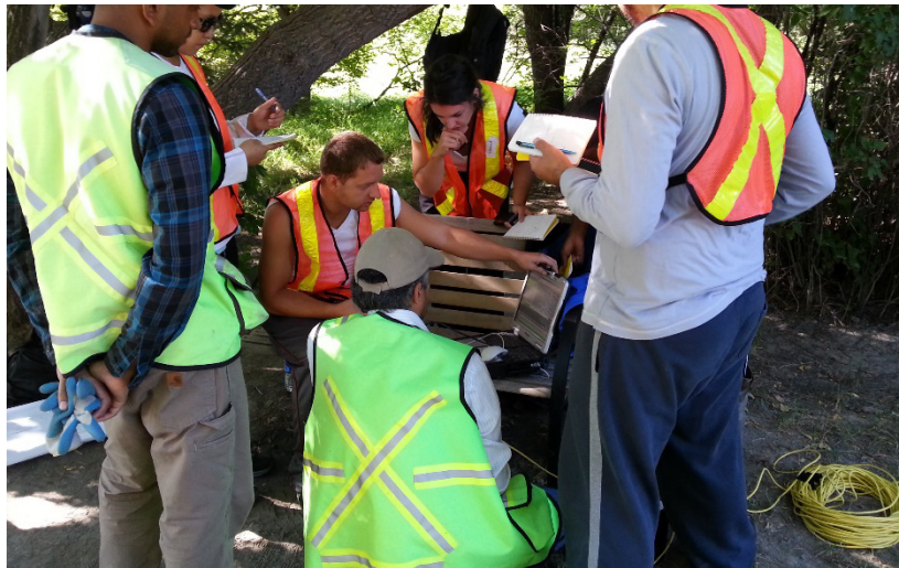
FIG. 3. The Geometrics Geode system being used with a laptop and a hammer and plate source.
