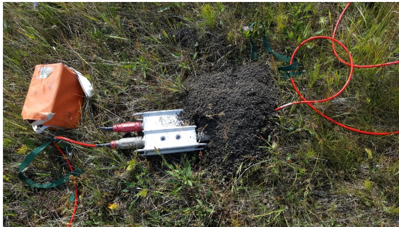
FIG. 1a. An Aries eight channel RAM with battery and dirt.
