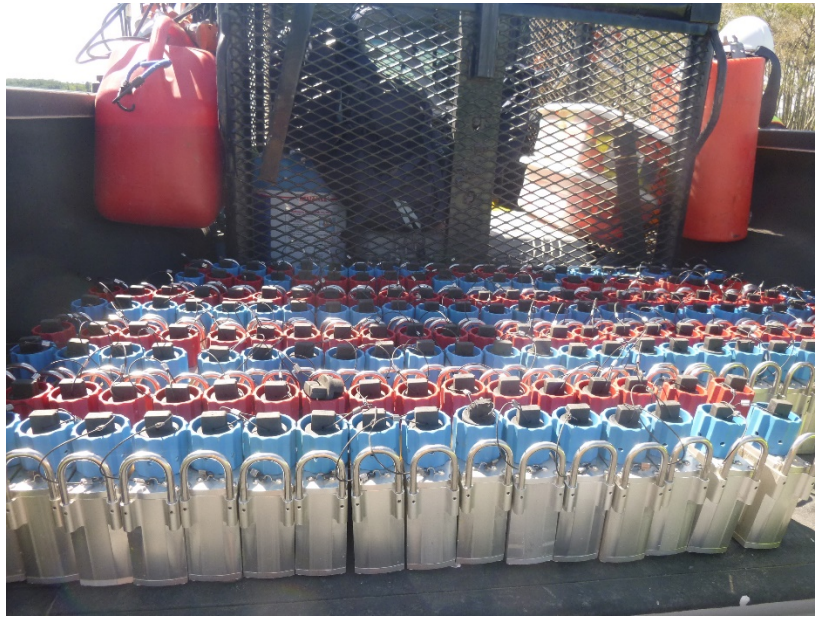
FIG. 2. Hawk node, each one connects to a battery and three analogue or digital channels.
