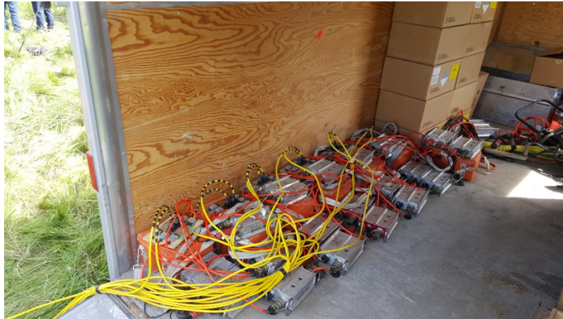
FIG. 5. Custom built adapter boards to convert the Weir-Jones downhole geophones to Aries recording system.
