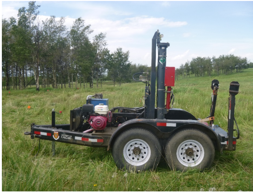
FIG. 8. The shear wave accelerated weight drop thumper.
