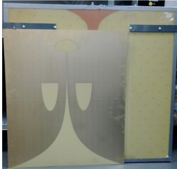
FIG. 1. Two uwb antennas. In the foreground is shown the smaller tapered slot antenna that will be used for the array trolley (Yedlin et al., 2016).
