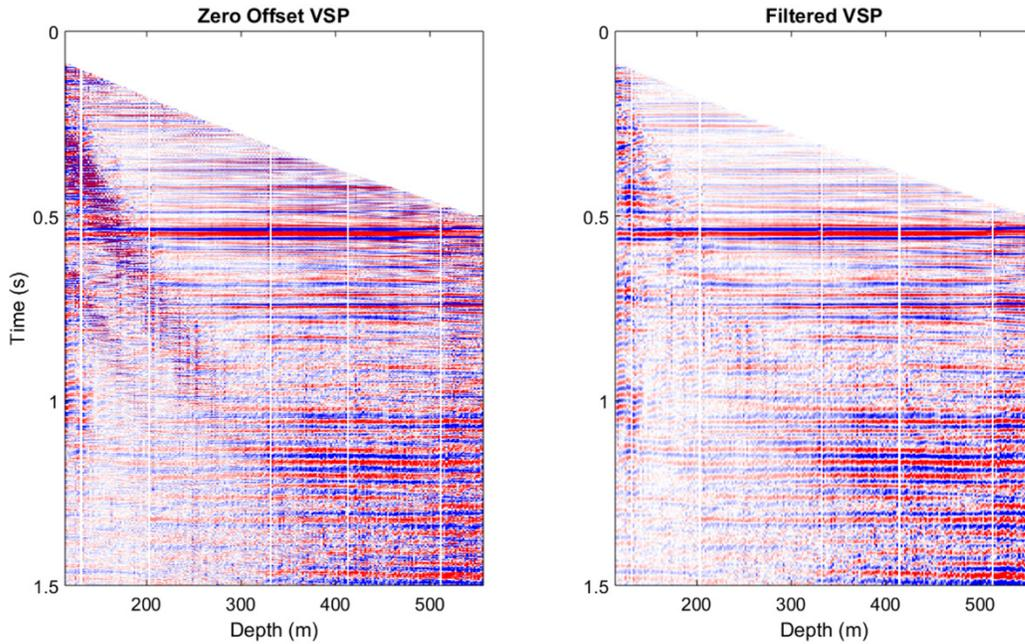
FIG. 10. Zero offset VSP data (left), and VSP data filtered with a high cut Butterworth filter (right).
