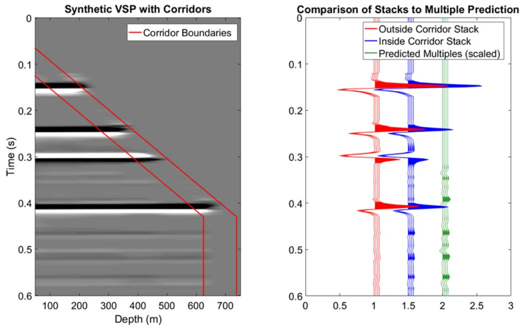
FIG. 7. VSP dataset with overlain corridors (left), outside corridor stack (red), inside corridor stack (blue), internal multiple prediction (scaled, green).
