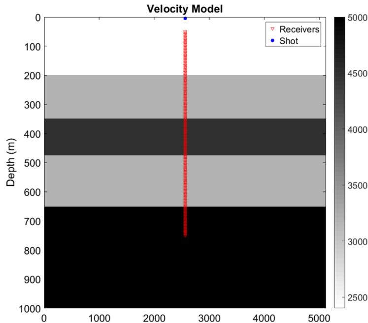
FIG. 1. Synthetic velocity model used to construct zero offset VSP, the red triangles represent the receiver locations (receiver spacing = 10m), blue circle indicates the shot location.
