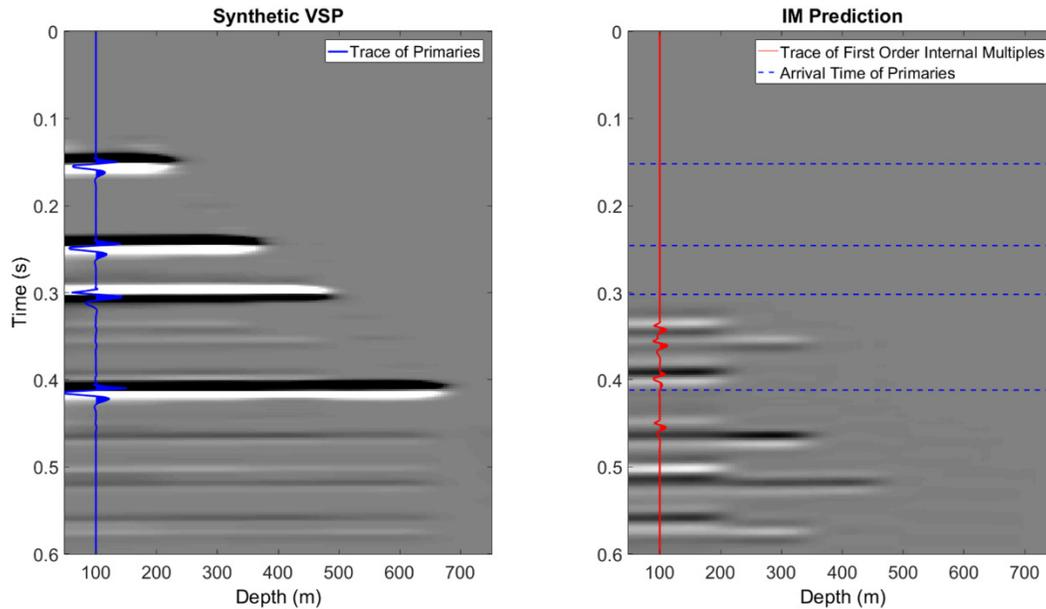
FIG. 6. Flattened upgoing wavefield (left), internal multiple prediction (right). The blue trace shows the trace containing only primaries, while the red trace shows the trace of first order internal multiples. The dashed blue lines indicated the arrival time of the primaries.
