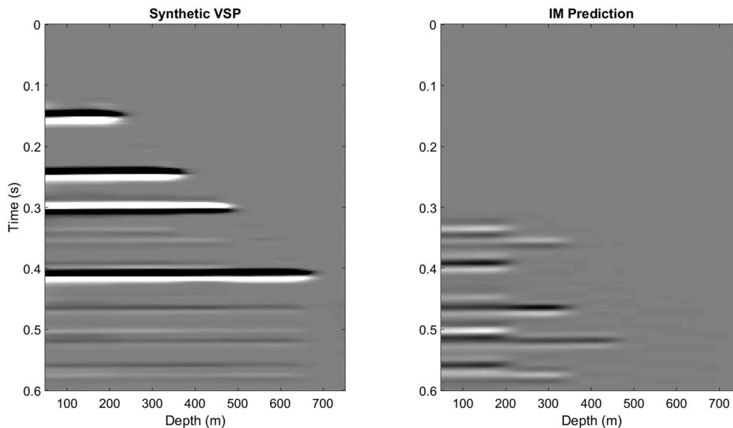
FIG. 5. Flattened upgoing wavefield (left), internal multiple prediction (right).
