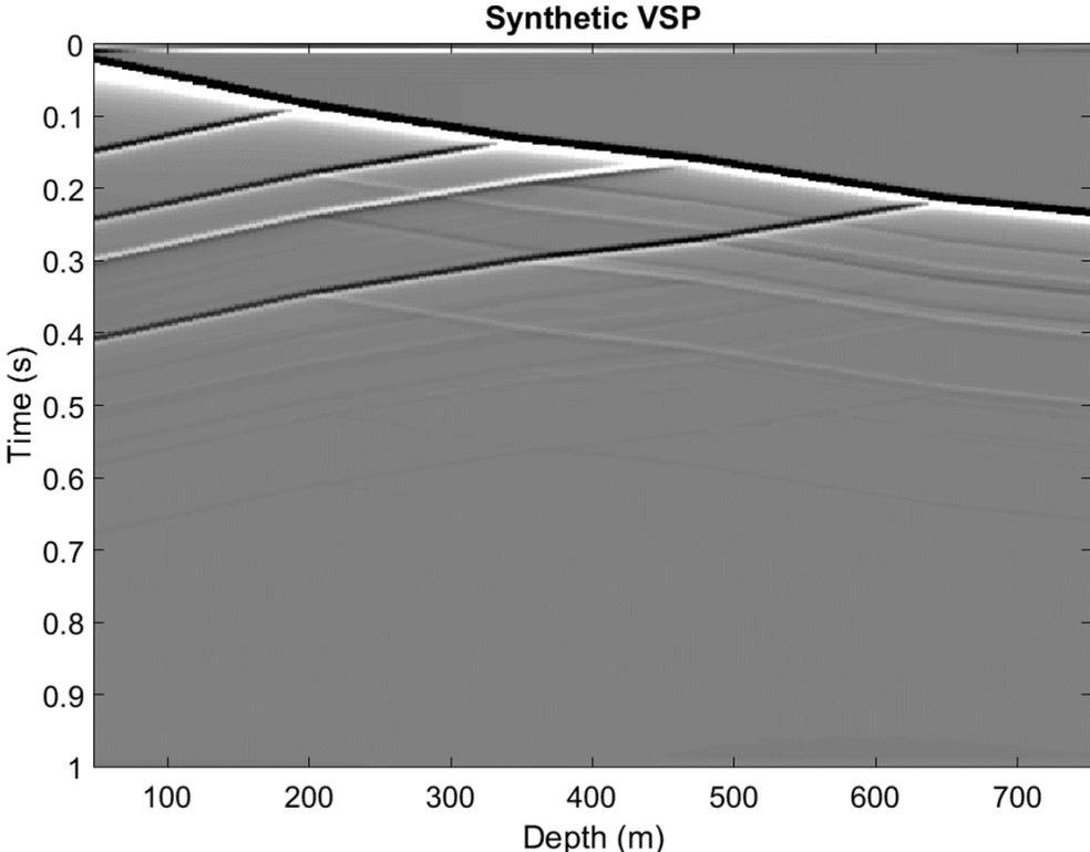
FIG. 2. Synthetic vertical seismic profile before processing.
