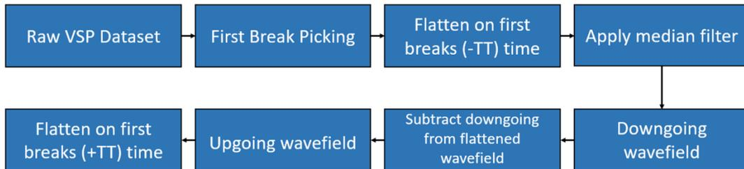
FIG. 4. Flow chart of the processing steps applied to go from figure 2 to figure 3.
