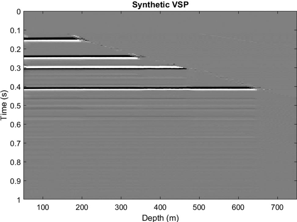
FIG. 3. Synthetic vertical seismic profile after processing.
