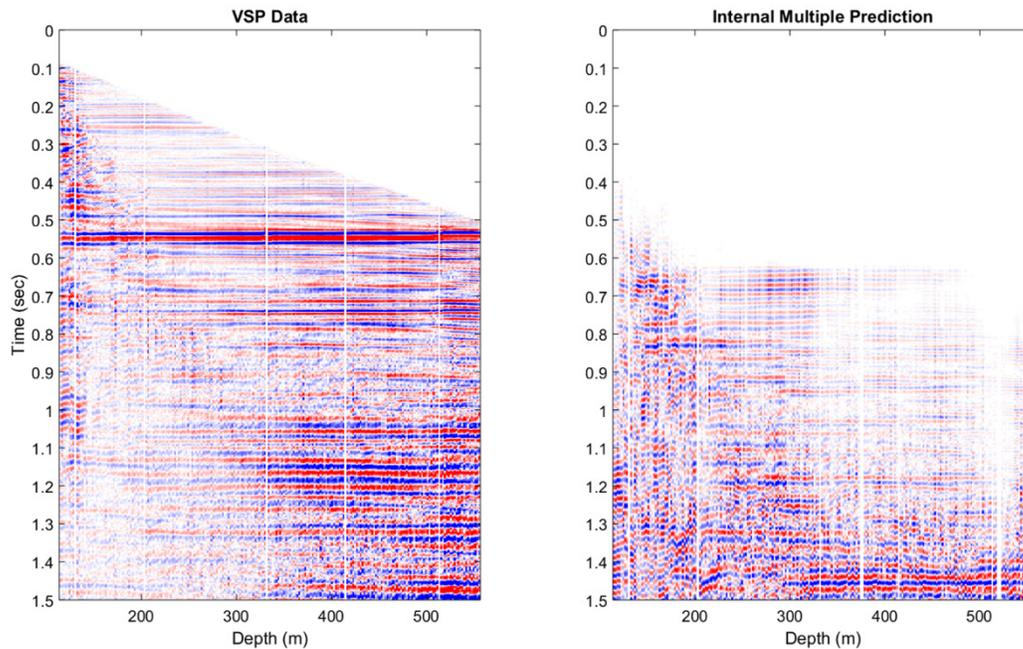
FIG. 12. Filtered zero-offset VSP data (left), time domain internal multiple prediction (right).
