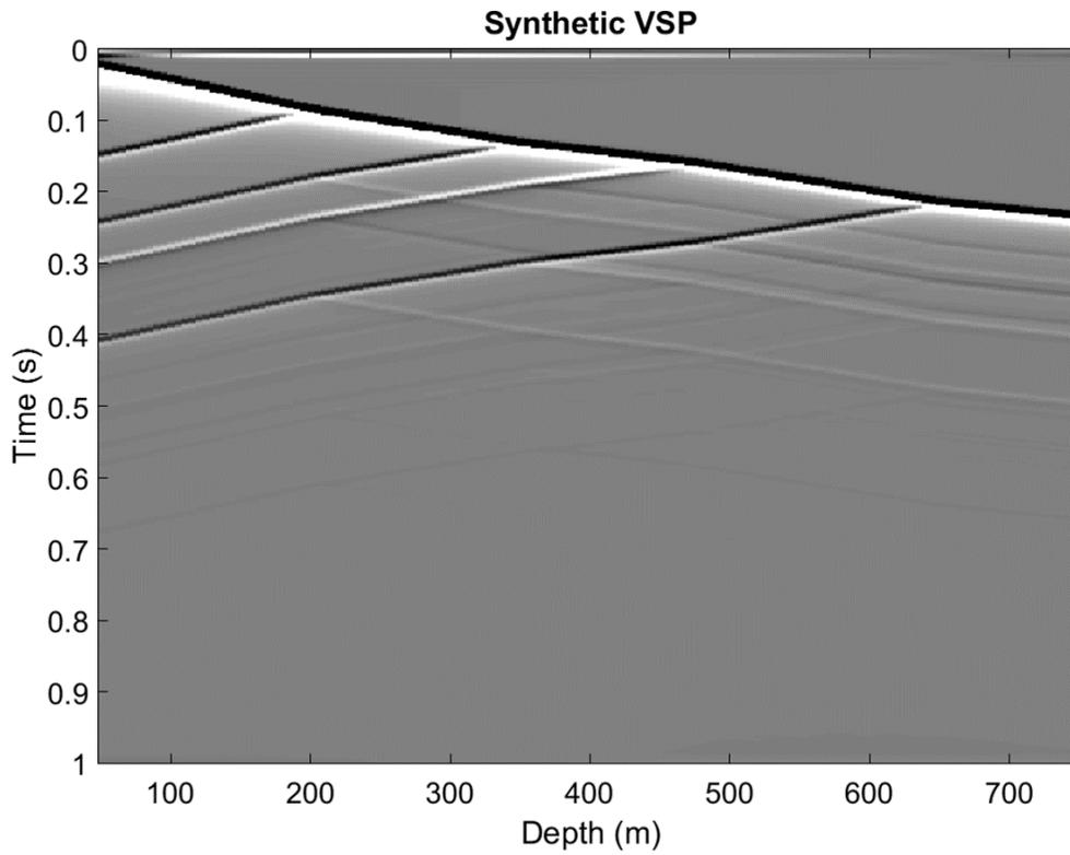
FIG. 2. Synthetic vertical seismic profile before processing.
