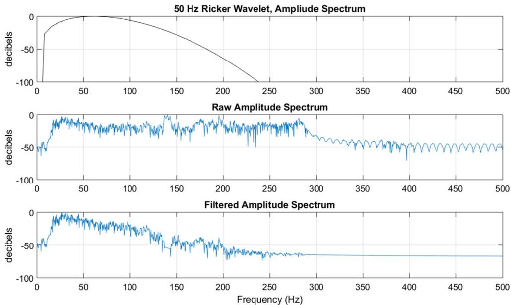
FIG. 11. The amplitude spectrum of a 50 Hz Ricker wavelet (top), amplitude spectrum of the unfiltered amplitude spectrum (middle), filtered amplitude spectrum (bottom).
