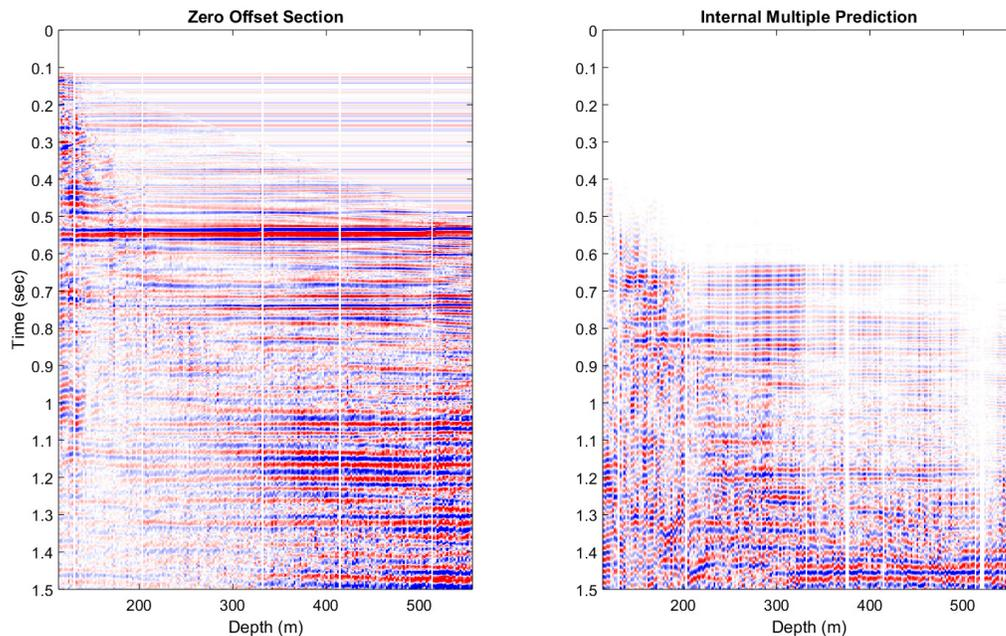
FIG. 13. Filtered zero offset section (left), time domain internal multiple prediction (right).
