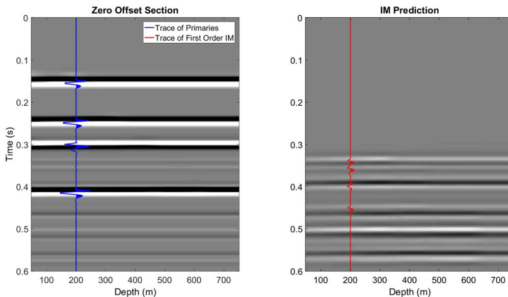
FIG. 9. Zero offset section (left), internal multiple prediction (right). The blue trace shows the trace containing only primaries, while the red trace shows the trace of first order internal multiples. The dashed blue lines indicated the arrival time of the primaries.
