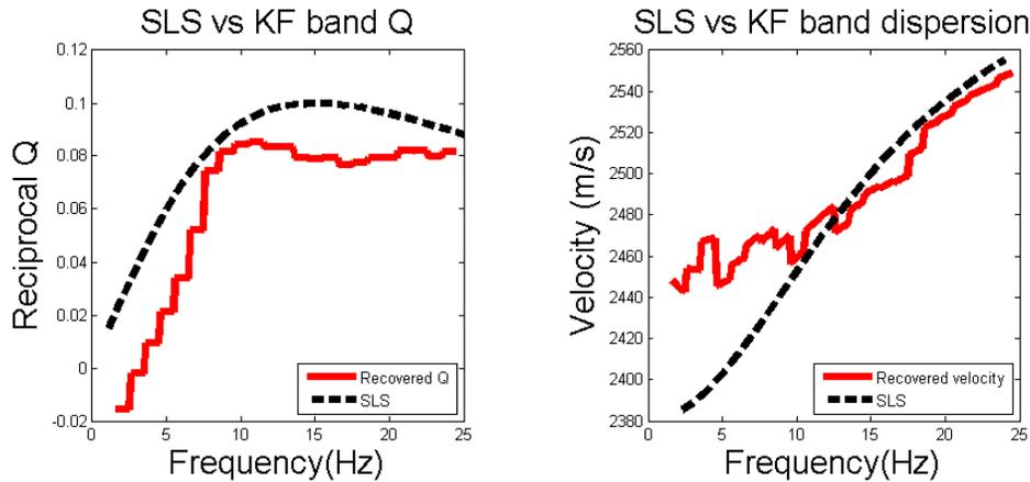
FIG. 9. Average reciprocal  $Q$  and velocity over the non-zero  $Q$  region of the true model. Recovered values using flexible KF method reproduce trend of true values much more accurately than a true KF model can (figure 2). Velocity is poorly recovered at low frequency.
