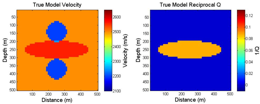
FIG. 4. True model velocity (left) and Q (right) for SLS model type at 25Hz.
