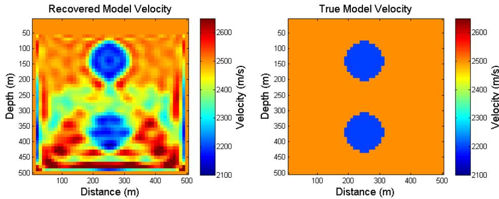
FIG. 5. Recovered velocity (left) and true velocity (right) using acoustic FWI.
