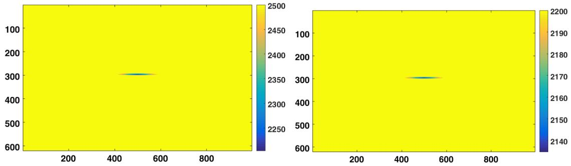
Figure 2: The diffusive velocity and density models for 7% and 3% change in the ellipsoid shape. The ellipsoids diameters are 180\*10m. 6
