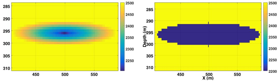
Figure 1: Internal structure of diffusive and solid velocity models. The reduction is linear from the center to the margin in the diffusive model.
