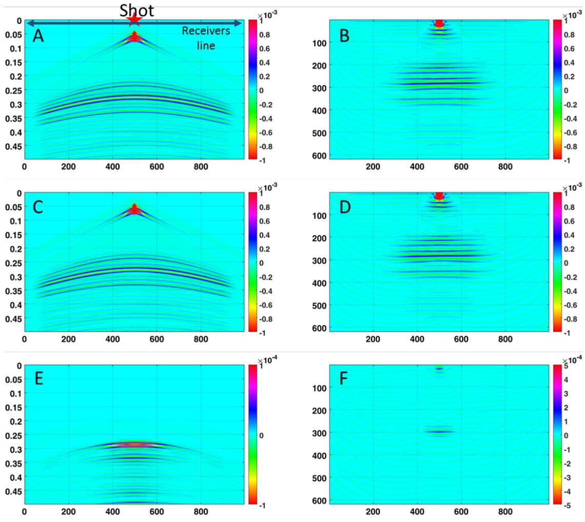
Figure 16: The seismic model generated by the velocity and density patterns introduced in Figure 15 for a surface seismic experience with one shot in  $x=500$  m and receivers with 1 m interval and extension from 0 to 1000 m. A. Baseline seismic model. B. Baseline RTM result. C. Monitor seismic model. D. Monitor RTM result. E. Difference between monitored and baseline seismic models (amplitude ten times magnified). F. Difference between RTM results (amplitude ten times magnified).
