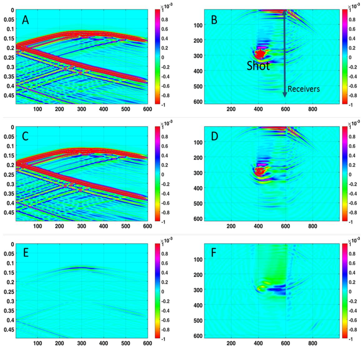
Figure 18: The seismic model generated by the velocity and density patterns introduced in Figure 15 for a Cross-Well experience with one shot in  $x=400$  m and 295 m depth and receivers with 1 m interval in  $x= 600$  and extension from 0 to 600 m depth. A. Baseline seismic model. B. Baseline RTM result. C. Monitor seismic model. D. Monitor RTM result. E-Difference between monitored and baseline seismic models. F. Difference between RTM results.
