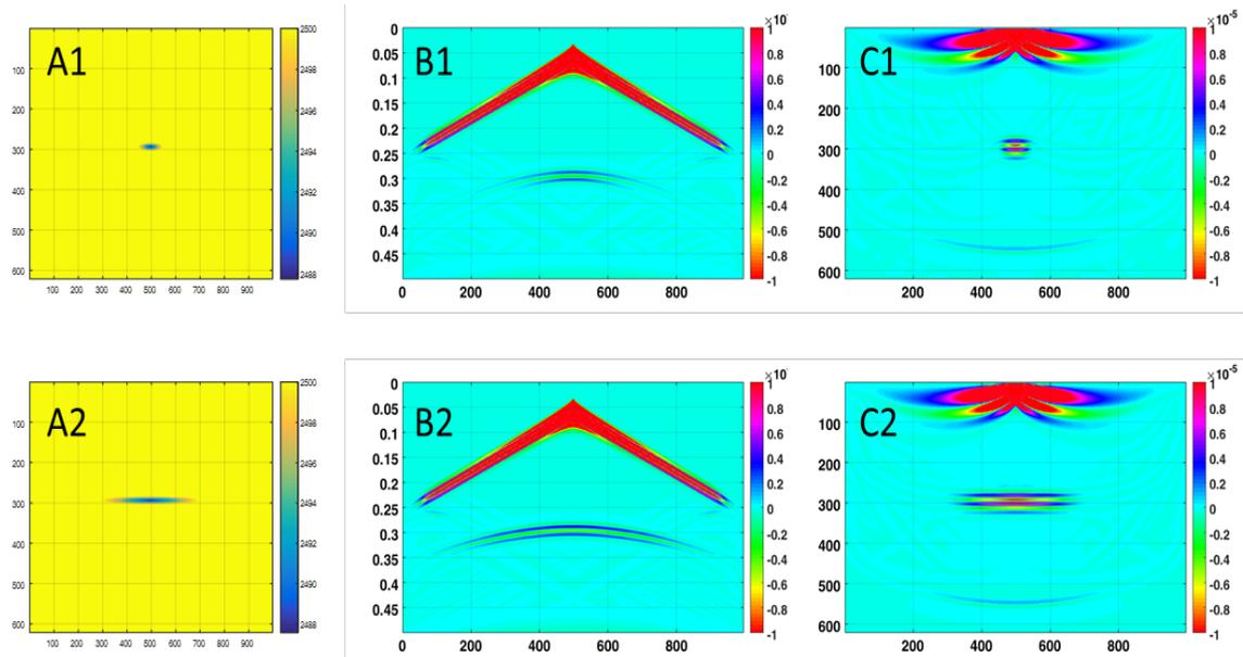
Figure 8: The seismic response and RTM result for two models with a different plume size and 5% velocity change in the center of ellipsoids. A1: 50\*20 m A2:200\*20 m.
