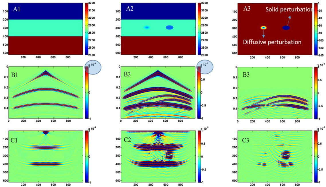
Figure 6: The figure shows (row A) a simple 3-layer media with and without two velocity change ellipsoids (solid and diffusive change). The second row (B) is seismic responses (FWI acoustic, pressure component). The amplitude of the B2 and B3 are ten times more than B1 to demonstrate diffusive perturbation's response. The third row (C) are imaging result by RTM method.
