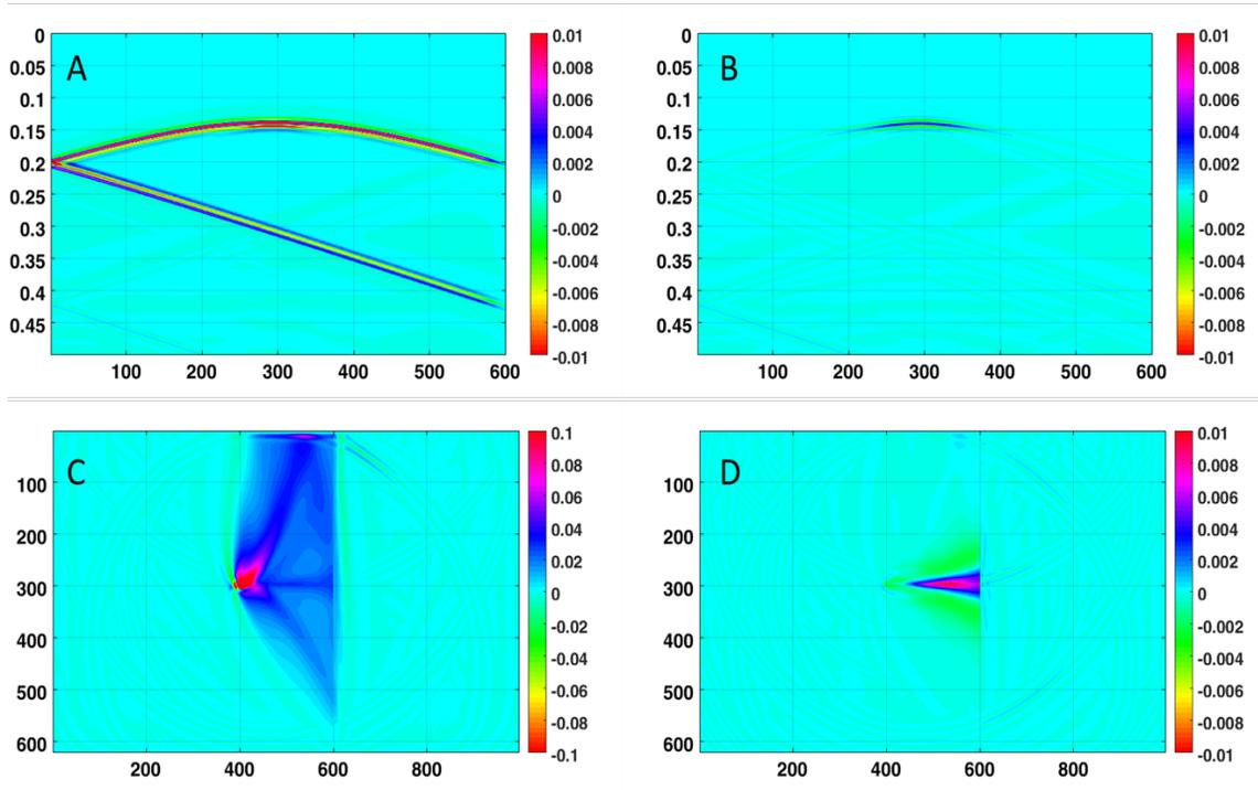
Figure 5: A: The seismic response of the models in Figure 2. B: After eliminating the surface and shot effects. C: The migrated data (from A). D: The noise reduced migrated section. E: Section D in the higher amplitude.
