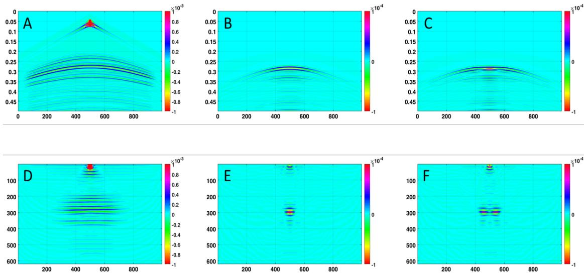
Figure 19: The time lapse seismic models: A. The seismic model for one-year injection. B- The difference between the baseline and A. C. The difference between seismic models after five and one-years' injection. D. Migrated section of A. E. Difference of migration sections between the baseline and one year's injection data. F. Difference of migrated data between five years and one-year injection data.
