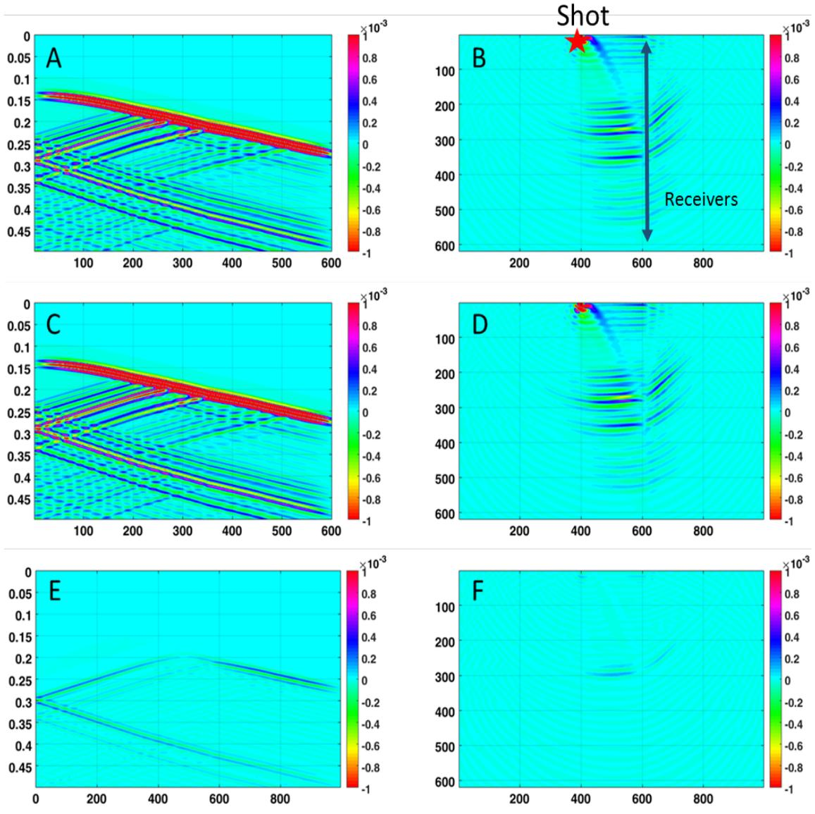
Figure 17: The seismic model generated by the velocity and density patterns introduced in Figure 15 for a VSP experience with one shot in  $x=400$  m and receivers with 1 m interval in  $x=600$  and extension from 0 to 600 m depth. A. Baseline seismic model. B. Baseline RTM result. C. Monitor seismic model. D. Monitor RTM result. E. Difference between monitored and baseline seismic models. F. Difference between RTM results.
