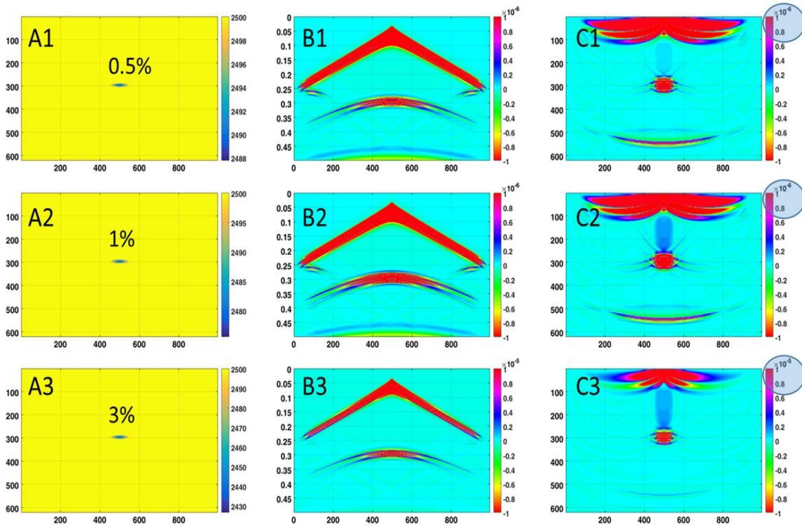
Figure 7: The seismic response and RTM result for a model (100 \* 20 m) with a different velocity. Higher velocity difference caused greater amplitude for the surface acquisition survey.
