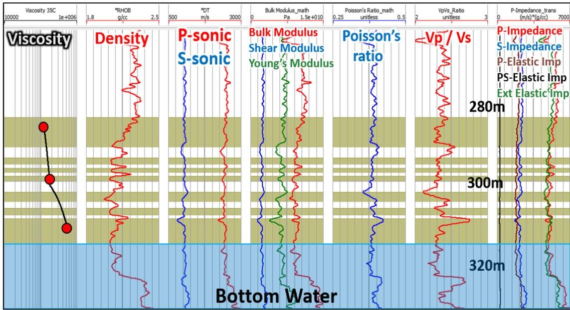
FIG. 14. Type well of the project area with calculated seismic properties. The red dots in the left track are the provided viscosity measurements and the black curve is the interpolated target viscosity log. The viscosity is presented on a logarithmic scale from 10,000 cP to 1,000,000 cP. The gold zones highlight the training intervals (with mud barriers being avoided).
