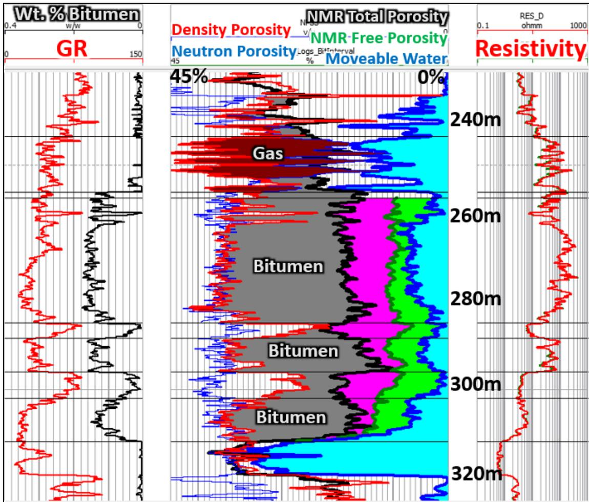
FIG. 17. Oil sands well in the study area with NMR data. The density porosity and NMR total porosity curves overlap above and below the hydrocarbon zones, but separate in the bitumen zones. The grey filled area is bitumen, the filled magenta area is hydrocarbon in small pores and capillaries (seen by NMR), the filled green area is free hydrocarbon in medium pores (seen by NMR), and filled blue is free fluids in the larger pores (seen by NMR).
