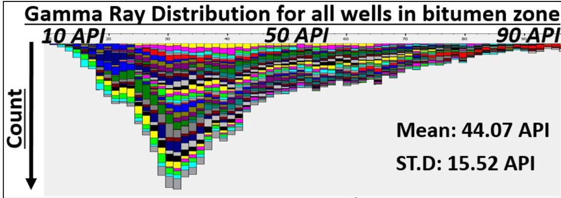
FIG. 10. Distribution of the gamma ray values for all wells from top to base of the gross bitumen interval. Each color represents a different well.
