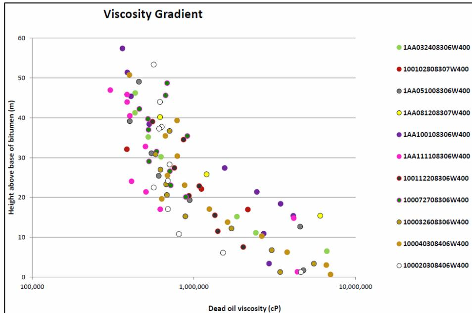
FIG. 3. Core sample viscosity measurements of the McMurray formation from ConocoPhillips's Surmont SAGD oil sands operation, located only 10km south of the study area. This data shows that bitumen viscosity increases with depth in the McMurray formation (ConocoPhillips 2015).
