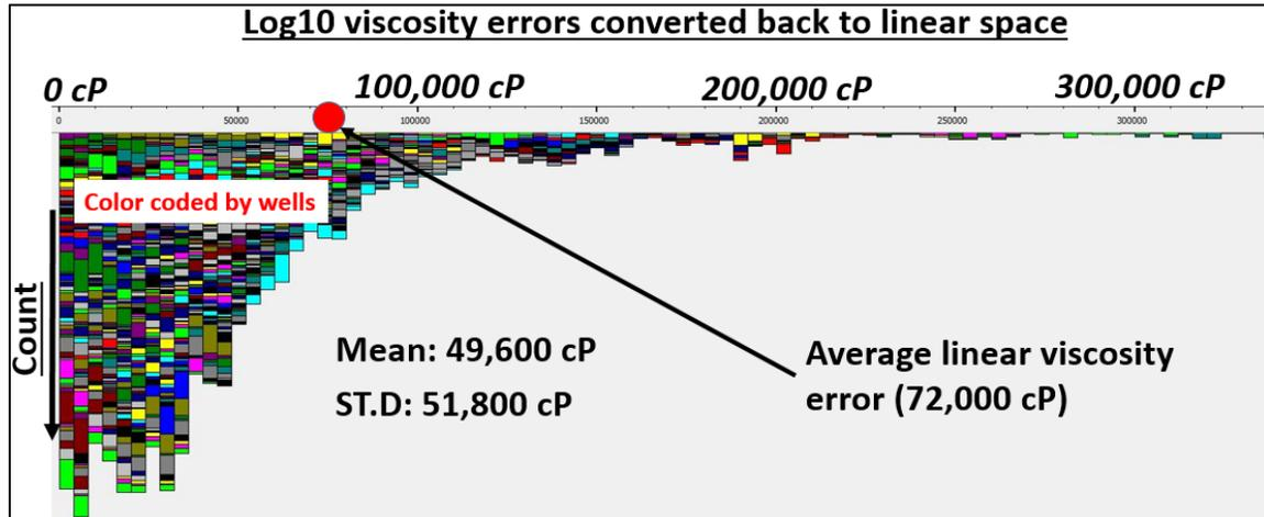
FIG. 13.  $\log_{10}(\text{viscosity})$  prediction errors converted back to linear space.
