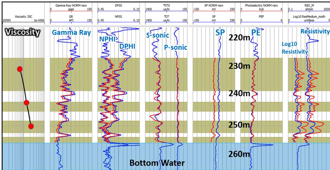
FIG. 11. What the normalized logs look like (red) versus the un-normalized logs (blue). The normalization was focused from top to base of the gross bitumen interval. The gold zones highlight the bitumen intervals.
