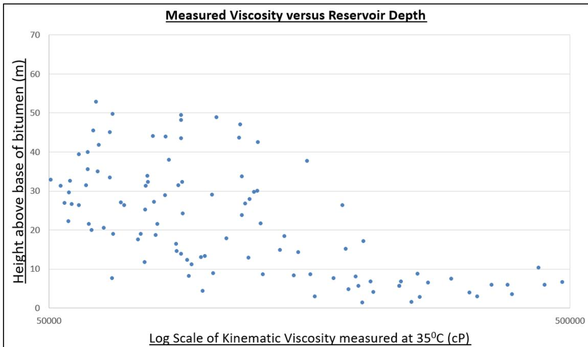
FIG. 22. Reservoir depth vs. viscosity plot. All the viscosity measurements from the 40 study wells are plotted.
