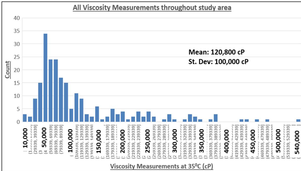
FIG. 8. Distribution of all the laboratory viscosity measurements throughout the study area.
