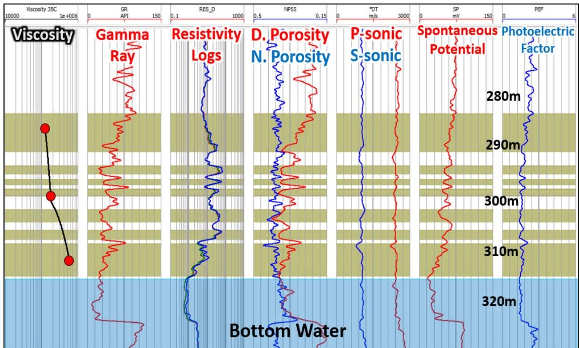
FIG. 9. Type well of the project area. The red dots in the left track are the provided viscosity measurements and the black curve is the interpolated target viscosity log. The viscosity is presented on a logarithmic scale from 10,000 cP to 1,000,000 cP. The gold zones highlight the training intervals (with mud barriers being avoided). There is bottom-water present at the base of the reservoir, based on the low resistivity, high porosity, and high sand content.
