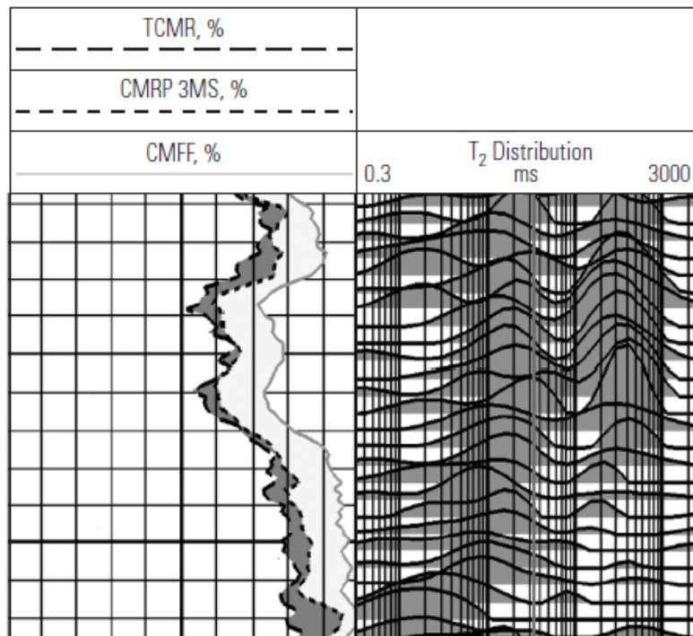
FIG. 16. NMR *T<sub>2</sub>* distributions as a function of depth are shown in the right track. The left track shows the free-fluid, capillary-bound, and clay-bound porosities calculated from the *T<sub>2</sub>* amplitudes (Ellis & Singer 2007).
