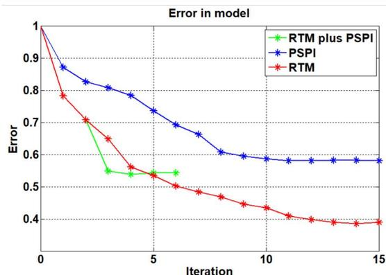
FIG. 15. Error in inverted model for PSPI, RTM and the combination of both of them.
