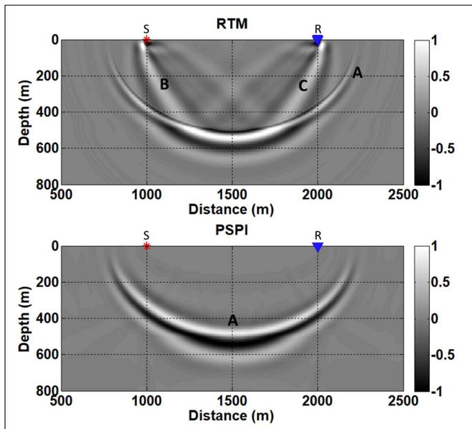
FIG. 2. PSPI and RTM applied to the 1000-m offset trace of figure 1 with cross-correlation imaging condition.
