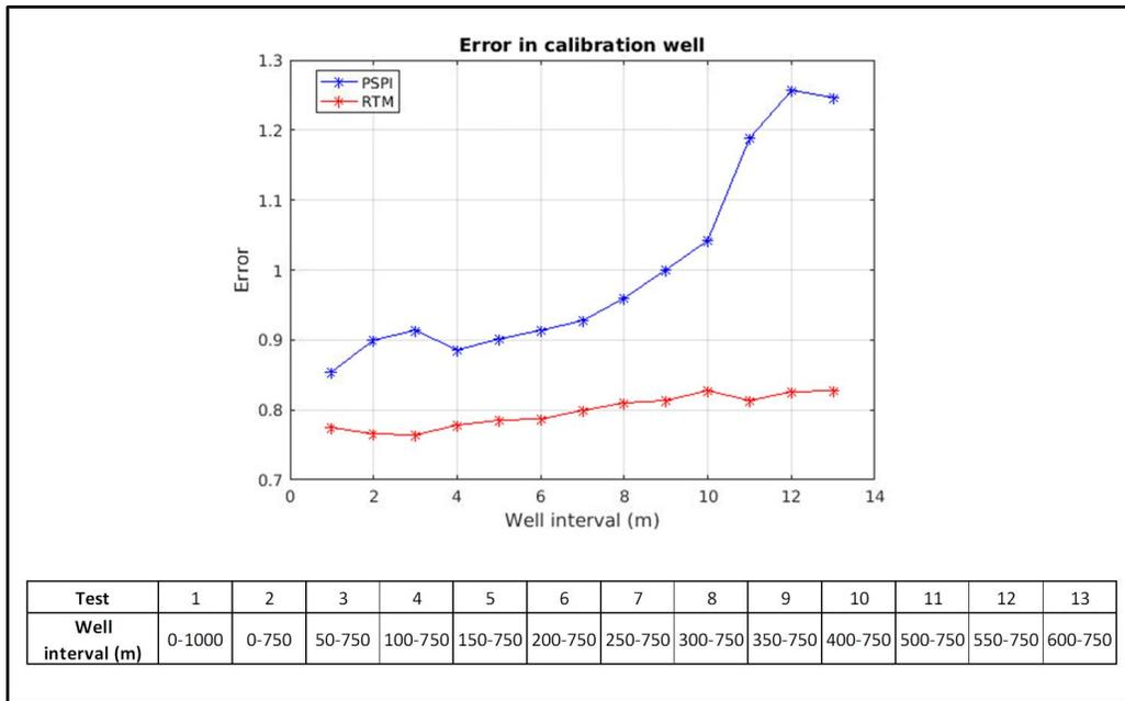
FIG. 16. Sensitivity of PSPI and RTM with well interval coverage for the first iteration (1-6 Hz).
