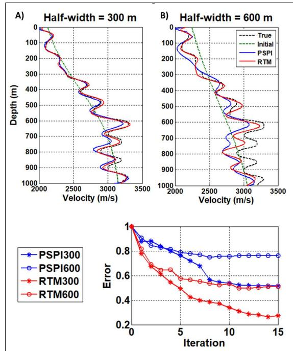
FIG. 13. Sensitivity to the initial velocity model of PSPI and RTM. A) Gaussian smoother half-width = 300 m. B) Gaussian smoother half-width = 600 m.
