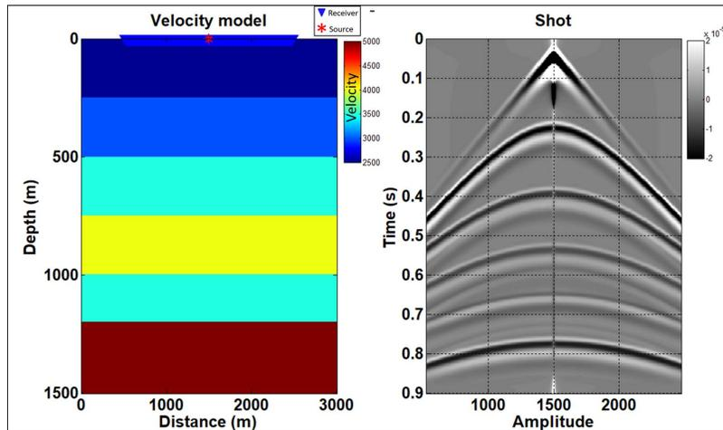
FIG. 3. Horizontal layered model used to generate the shot shown to the right hand side.
