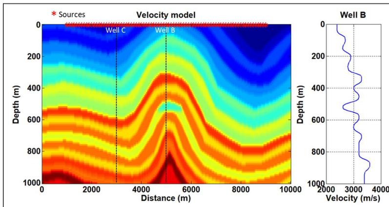
FIG. 5. Velocity model to be solved in the inversion.
