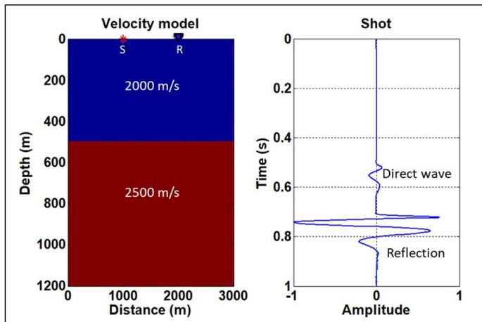
FIG. 1. Seismic trace generated by finite-difference modelling through a single interface model.
