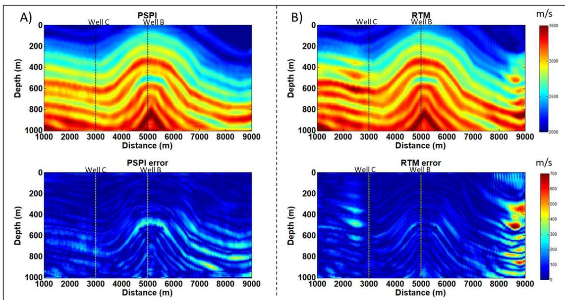
FIG. 11. Final inverted model after 15 iterations: A) PSPI and B) RTM.
