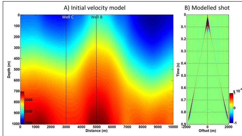
FIG. 7. A) Initial velocity model. B) Synthetic shot modelled by finite differences through the initial velocity model.
