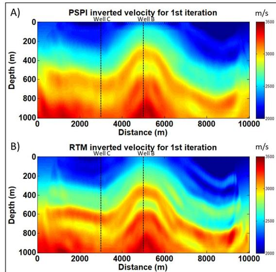
FIG. 10. Inverted velocity model for iteration 1 that result of summing up the velocity update and the initial velocity model. A) PSPI and B) RTM.
