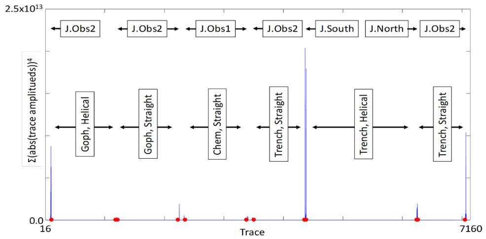
FIG. 3. Square of the sum of squared amplitudes and STA/LTA results (red dots).
