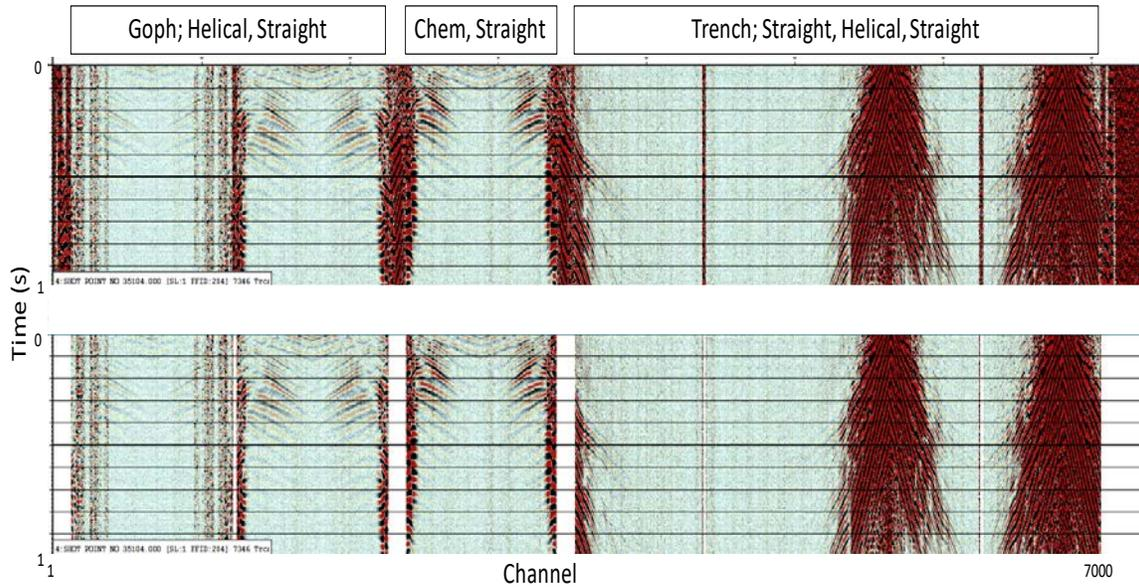
FIG. 8. Correlated data with junction box noise trace mutes calculated using a modified STA/LTA algorithm.
