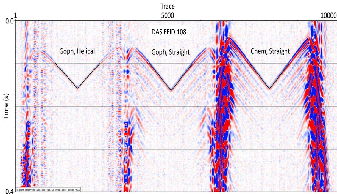
FIG. 9. Example of first break picking (black) across deepest point in each well.
