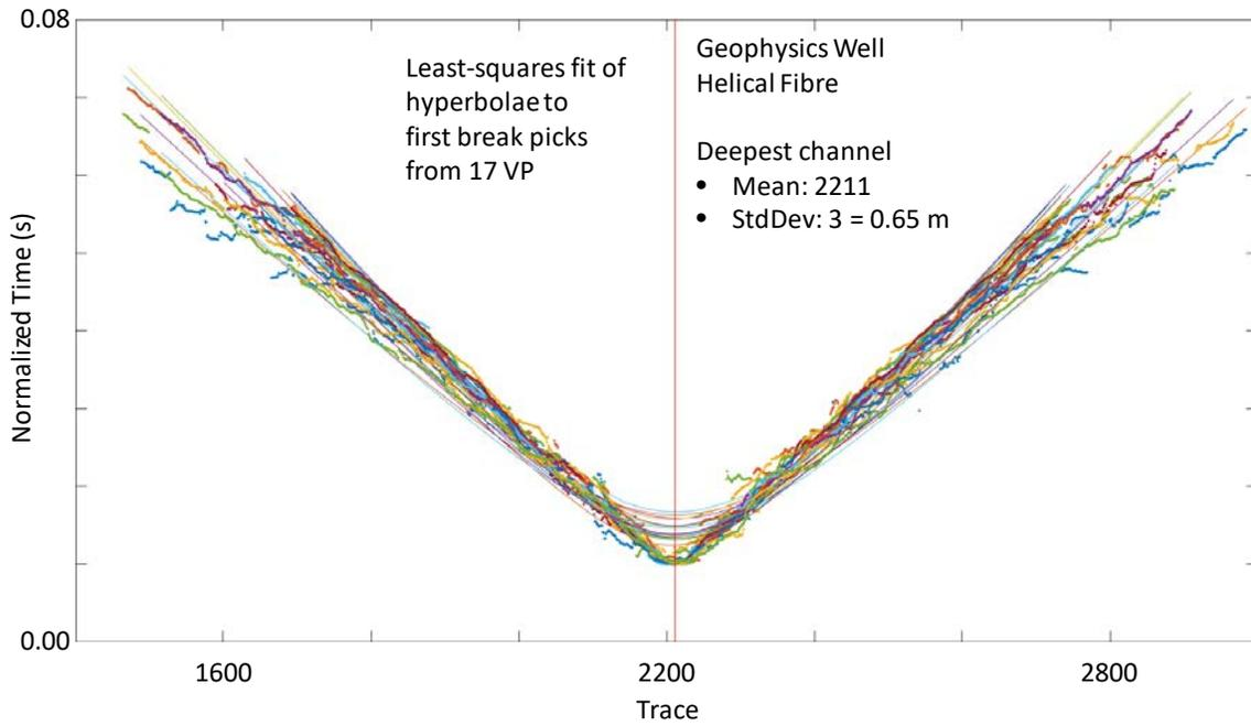
FIG. 10. Geophysics well helical fibre least-squares fit of hyperbolae to first-break picks for 17 VP. Deepest channel=2211 (vertical red line). Standard deviation = 3 traces or 0.65 m.
