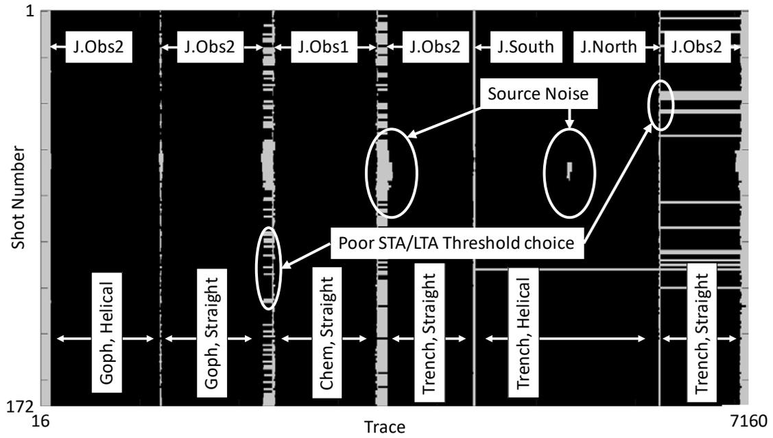
FIG. 5. STA/LTA Threshold = 0.4; Trace range threshold = 100. Black = 1 (keep trace), Grey = 0 (mute trace).
