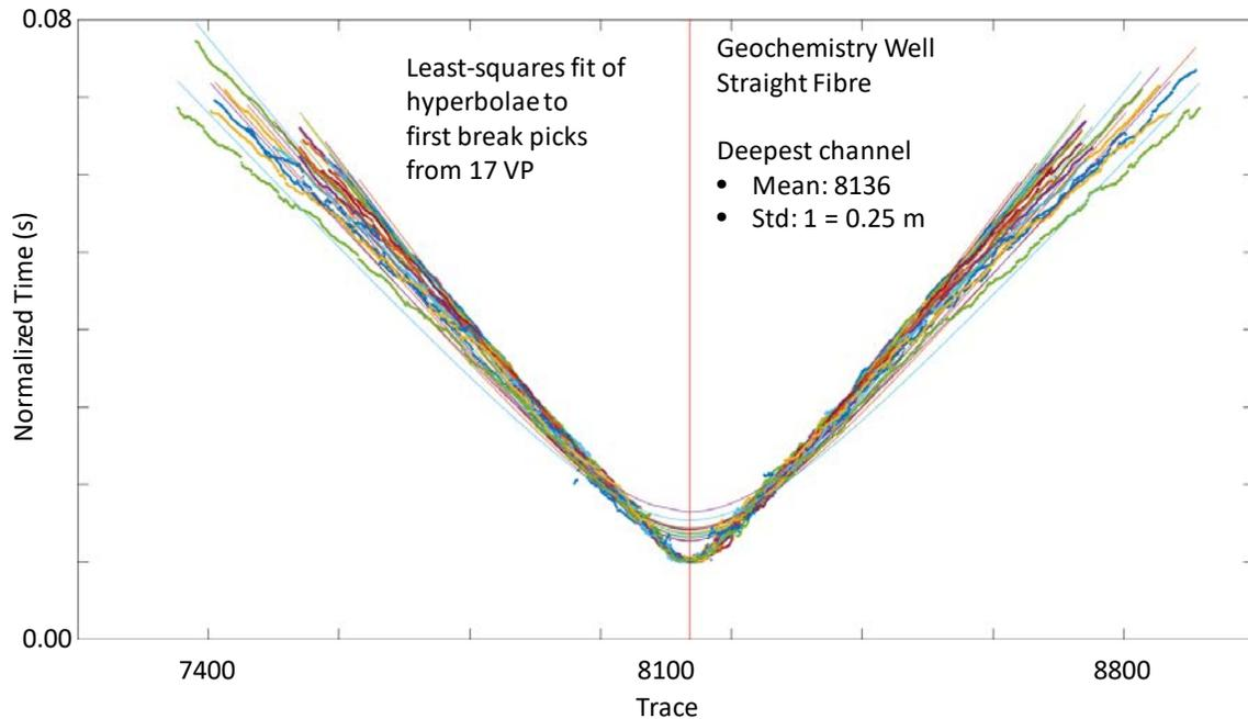
FIG. 12. Geochemistry well straight fibre least-squares fit of hyperbolae to first-break picks for 17 VP. Deepest channel=8136 (vertical red line). Standard deviation = 1 trace or 0.25 m.
