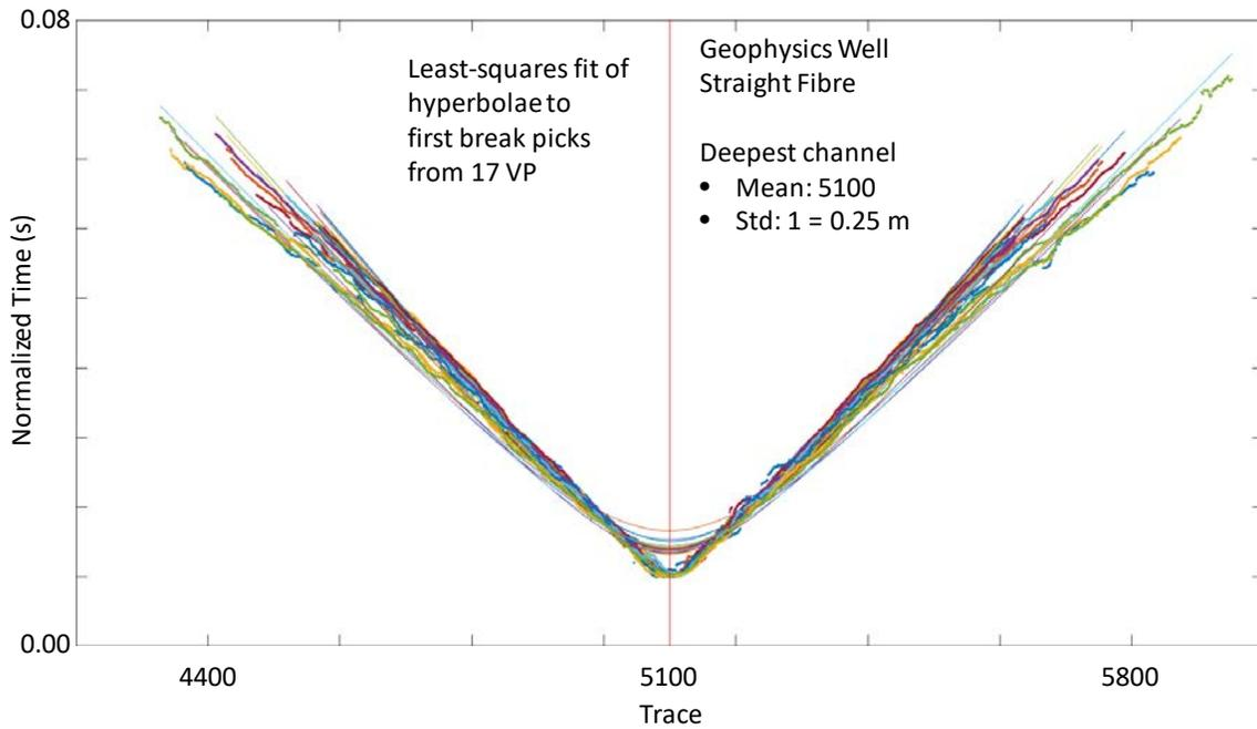
FIG. 11. Geophysics well straight fibre least-squares fit of hyperbolae to first-break picks for 17 VP. Deepest channel=5100 (vertical red line). Standard deviation = 1 trace or 0.25 m.
