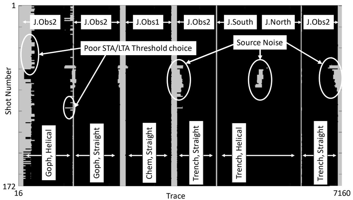
FIG. 6. STA/LTA threshold = 0.001; Trace range threshold = 100. Black = 1 (keep trace), Grey = 0 (mute trace).
