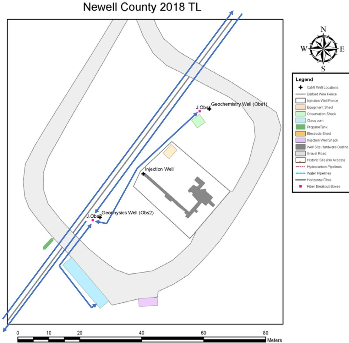
FIG. 1. Wellsite map showing locations of the classroom (light blue), the geophysics and geochemistry wells (black plusses), fibre junction boxes J.Obs1 and J.Obs2 (magenta squares), the trench (dark grey line), and approximate underground fibre routing (dark blue arrows).
