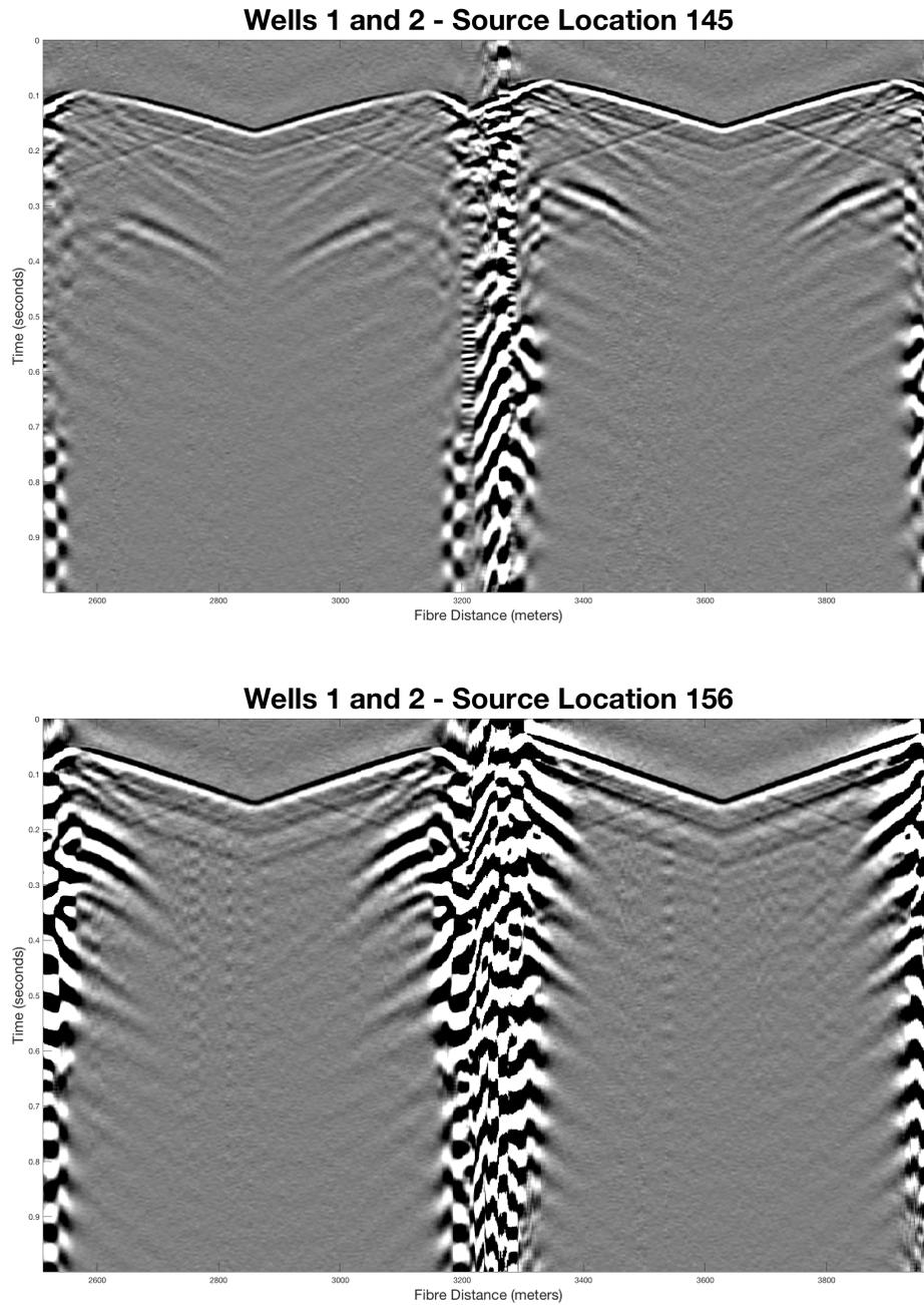
FIG. 6. The straight-fibre from well 1 to the straight fibre in well 2 acquired when the vibroseis truck was at source locations 145 (top) and 156 (bottom)
