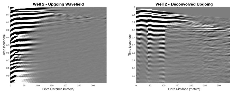
FIG. 17. (Left) The upgoing wavefield for Well 2. (Right) The deconvolved upgoing wavefield for Well 2.
