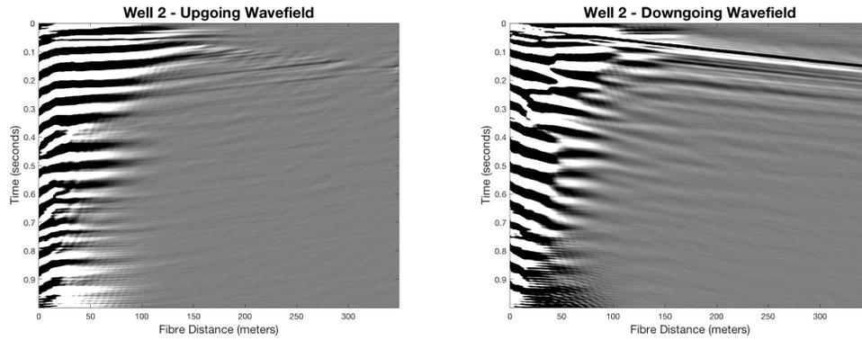
FIG. 15. (Left) The upgoing wavefield for Well 2. (Right) The downgoing wavefield for Well 2.
