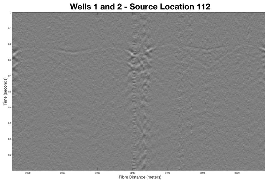
FIG. 4. The straight-fibre from well 1 to the straight fibre in well 2 acquired when the vibroseis truck was at source locations 101 (top) and 112 (bottom)
