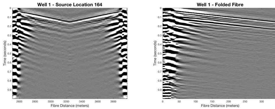
FIG. 10. (Left) Well 1 when the vibroseis truck is at Source Location 164. (Right) The straight fibre in Well 1 folded.
