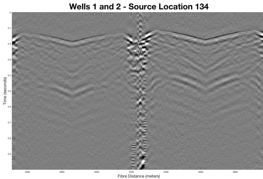
FIG. 5. The straight-fibre from well 1 to the straight fibre in well 2 acquired when the vibroseis truck was at source locations 123 (top) and 134 (bottom)
