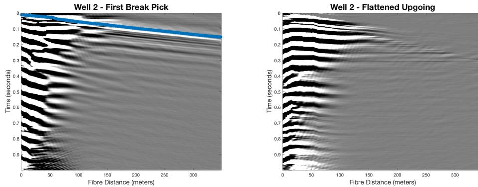
FIG. 16. (Left) The first-break picks for Well 2 at source location 158. (Right) The flattened upgoing wavefield for Well 2.
