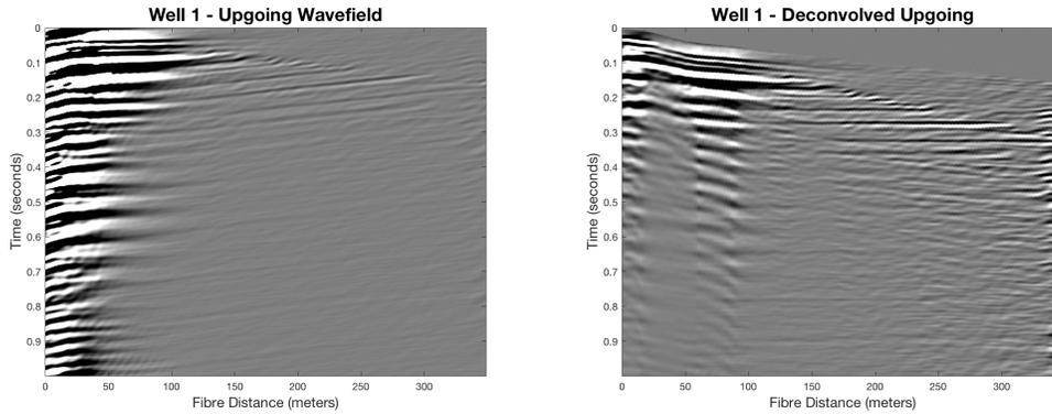
FIG. 13. (Left) The upgoing wavefield for Well 1. (Right) The deconvolved upgoing wavefield for Well 1.
