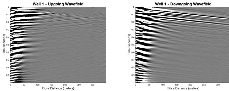
FIG. 11. (Left) The upgoing wavefield for Well 1. (Right) The downgoing wavefield for Well 1.
