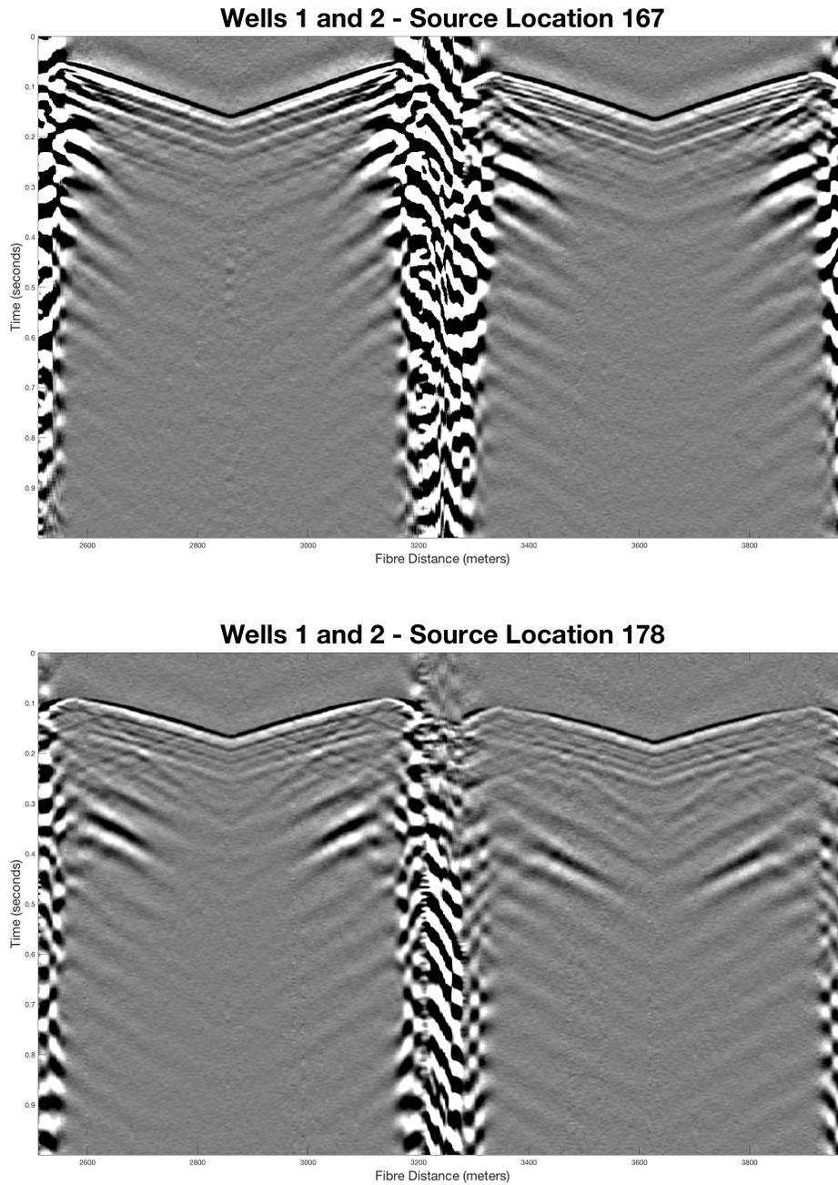
FIG. 7. The straight-fibre from well 1 to the straight fibre in well 2 acquired when the vibroseis truck was at source locations 167 (top) and 178 (bottom)
