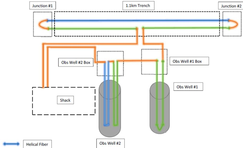
FIG. 2. A schematic of the fibre at the site in Newell County, AB.
