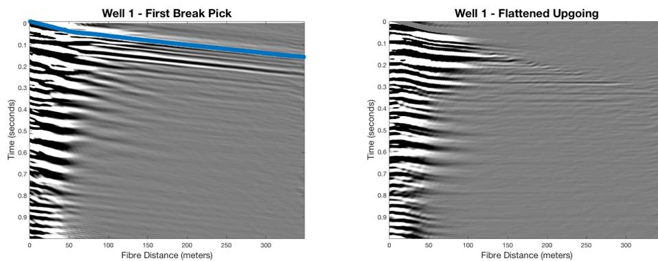
FIG. 12. (Left) The first-break picks for Well 1 at source location 164. (Right) The flattened upgoing wavefield for Well 1.
