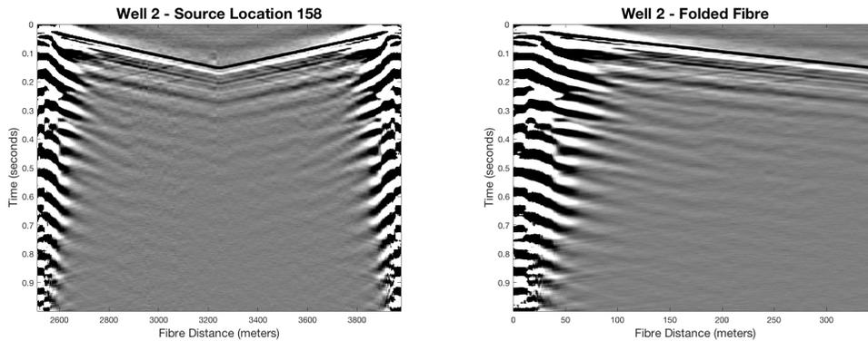
FIG. 14. (Left) Well 2 when the Vibroseis truck is at Source Location 158. (Right) The straight fibre in Well 2 folded.
