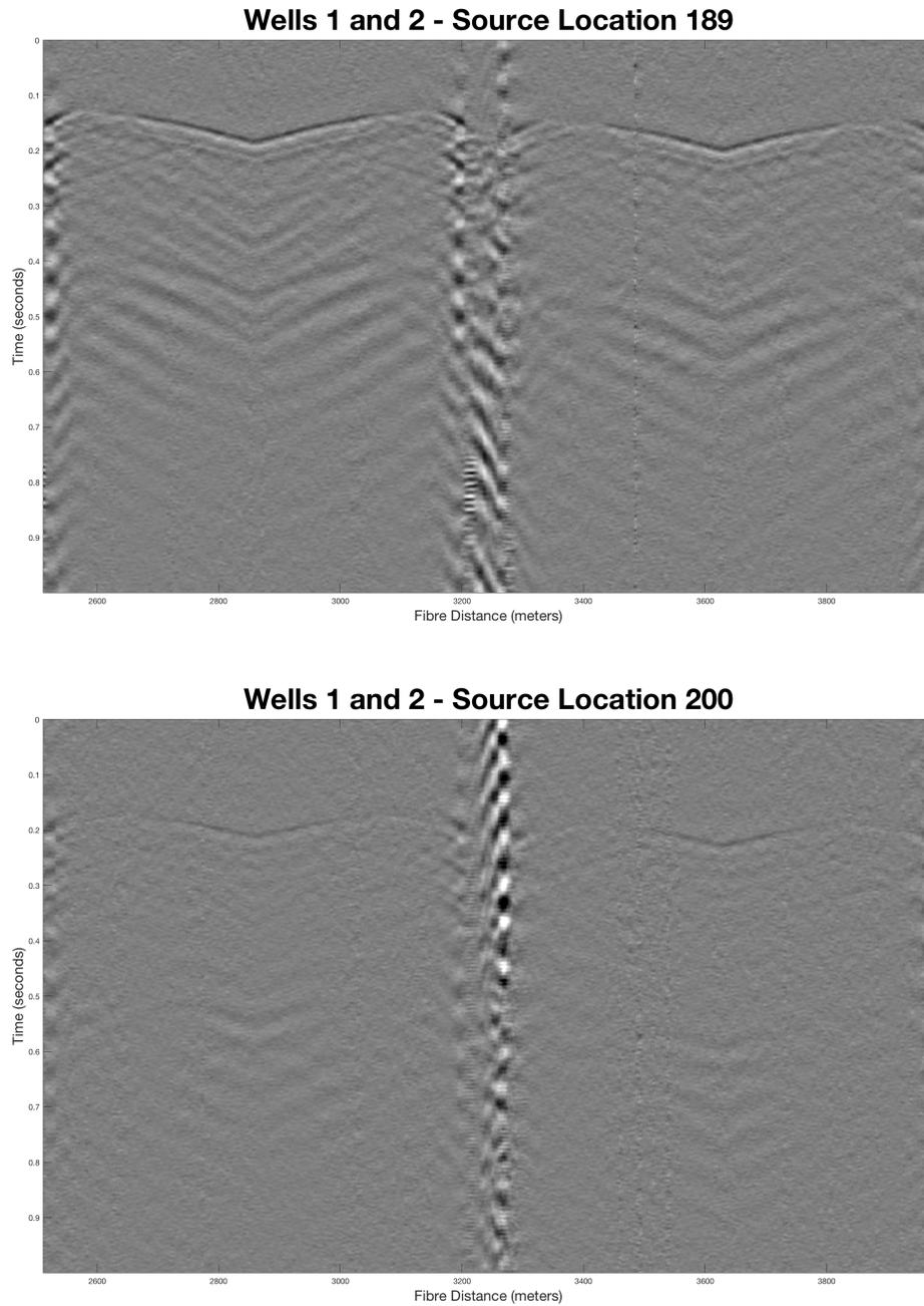
FIG. 8. The straight-fibre from well 1 to the straight fibre in well 2 acquired when the vibroseis truck was at source locations 189 (top) and 200 (bottom)
