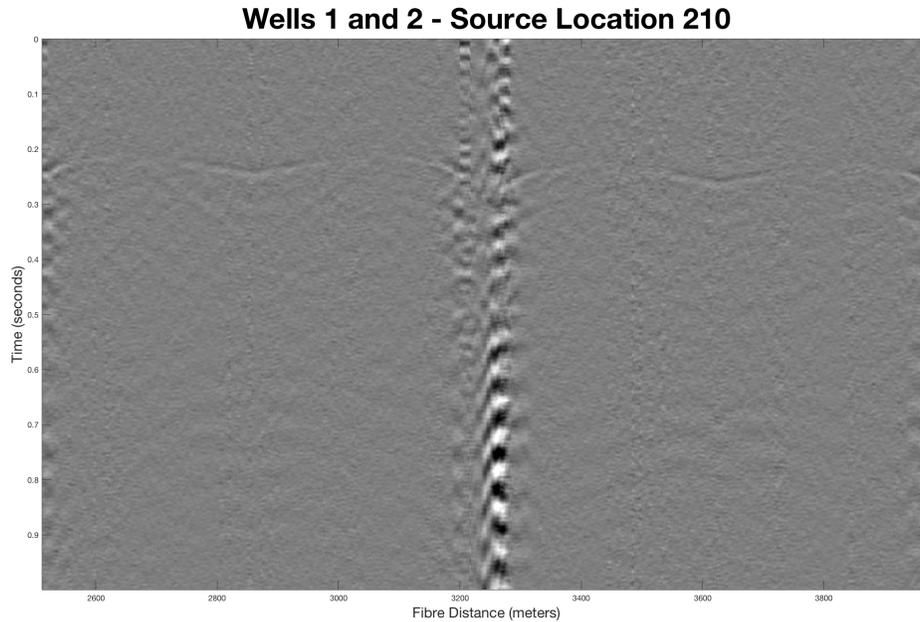
FIG. 9. The straight-fibre from well 1 to the straight fibre in well 2 acquired when the vibroseis truck was at source location 210.
