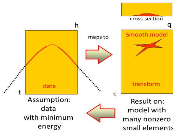
FIG. 3. Standard transforms principle:  $l_2$  norm inversion.
