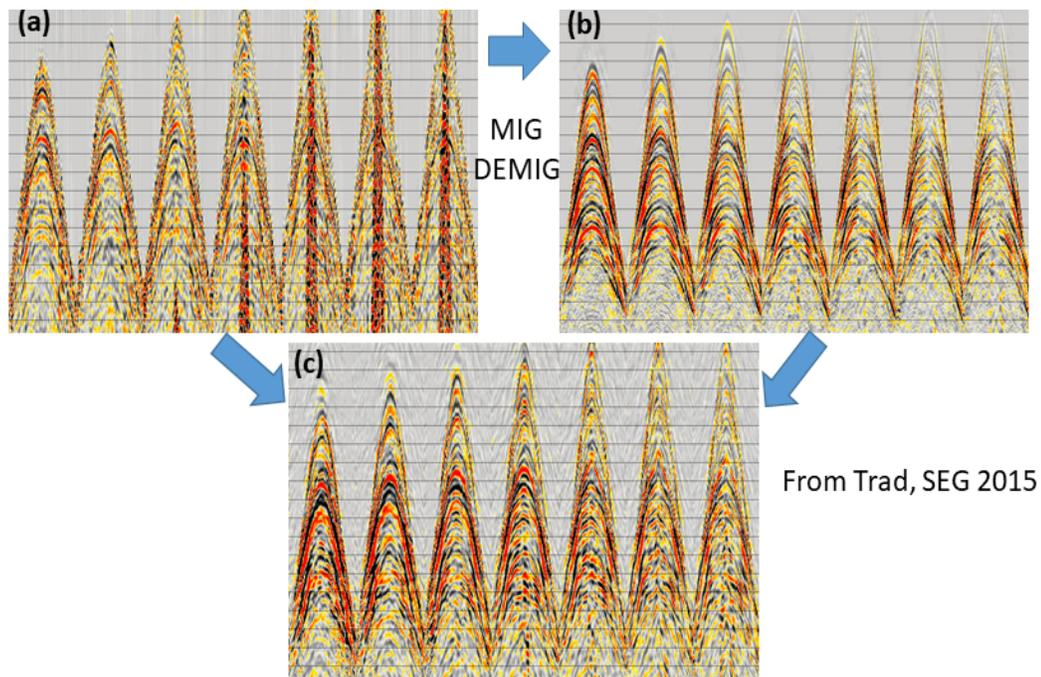
FIG. 13. a) Raw real shots before noise attenuation, b) predicted shots, c) denoised shots obtained by using predictions in b) as an inversion guided for 5D (from Trad (2015))
