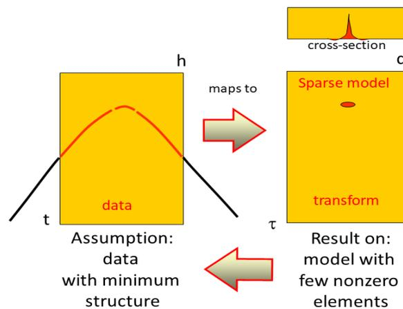
FIG. 4. Sparse transforms principle:  $l_1$  norm inversion.
