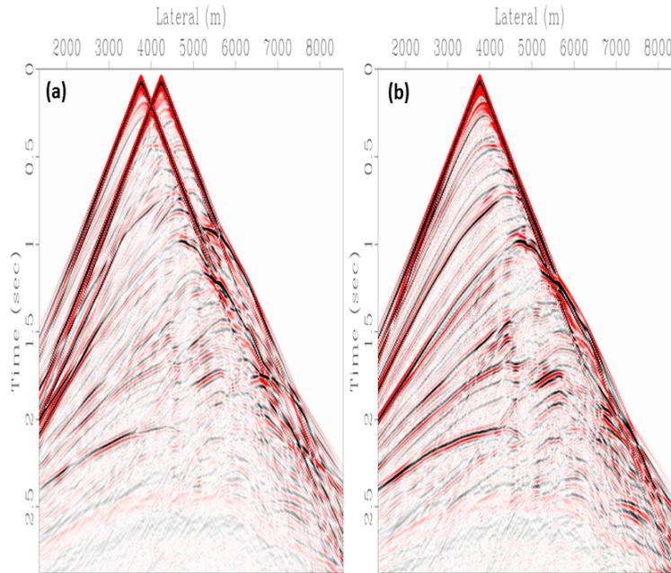
FIG. 7. a) A blended shot produced by finite differences, b) One of the shots predicted by RTM migration/demigration
