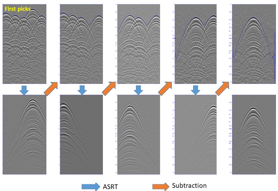
FIG. 9. A five-shot gather deblended by an Apex Shifted Radon Transform sequence
