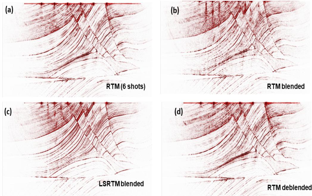
FIG. 10. a) RTM for 6 individual shots, b) RTM for 6 shots blended in groups of 3 (2 blended shots), c) LSRTM for the same 6 shots (groups of 3) with 5 iterations (migration cost of LSRTM for 2 individual shots), d) RTM for deblended shots from b) by migration/demigration of 2 shots with groups of 3).
