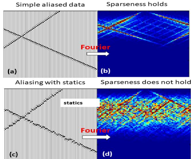
FIG. 6. a) Linear events map to well defined Fourier components in b), where standard techniques for sparse inversion would work very well, even if there is aliasing. c) Static shifts, as commonly presented in raw data, map to mixed Fourier coefficients in d) where sparse inversion would not work.
