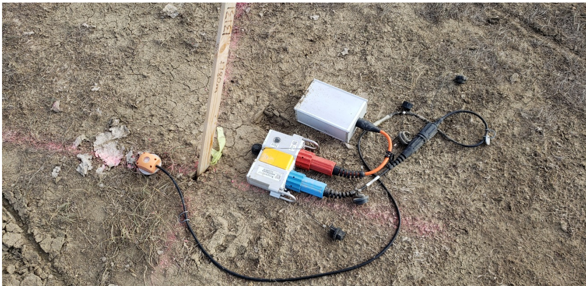
FIG. 3. A Hawk node, geophone and battery recording.
