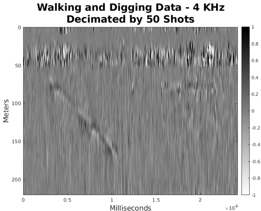
FIG. 10: The 4kHz PRF walking and digging data set decimated by 50 shots. The walking events are located between 50 and 175 meters and 0.25 \times 10^4 and 1.1 \times 10^4 milliseconds. The digging events reside between 50 and 100 meters and 1.5 \times 10^4 and 2.25 \times 10^4 milliseconds.
