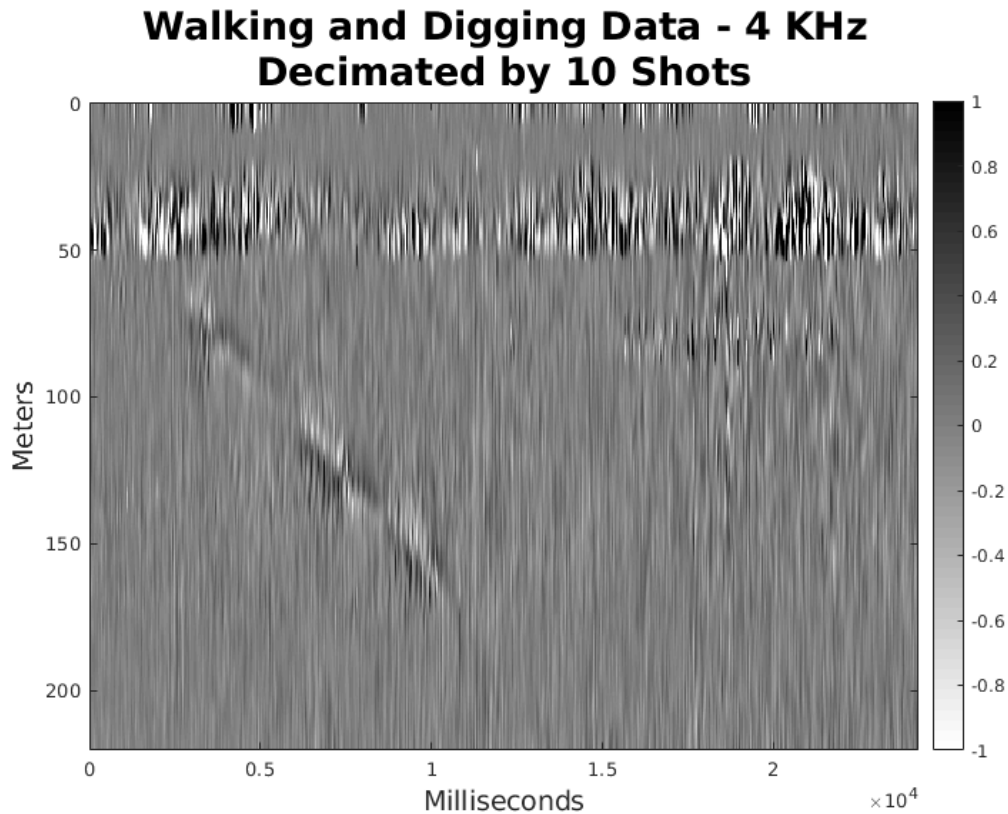
FIG. 8: The 4kHz PRF walking and digging data set decimated by 10 shots. The walking events are located between 50 and 175 meters and 0.25 \times 10^4 and 1.1 \times 10^4 milliseconds. The digging events reside between 50 and 100 meters and 1.5 \times 10^4 and 2.25 \times 10^4 milliseconds.
