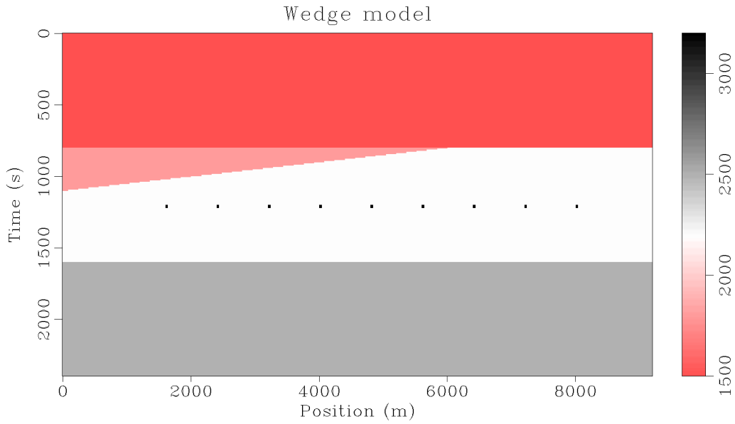
FIG. 7. Wedge model: Model consisting of two layers, a dipping reflector(wedge), and a set of diffraction points.
