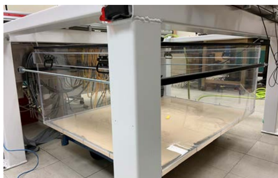
FIG. 1. Top: AWG showing Raspberry Pi 4B to the left and DAC circuitry to the right. Bottom: New acrylic water tank...
