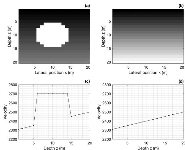
FIG. 2. A small (20x20 cell) model is adopted as a backdrop for numerical testing. (a) The geology is a linearly increasing P-wave velocity interrupted by a high velocity zone; (b) the background linear velocity is adopted as the initial model. In (c)-(d) profiles are extracted from the centre to enable more precise monitoring of the FWI convergence.
