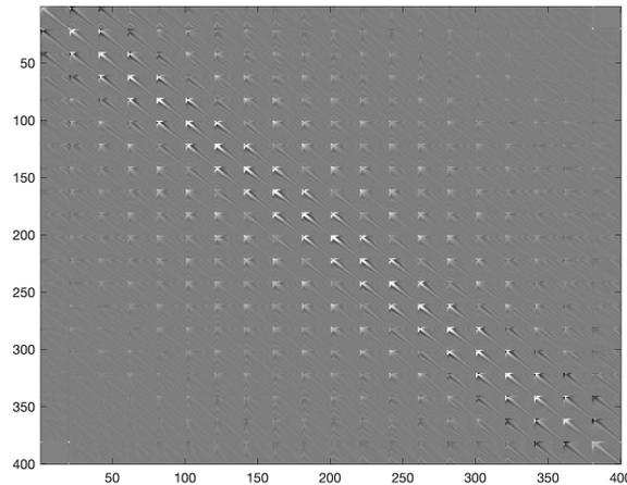
FIG. 4. The Hessian matrix calculated during the 10th iteration of the benchmark steepest descent optimization illustrated in Figure 3.
