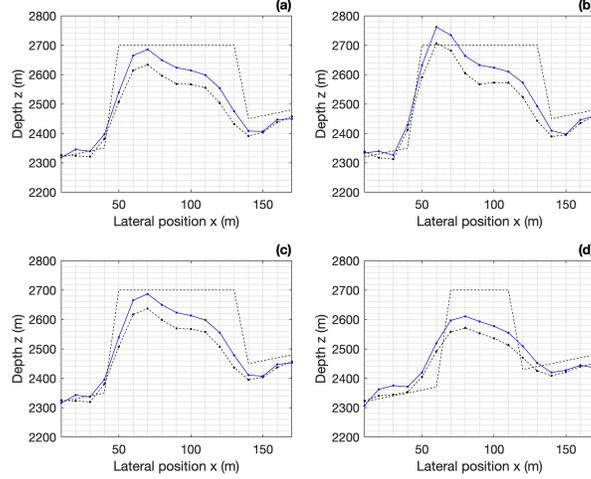
FIG. 9. (a-d) Various vertical profiles through the final results, through basic steepest descent (black) and through transformed steepest descent (blue).
