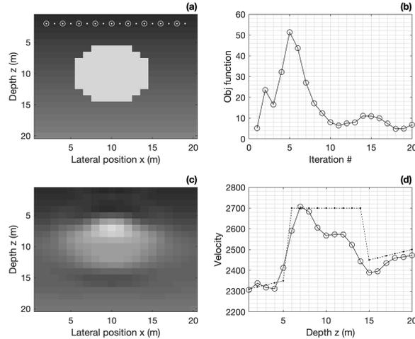
FIG. 3. Benchmark steepest-descent optimization example. (a) The true model with source (circle) and receiver (dot) locations; (b) data misfit per iteration; (c) final results after 20 iterations; (d) profile of actual result versus steepest descent result.
