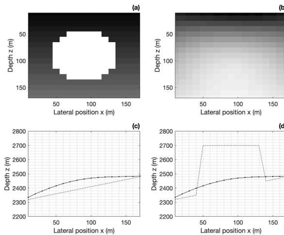
FIG. 6. Steepest descent optimization is carried out to iteration 4 and paused. (a) Actual simulated geological model; (b) updated model in image form at 4th iteration; (c) central profile of updated model plotted against initial model; (d) central profile of updated model plotted against actual model.
