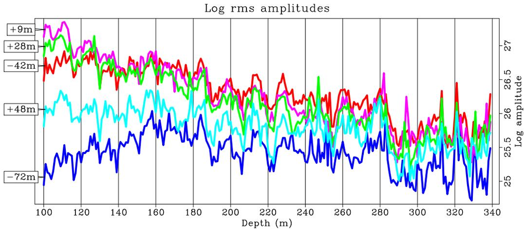
FIG. 3. Logarithms of the RMS amplitudes of the DAS VSP shot gathers in Figure 2.
