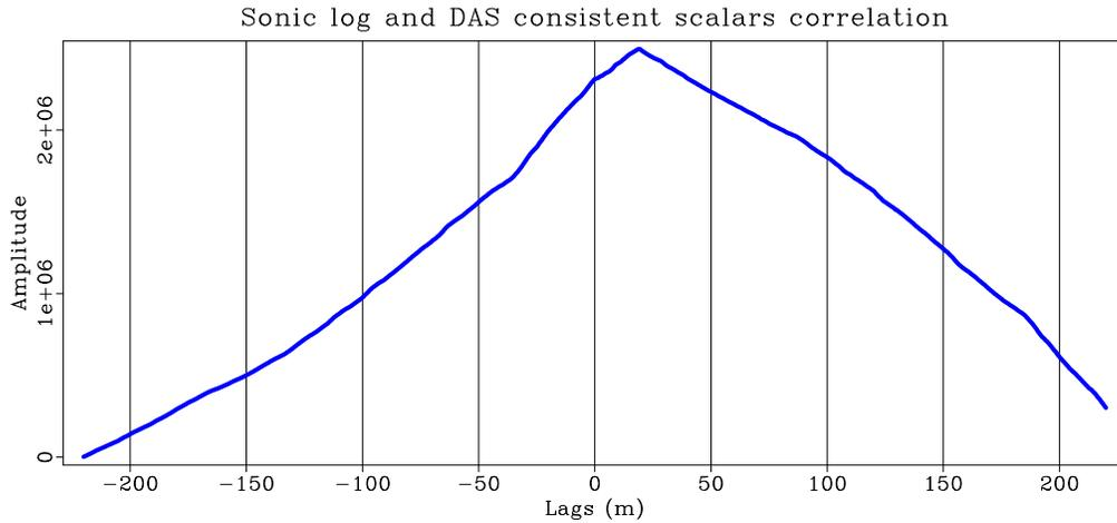
FIG. 5. Cross-correlation of the consistent scalars and the sonic log of Figure 4. The maximum value occurs at 19.5m.
