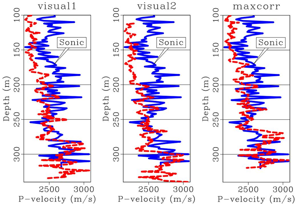
FIG. 6. Three different vertical shifts of the consistent scalars, in dashed lines, with respect to the sonic log. On the left, the vertical shift is 4.5m upward to line up the three peaks in "zone 1" of Figure 4. On the centre, the shift is 12m downward to align the two peaks in "zone 1" of Figure 4. On the right, the shift is 19.5m upward, obtained from the lag of the cross-correlation maximum between the consistent scalars and the sonic log.
