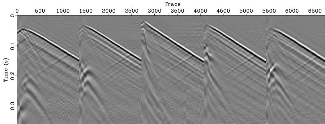
FIG. 2. DAS VSP shot gathers used for the consistent scalars calculation. Their shot numbers, from left to right are 21124, 21127, 21132, 21134 and 21136. Above, from left to right, their distances to the well are  $-72\text{m}$ ,  $-42\text{m}$ ,  $9\text{m}$ ,  $28\text{m}$  and  $48\text{m}$ . The negative offsets are located North of the well and the positive at the South.
