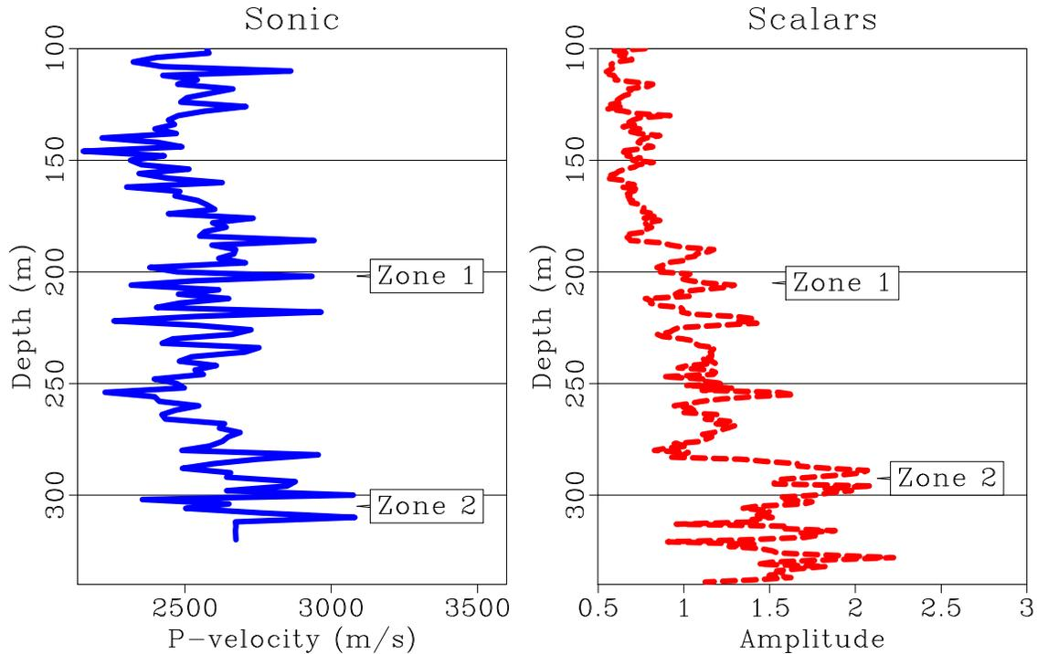
FIG. 4. The left part is the sonic log in the well containing the DAS. The right part are the consistent scalars obtained by inverting the system in Equation 4, multiplying by  $-1$  and being used as argument of the exponential function.
