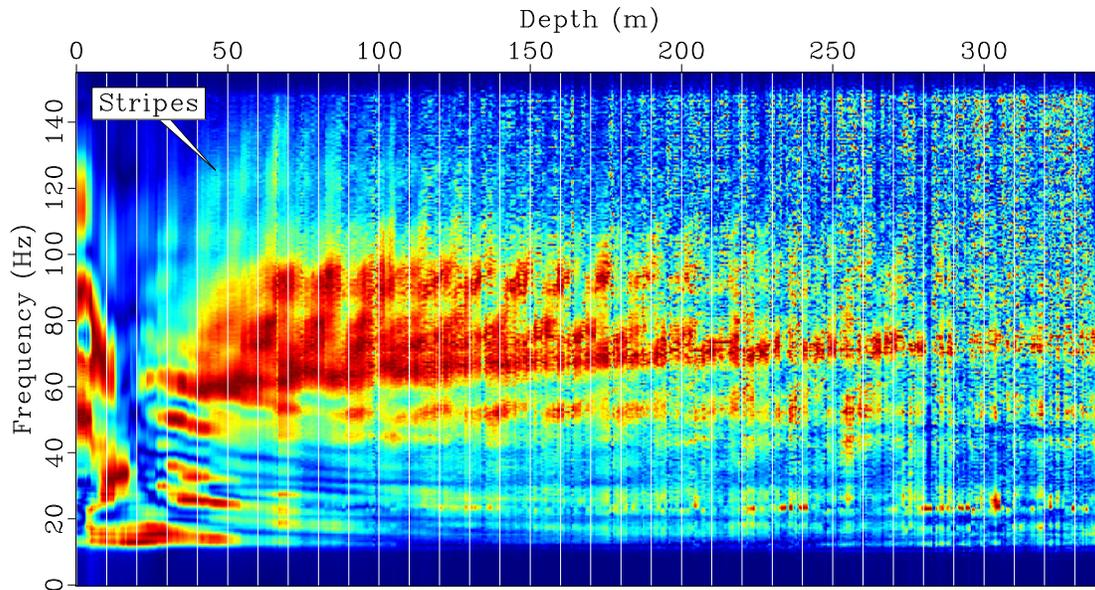
FIG. 1. Normalized frequency spectrum of the DAS VSP shot gather 21132, the closest, just 9m, from the well. The depth axis is the original depth calibration. Some stripes can be seen in the top left part.
