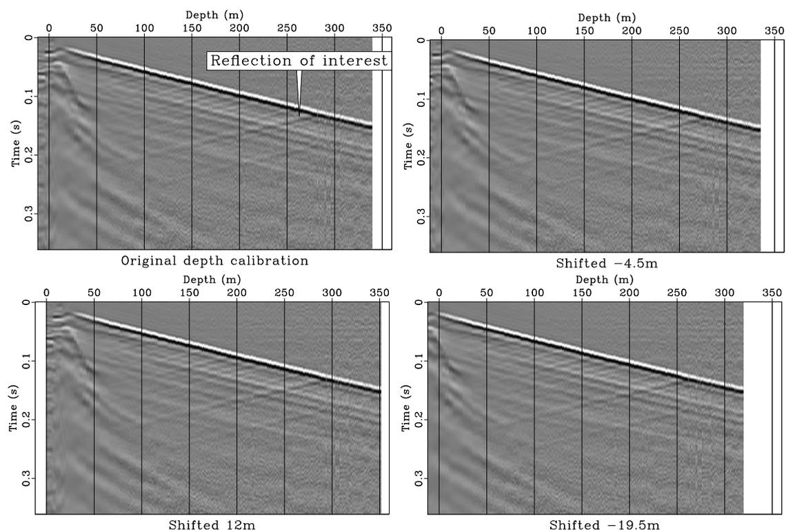
FIG. 7. DAS VSP shot gather 132 at 9m from the well. Top left is the original depth calibration. Top right is after moving the shot upwards 4.5m. Bottom left is after moving it downwards 12m. Bottom right is after moving it upwards 19.5m. The reflector of interest is marked on the original gather. This reflector corresponds to the top of the CO<sub>2</sub> injection zone.
