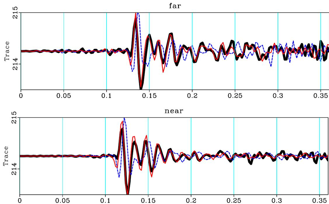
FIG. 6. Trace comparison from the original and inverted gathers of Figure 5. Above is from the far gathers and below from the near ones. Continuous thick black line is the original DAS trace, continuous thin red one is the predicted DAS trace. Dashed blue line is the predicted geophone trace in the latent space.
