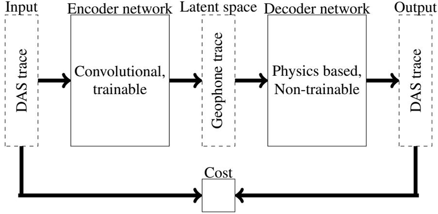
FIG. 2. DAS to geophone encoder-decoder neural network. The input and output is the DAS trace and the whole network acts like an identity operator. The encoder part is a CNN that transforms DAS to geophone, the latent space. The decoder part is non trainable and physics based that transforms geophone to DAS.
