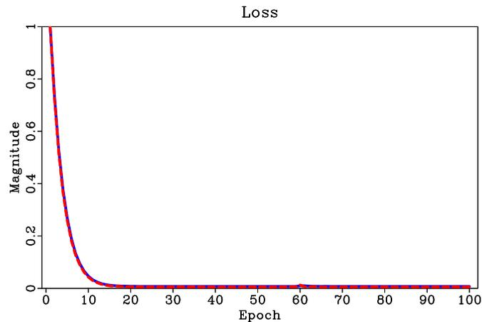
FIG. 4. Encode-decoder CNN network training loss (continuous line) and validation loss (dashed line) functions. The loss function is mean squared error.
