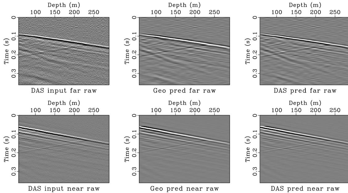
FIG. 5. Far, above, and near, below, gathers. Left column are the input DAS gathers, the middle column contains the predicted geophone gathers (in the latent space), and the right column are the predicted DAS gathers.
