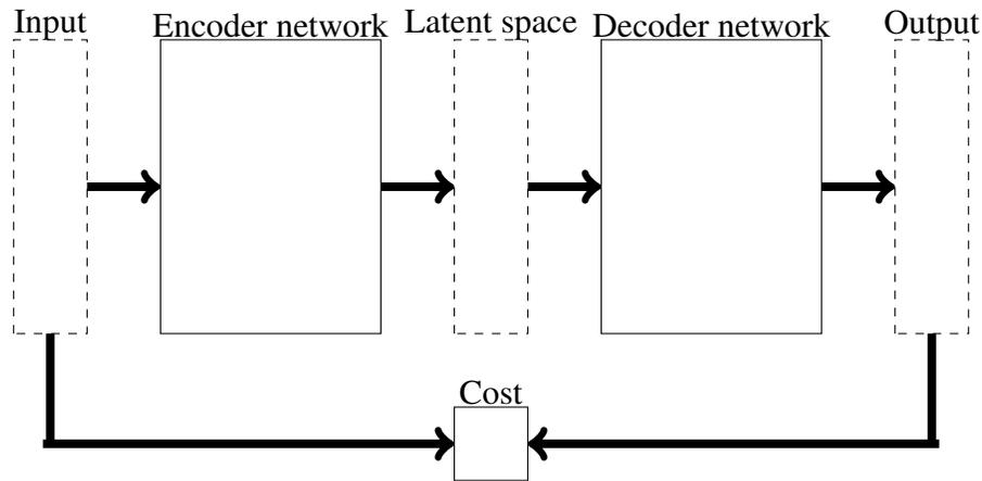
FIG. 1. Basic encoder-decoder network architecture. The network trains by optimizing the difference between input and output. The latent space is configured depending on the application.
