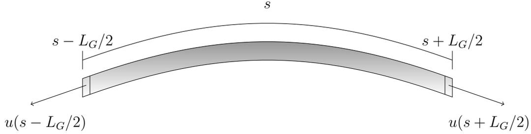
FIG. 3. A portion of optical fibre of gauge length  $L_G$  centred at  $s$ . The total elongation or contraction of this portion of fibre is the difference of the displacements at their ends (From Monsegny et al. (2021)).
