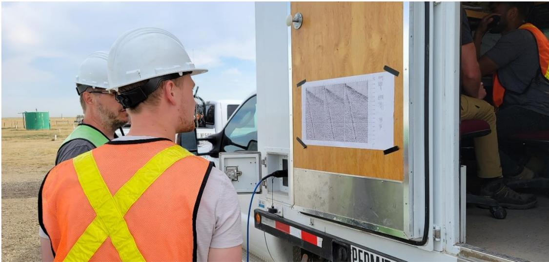
FIG. 5. A field school student discussing the raw seismic record recently acquired. The vertical components are displayed on the of the paper taped to the door. The first breaks, air blast, and a reflection can all be seen in this image.
