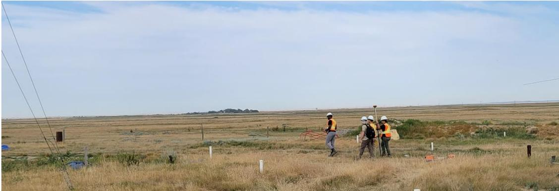
FIG. 3. Students using the differential GPS to record the location of each geophone.
