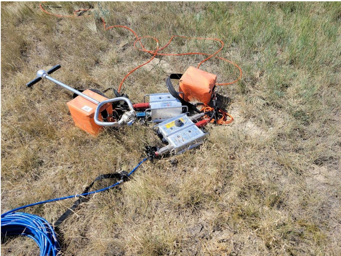
FIG. 4. A twenty four channel three component RAM and a line tap. The line tap is connected to the blue cable. Also visible are two batteries (orange boxes) and a geophone planting pole.
