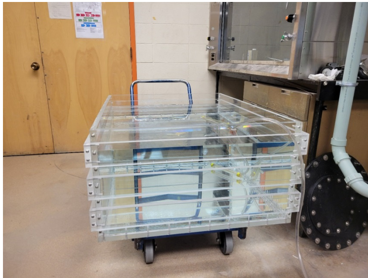
FIG. A4. The newly assembled and chemically bonded tank, after a weekend holding water near a floor drain. The tank did not leak.
