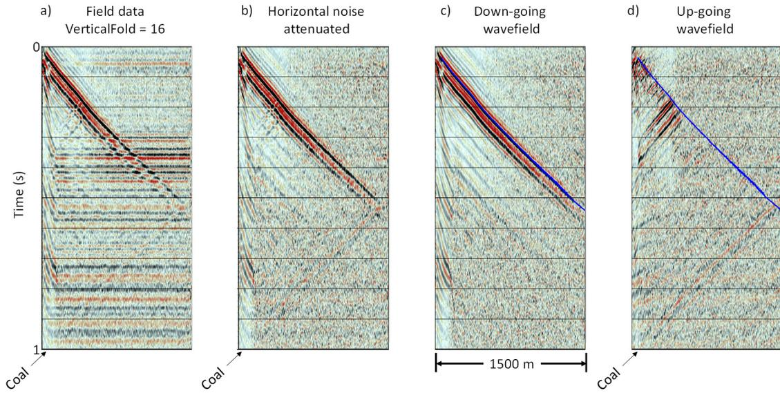
FIG. 3. March VP 2010 field data with vertical fold equal to sixteen (a), after removing horizontal noise bands using a  $f$ - $k$  filter with 8 km/s cut-offs (b), and the down-going (c) and up-going (d) wavefields separated using  $f$ - $k$  filters. Data are displayed with a 500 ms window AGC.
