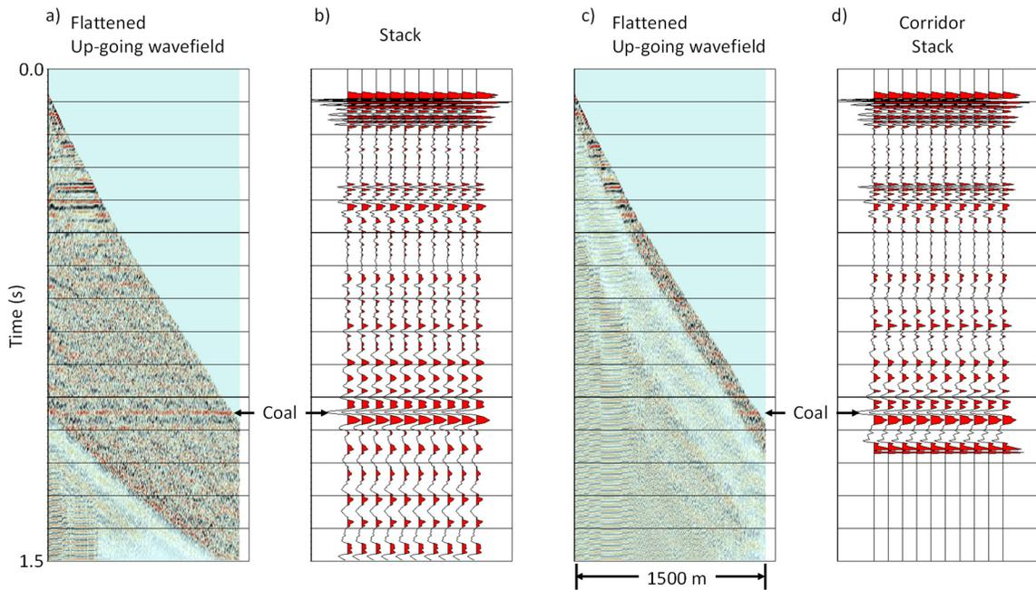
FIG. 4. March VP 2010 field data with vertical fold equal to sixteen after flattening on first-break picks (a) and stacking (b), and after applying a bottom mute (c) and corridor stacking (d). Data are displayed with a 500 ms window AGC. The stacked trace(s) have been repeated ten times for visibility (b and d).
