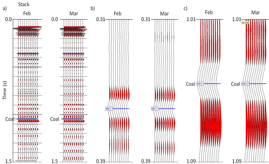
FIG. 6. February (vertical fold = 8) and March (vertical fold = 16) stack comparison (a) 0-1.5 s, (b) (0.31-0.39 s, (c) 1.01-1.09 s. The stacked trace(s) have been repeated ten times for visibility and with a 500 ms AGC.
