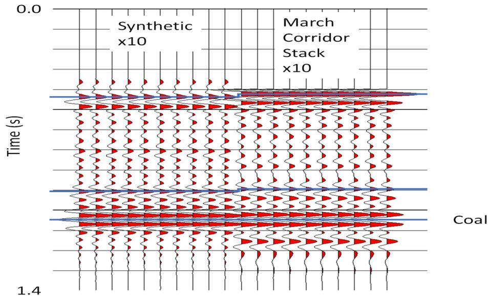
FIG. 5. Initial comparison of a synthetic seismogram (left) to the March VP 2010 corridor stack (right; Figure 4d). Data are displayed with an Ormsby 5-10-30-35 Hz filter and a 500 ms window AGC. The synthetic has been shifted to line up the trough associated with the coal but has not been stretched to better match shallower reflections. The synthetic and stacked trace(s) have been repeated ten times for visibility.
