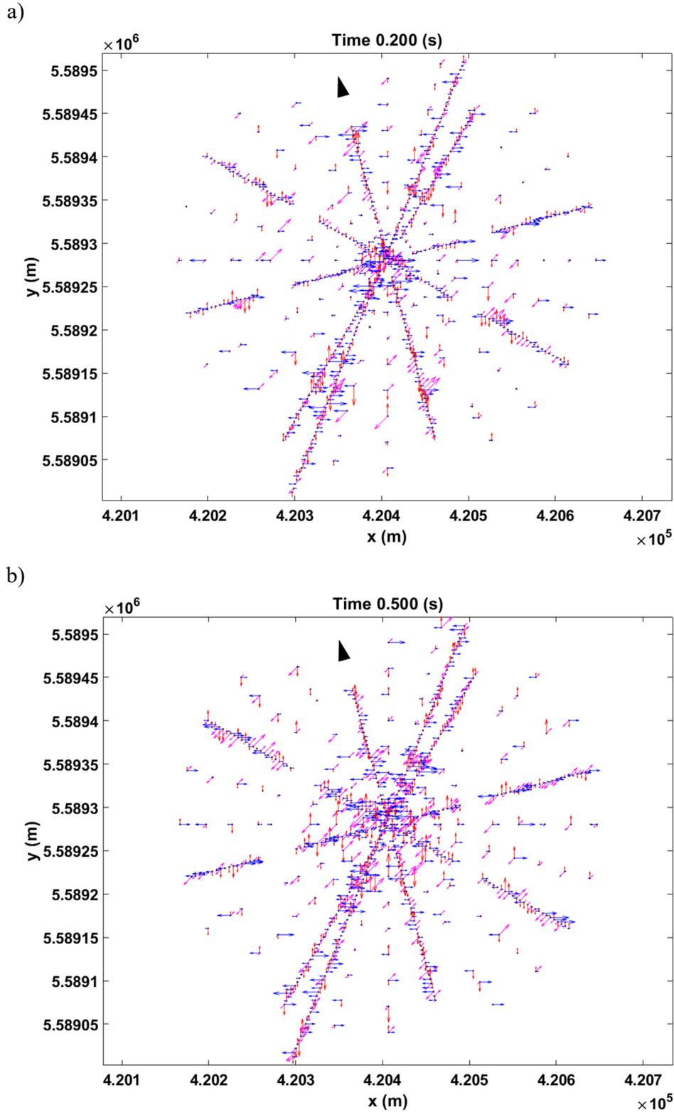
FIG. 6. Matlab quiver plot for time-slices at 0.2 s (a) and 0.5 s (b) of the directional strain traces highlighted by yellow lines in Figure 5. The base of the quivers are located at midpoint locations between each VP and the DDS. Map co-ordinates have been rotated 15 degrees counterclockwise around the DDS location for display.
