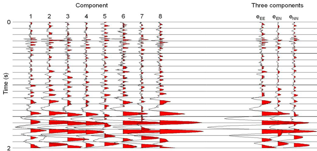
FIG. 4. VP 1101 example of reducing eight strain components to three directional components.
