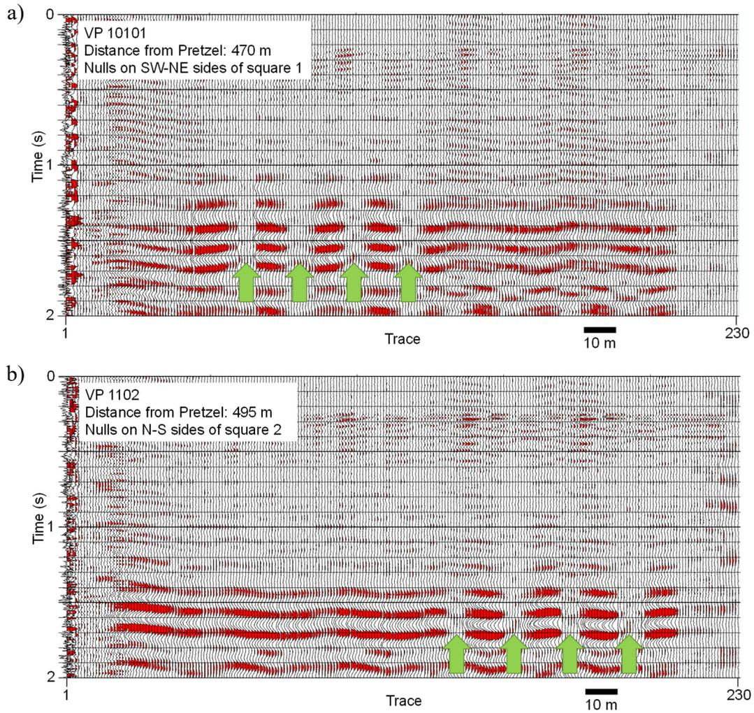
FIG. 3. Straight fiber data for VP 10101 (a) showing nulls for the two SW-NE sides of square 1 (green arrows, repeated twice) and VP 1102 (b) showing nulls for the two N-S sides of square 2.
