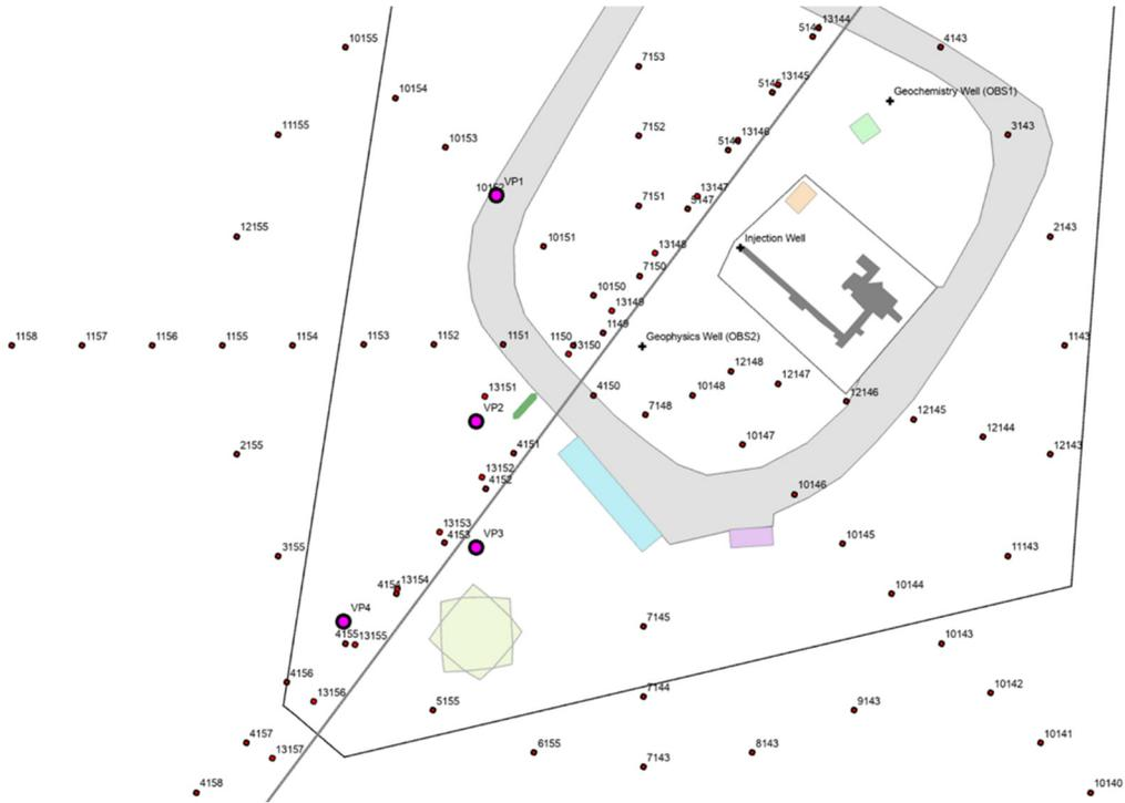
FIG. 1. Map showing the well lease with the DDS (Green), VP1-VP4 (magenta) that were acquired for initial testing of the DDS, and Snowflake2 VP (red dots) at a nominal 10 m VP spacing.
