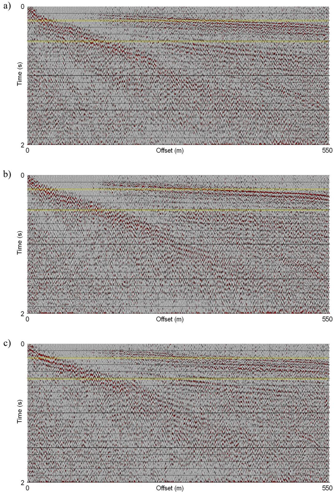
FIG. 5. Directional strain-rate receiver gathers sorted by the absolute value of source-DDS offset with AGC for display. The EE component (a), EN component (b), and NN component (c) show subtle differences at this scale. Yellow lines are shown as mapped time slices in Figure 6.
