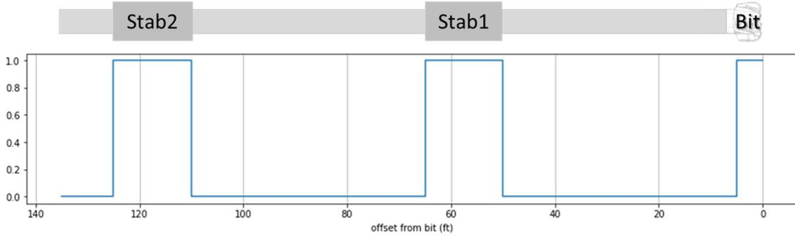
FIG. 4. The BHA source signal is created as sequence of square waves aligned with the components of the BHA that are near the same gauge as the borehole. For this example BHA, there are 2 stabilizers, denoted as Stab1 and Stab2, and the drill bit (denoted in the BHA schematic at the top) used to create the BHA source signal.
