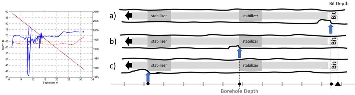
FIG. 2. The average HL versus bit position plot on the left from Freithofnig et al. exhibits an anomalous HL (blue line) associated with a dysfunction. Three example schematics of a drill string tripping out of the hole in the direction of the black arrow to the left demonstrate how dysfunctions at varying depths such as a) the bit, b) the first stabilizer, or c) the second stabilizer would be measured at the same bit depth reference (denoted by the triangle).
