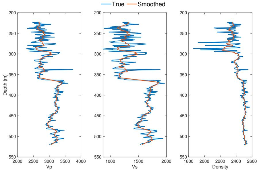
FIG. 5. Filtered velocity and density logs used as input data for the rock physics inversion.
