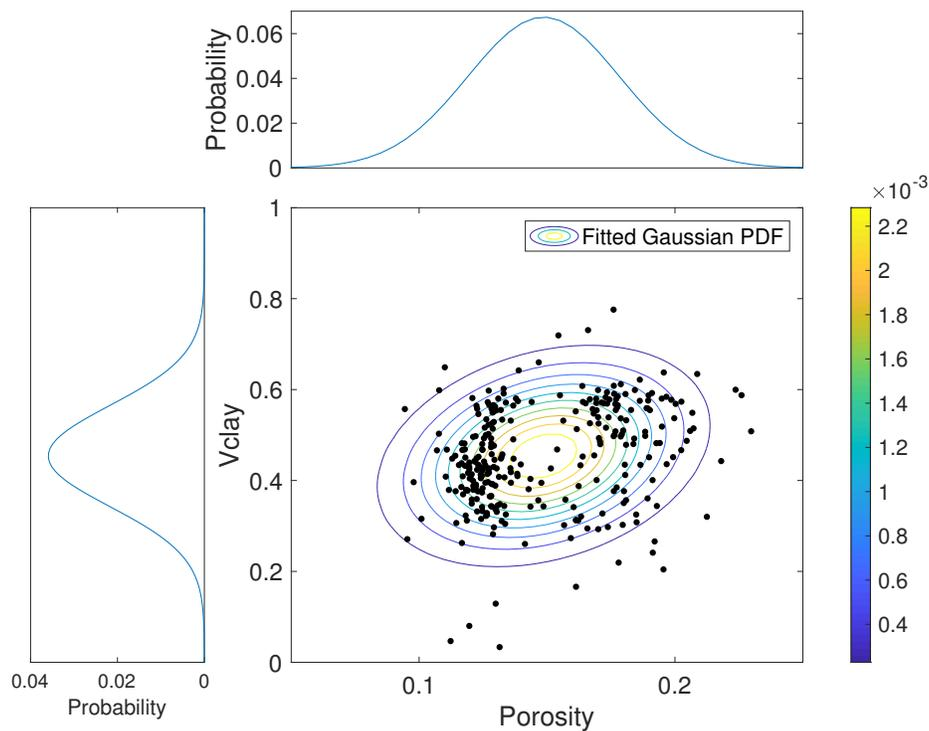
FIG. 2. Prior distribution of rock physics variables: Gaussian case. The curves represent the 2D joint distribution of porosity and clay content with associated 1D marginal distribution, obtained by fitting the well-log data (black dots).
