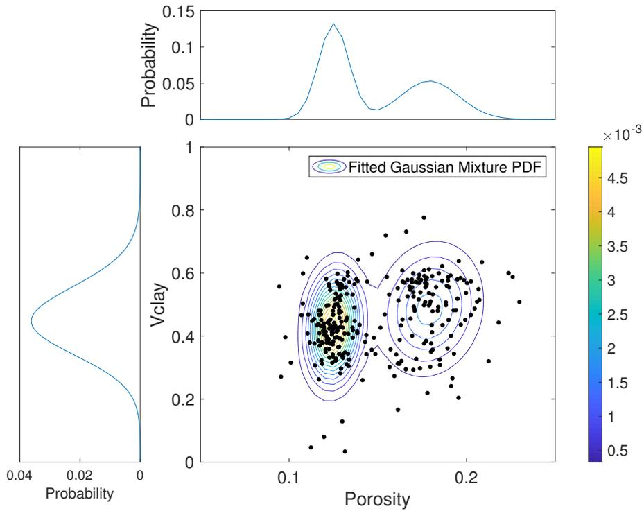
FIG. 3. Prior distribution of rock physics variables: Gaussian mixture case. The parameters of the Gaussian mixture model is obtained from the facies classification of the well-log data
