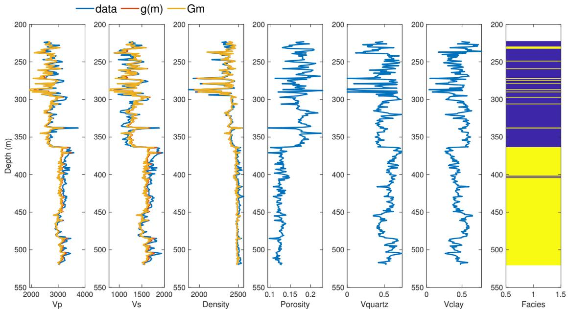
FIG. 1. Well-log data of the Countess 10-22 well at the CMC Newell County Facility. From left to right: P-wave velocity, S-wave velocity, density, porosity, and the volume fractions of quartz and clay. The blue, red, and yellow curves denote the real data, the data predicted by the nonlinear rock physics model, and the data predicted by the linearized rock physics model. The rightmost column shows the result of facies classification based on the measured data, assuming two facies.
