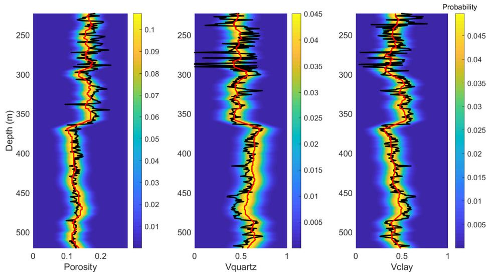
FIG. 6. Results of the Bayesian linearized rock physics inversion. The background color represents the posterior distribution and the solid red curves represent the maximum a posteriori predictions. The solid black curves represent the actual well logs.
