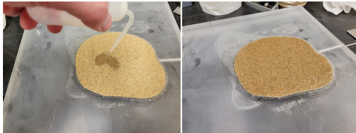
FIG. 10. Using water to determine the porosity of the glass bead blasting media.
