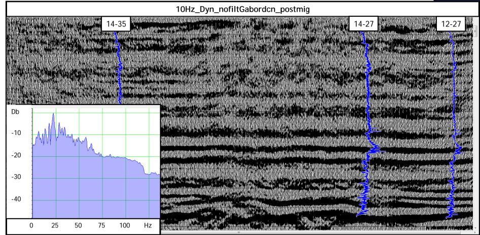
Seismic line: 2 kg of dynamite and 3C 10 Hz geophones 600-1100 ms 3 wells (Husky Energy): 14-35-25-21W4M 14-27-25-21W4M 12-27-25-21W4M
