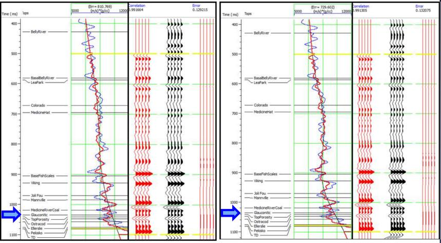
Post-stack inversion analysis for each model: Model 1-3 Hz (left) Model 2-4 Hz (right)
