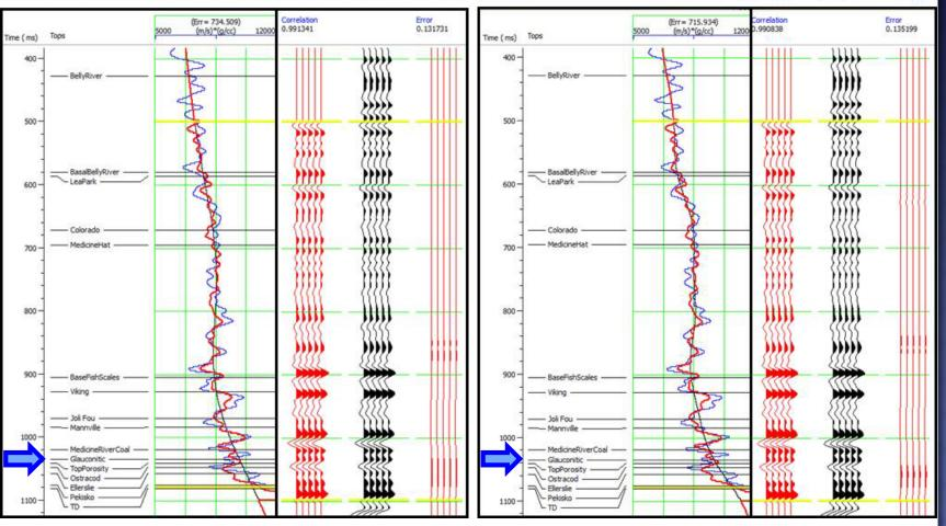
Post-stack inversion analysis for each model: Model 3-5 Hz (left) Model 4-8 Hz (right)
