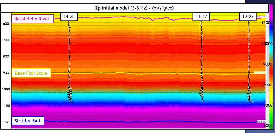
3-5 Hz modelWell 14-35-25-213 horizons: Basal Belly River, Base Fish Scale and Stettler Salt.
