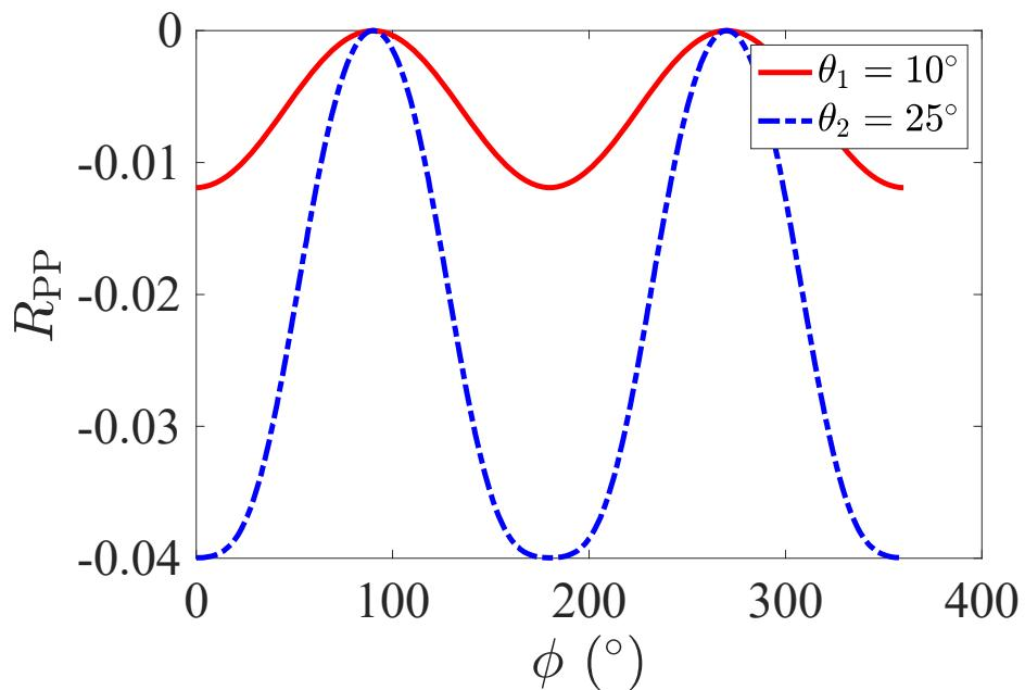
P-wave velocity variation with azimuthal angle (VVAZ)
