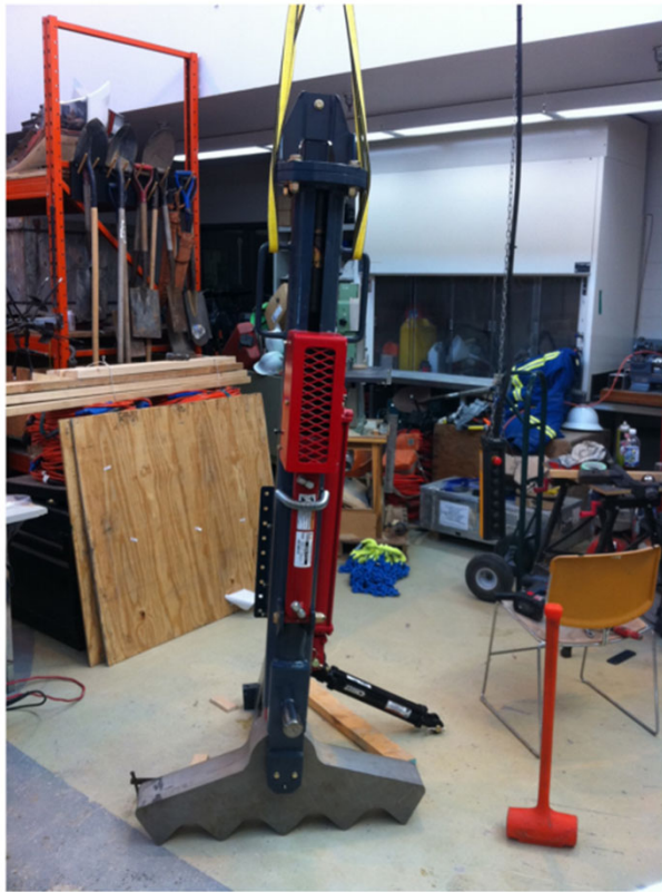
FIG. 2. The USAInc compressed nitrogen accelerated weight-drop source as delivered. Lawton et al., 2013
