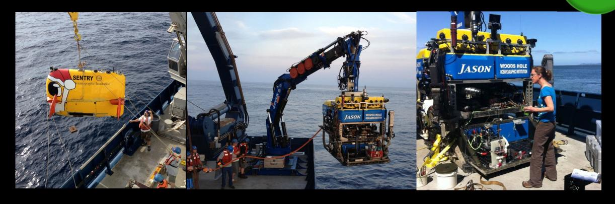
AUV Sentry used to map seafloor, measure water column data, profile sediment thickness
