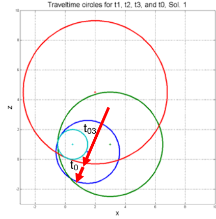
Figure 3 Three circles (red, green and blue) from the receiver locations representing t_0 = 1.0 plus the traveltime from the source to the receiver. A cyan colored circle represents the radius of v*t_0 and is tangent to the other circles.
