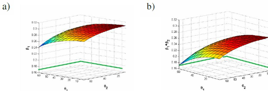
FIG. 2. Recovered parameter from the normal incidence for  $\beta$ . The exact value of  $\beta$  is 0.17. The linear approximation  $\beta_1$  (a) and the sum of linear and first non-linear  $\beta_1 + \beta_2$  (b).
