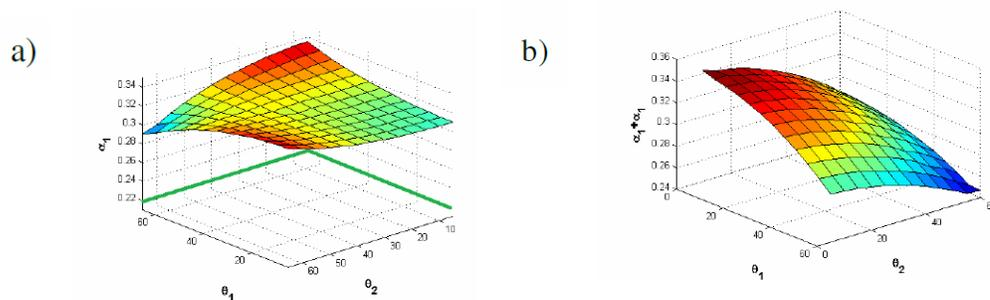
FIG. 3. Recovered parameter from the normal incidence for  $\alpha$ . The exact value of  $\alpha$  is 0.22. The linear approximation  $\alpha_1$  (a) and the sum of linear and first non-linear  $\alpha_1 + \alpha_2$  (b).
