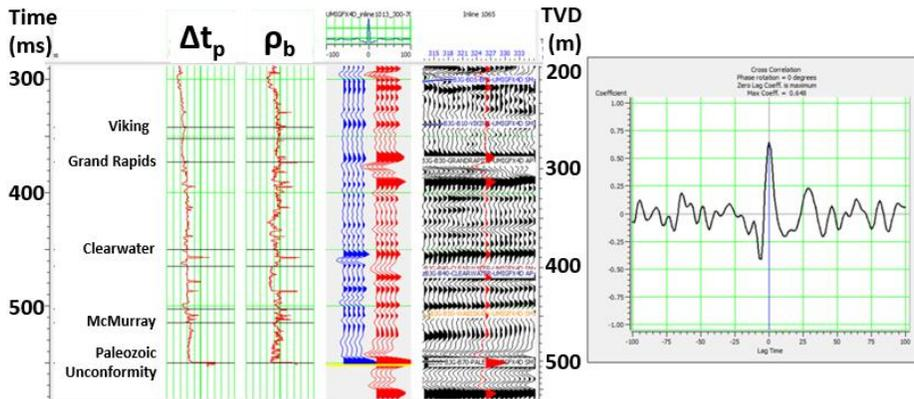
FIG 3: Example seismic to synthetic seismogram tie and associated crosscorrelation. The synthetic traces are blue and seismic traces are red.
