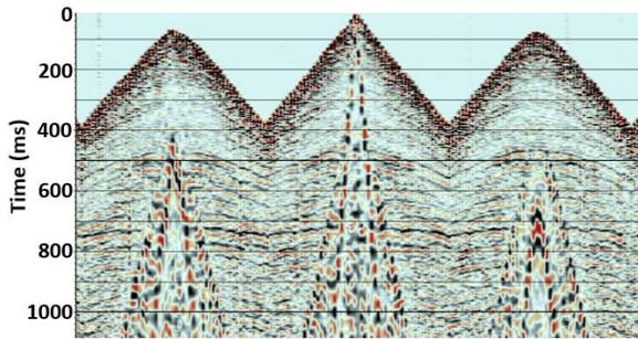
FIG 2a: Vertical geophone component raw shot record example.
