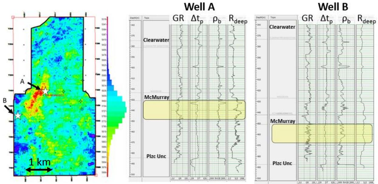
FIG. 6: Upper McMurray RMS impedance from a post-stack inversion. Impedance is higher at the location of well A than at the location of well B. Well A shows a thicker sand interval through the McMurray Formation compared to well B.
