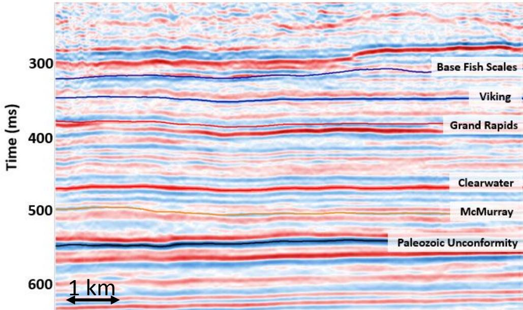
FIG. 4: Type section depicting the main geological horizons in the project area. Generally the region is not heavily structured and reflection seismic character remains quite constant regionally.
