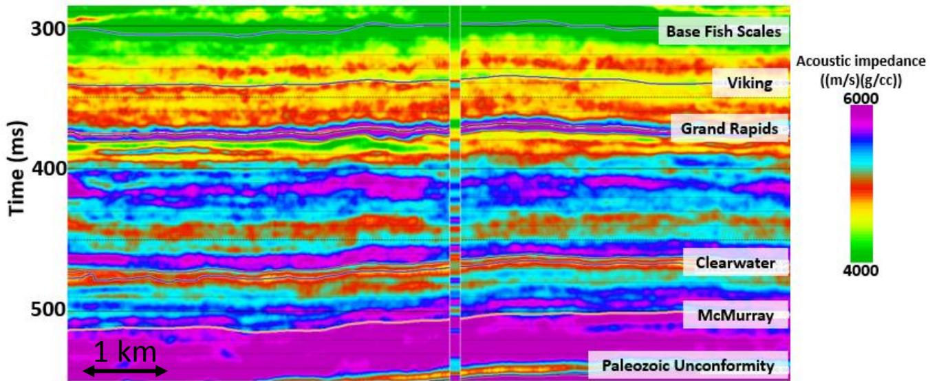
FIG 5: Post-stack impedance in-line from the inverted volume, with a blind well test. The inversion included a low frequency model based on stratigraphic interpretation and a sonic log from a well proximal to the section.
