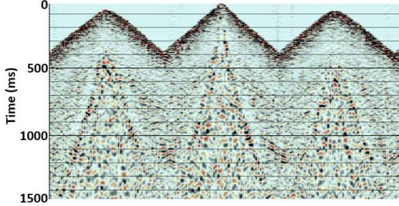
FIG 2c: Transverse geophone component raw shot record example.
