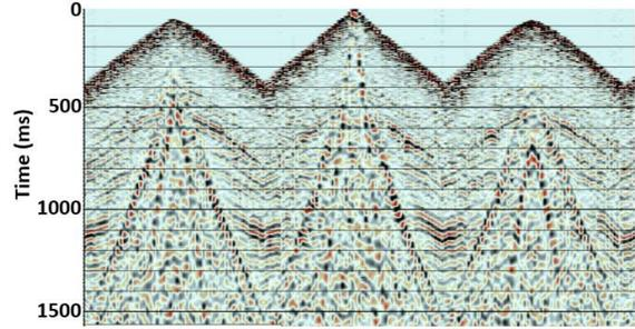
FIG 2b: Radial geophone component raw shot record example.
