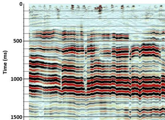
FIG. 7: Radial component receiver stack. Paleozoic Unconformity is approximately in the lowermost bright PS reflection set, ~ 1200 ms.
