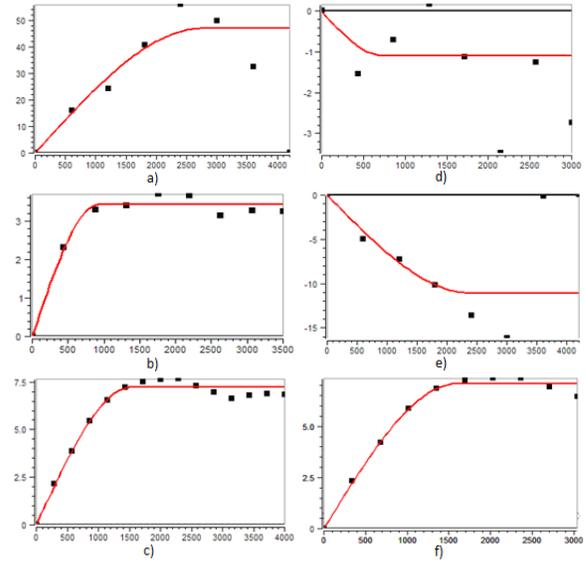
Figure 5: Variograms of the primary and two secondary variables, where a) shows the variogram of the well, b) shows the variogram of the angle stack amplitude, c) shows the variogram of the  $v_p/v_s$  ratio, d) shows the variogram of well and angle stack amplitude, e) shows the variogram of well and  $v_p/v_s$  ratio, and f) shows the variogram of angle stack amplitude and  $v_p/v_s$  ratio.
