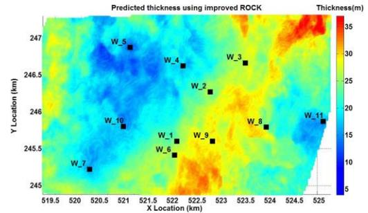
Figure 6: Predicted thickness and distribution of the reservoir formation using the improved ROCK method, obtained by considering thickness from the wells as the primary variable, and the angle stack amplitude and  $v_p/v_s$  ratio as two secondary variables.
