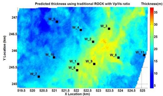
Figure 8: Predicted thickness and distribution of the reservoir formation using traditional ROCK with only one secondary variable:  $V_p/V_s$  ratio.
