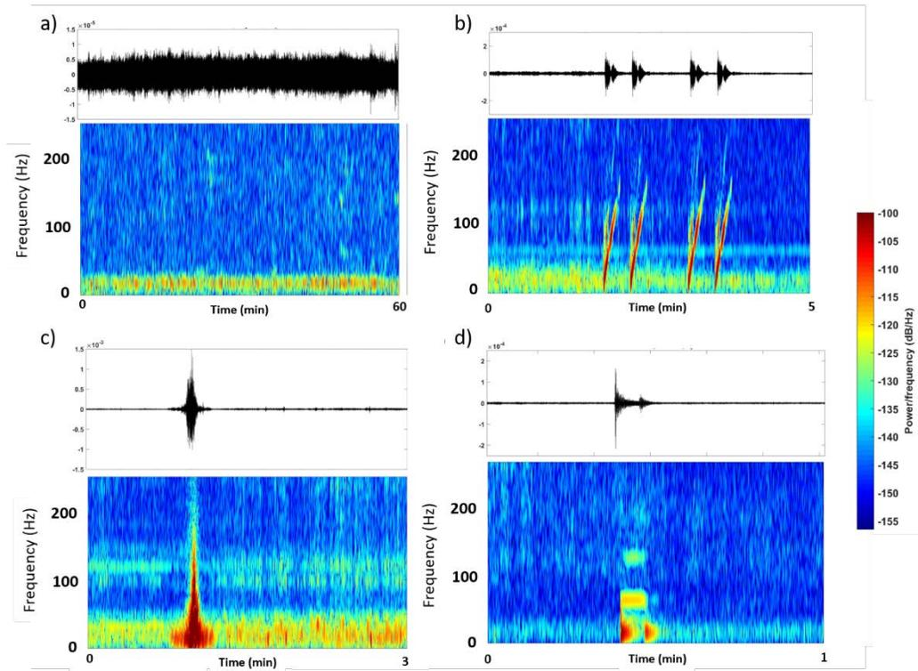
Figure 3: Example of continous seismic signal and corresponding spectrograms. a) 1hour of noise. b) 5min including 4 vibe shots. c) 3min including a pump triggering. d) 1min still-need to be determined spunctual event.
