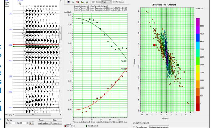
AVO modelling: synthetic angle gather (left), amplitude curves (middle), and intercept vs. gradient plot (right).
