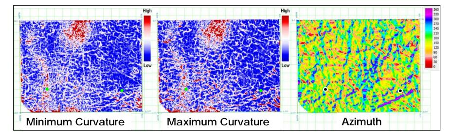
High curvature values indicate fractured zones. Azimuth map indicates that the major trends are about 0° and 40°.
