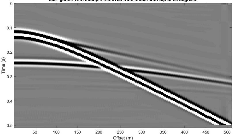
CMP gather with multiple removed from model with dip of 25 degrees.
