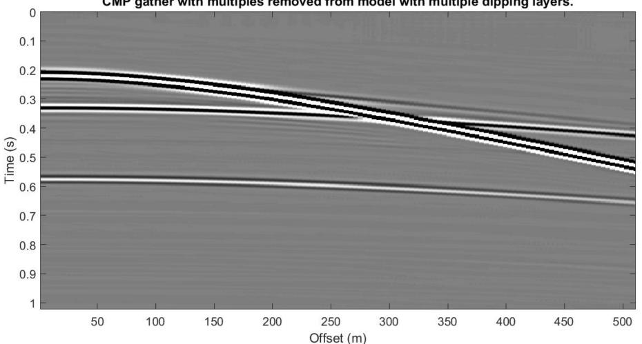
CMP gather with multiples removed from model with multiple dipping layers.
