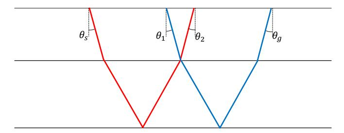
When flat layers exist in the subsurface, and  $p_g = p_s = p_1 = p_2$  the problem reduces to 1.5D, and the resulting prediction equation simplifies to:
