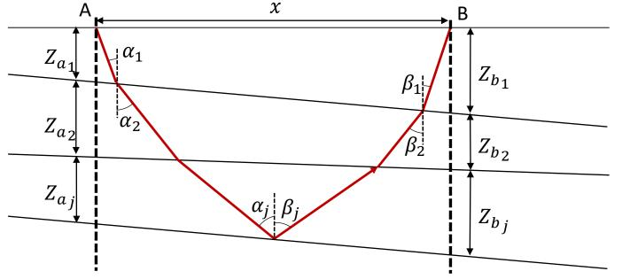
For a fixed source (or receiver) at location A, the travel time of the ray shown is:
