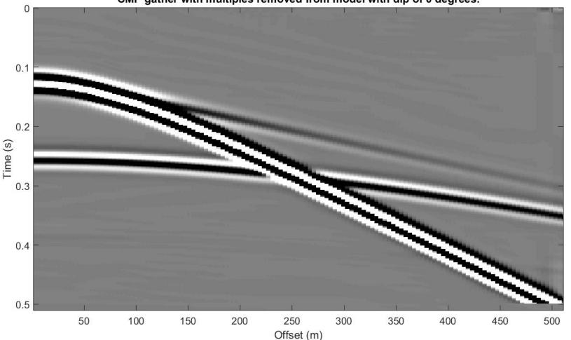
CMP gather with multiples removed from model with dip of 0 degrees.
