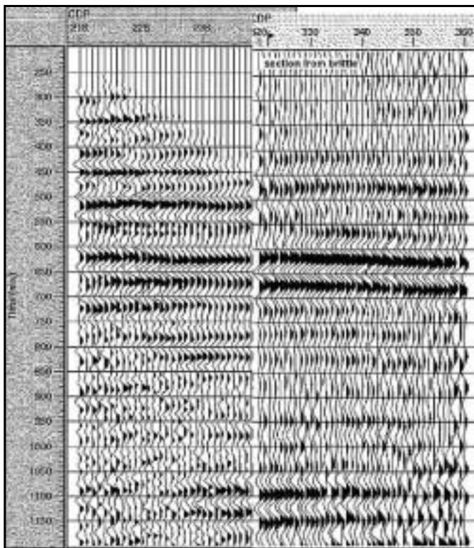
Figure 2: The lake-bottom cable stacked section (left) and low-pass filtered Winter 2000 section (right).
