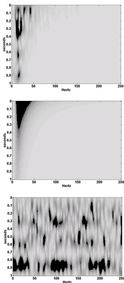
FIG. 1. The first panel shows the Gabor transform of a seismic trace. The second shows a smoothed version of the first panel. This estimated the wavelet times the attenuation function. The third shows the Gabor transform of the reflectivity. According to the nonstationary convolutional model, the first panel is the product of the second and third.
