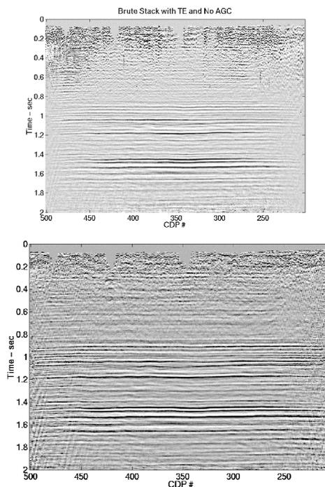
FIG. 2. CMP stacks for a Blackfoot dataset. Nonstationary deconvolution is used in the first panel, and stationary deconvolution is used in the second.
