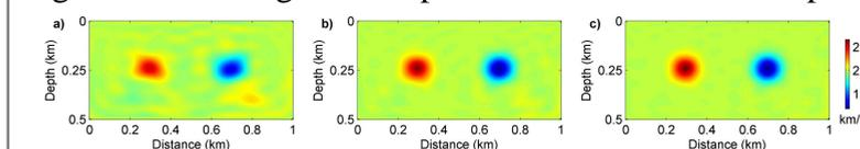
Figure 2. (a)-(c) show the inverted models using SD method, L-BFGS and Hessian-free Gauss-Newton methods respectively.
