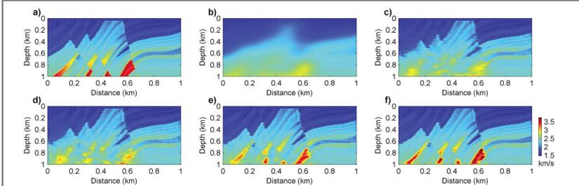
Figure 3. (a) and (b) show the true and initial models. (c), (d), (e) and (f) show the inverted models using SD, L-BFGS, non-preconditioned GN and L-BFGS preconditioned GN methods respectively.
