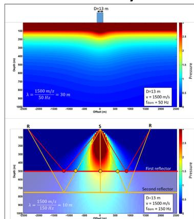
FIG. 6. Radiation pattern for source-receiver transducers for 10 and 30 m wavelengths.
