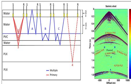
FIG. 3. Seismic shot from physical modelling. The transducers produce dominant frequencies of 500 kHz that scales down to 50 Hz.
