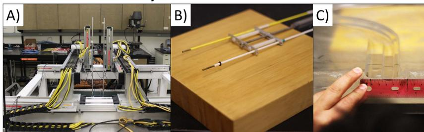
FIG. 1. A) CREWES seismic physical modelling laboratory facility. B) Transducers used as source and sensor. C) Acrylic slab (PLX) with a cut channel. Photographs by Kevin Bertram.
