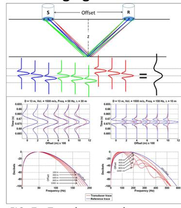
FIG. 7. Transducers work as an array of point sources and receivers, which affects the waveform with offset.
