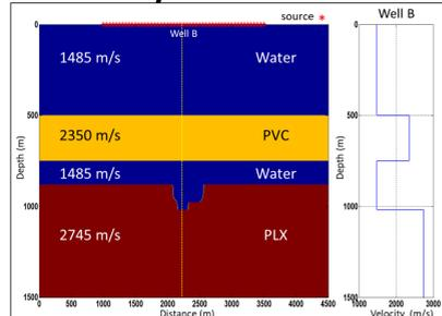
FIG. 2. Horizontal and vertical lengths of 450 mm and 150 mm scale up to 4500 m and 1500 m.
